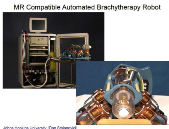
Figure 17: Robot compatible IRM (John Hopkins)
