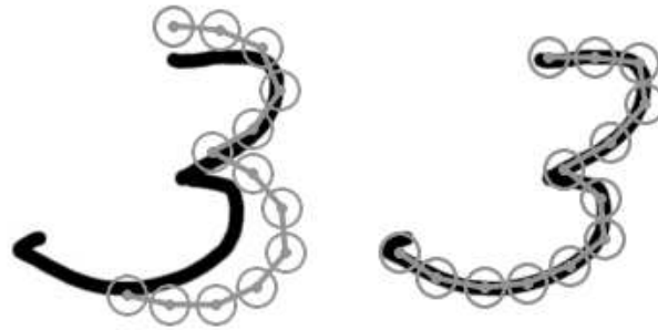
Figure 4.2: Illustration of the idea presented in the work by Hinton et al. [18]. The digit model is represented by a spline on which Gaussian ink-generators are placed. Each pixel of the observed image can be explained by each of these ink-generators. The registration and assignment problems are simultaneously solved for in an EM framework.
