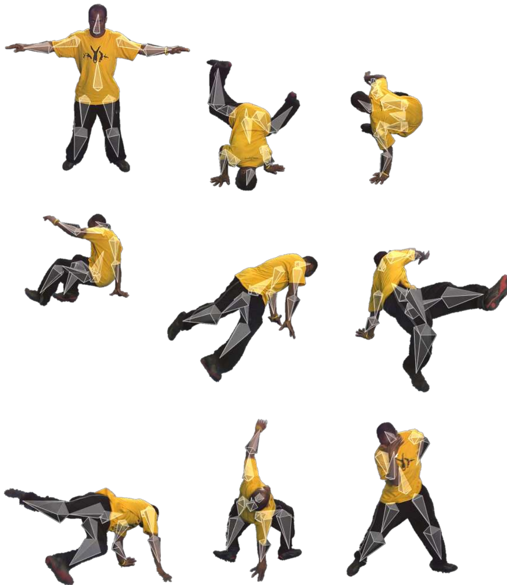
Figure 5.7: Results of the skeleton-based articulated tracking -with probabilistic assignments and patch-prediction- on the Free sequence, overlaid on the original images of camera 2.
