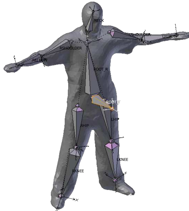
Figure 5.4: Sample kinematic tree with 11 joints to parametrize human motion. The root joint is a translate joint, and all the rotation joints are ball joints, which results in a total of 33 degrees of freedom for the kinematic chain.
