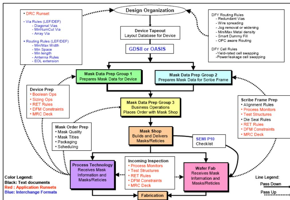
Figure 2.16 Scope of design rules, DFM rules and DFM models [DFM Dictionary, 2004]
