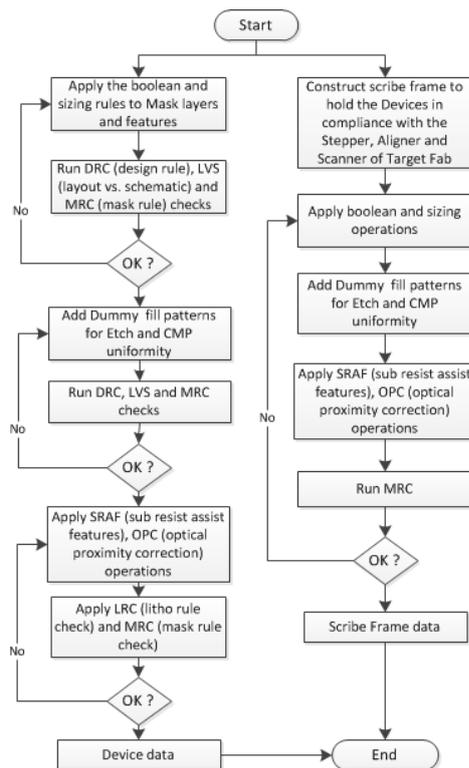
Figure B.6 – Mask data preparation flow
