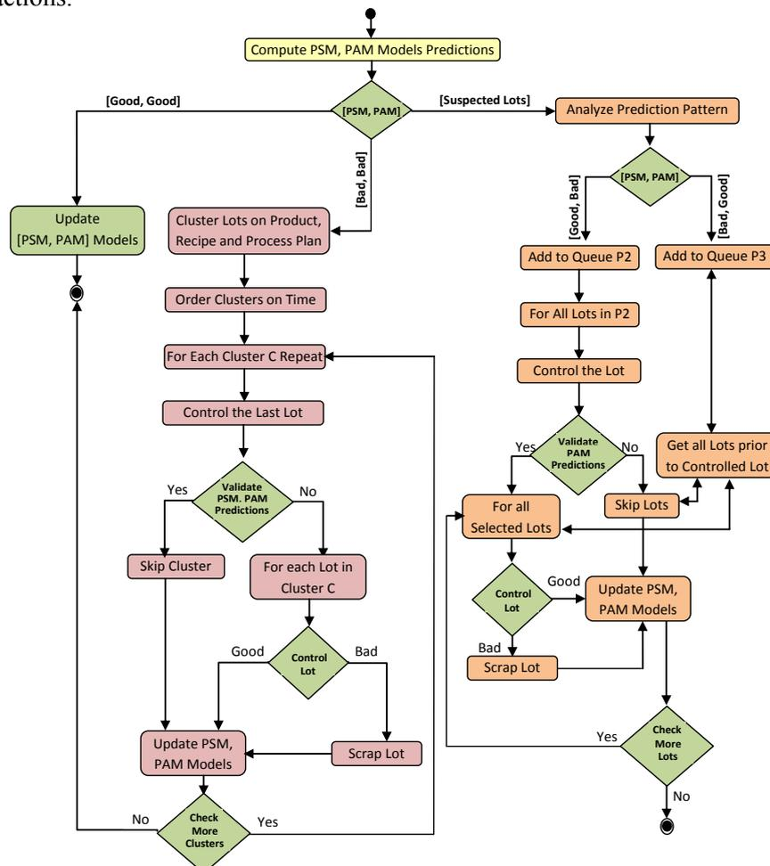
Figure 7.3 - Flow chart for clustering and queue allocations
