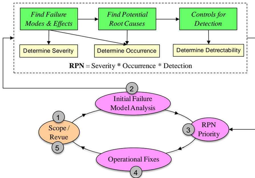
Figure 4.1 – Traditional 5-step FMEA process
