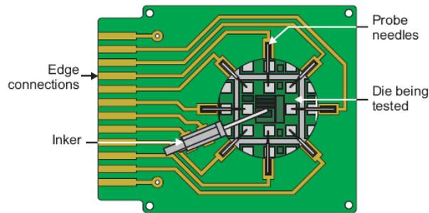
Figure B.16 – Probe interface card and electrical tests
