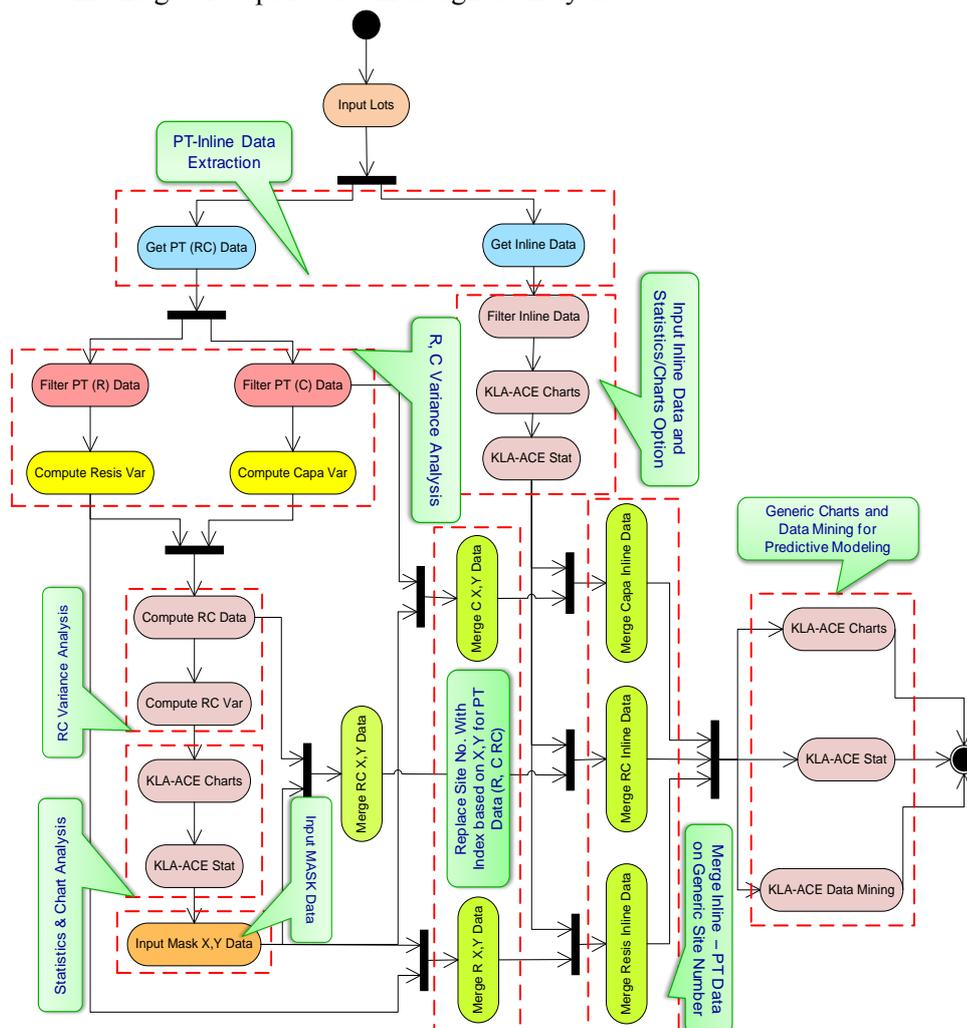
Figure F.1 – PT-Inline Mapping Flow Chart
