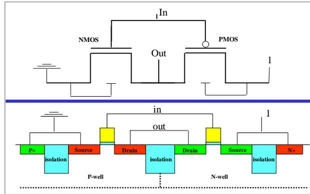
Figure C.2 – CMOS inverter structural presentation
