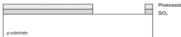
a) Etching of SiO<sub>2</sub> for n-Well diffusion
