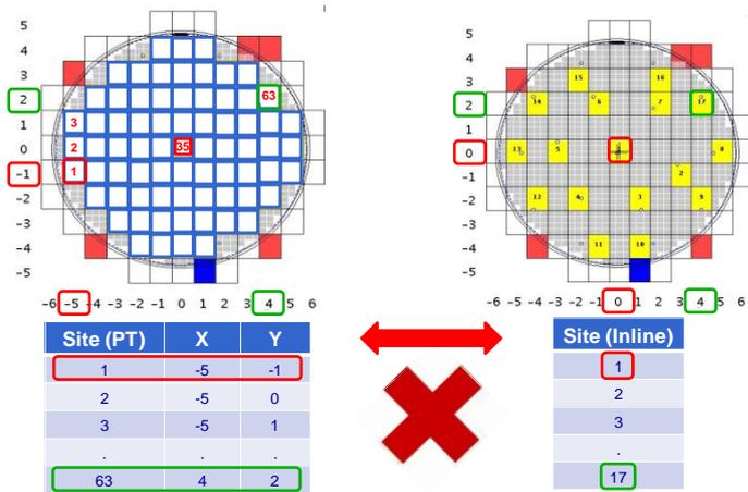
Figure F.2 – Site Level PT-Inline Mapping
