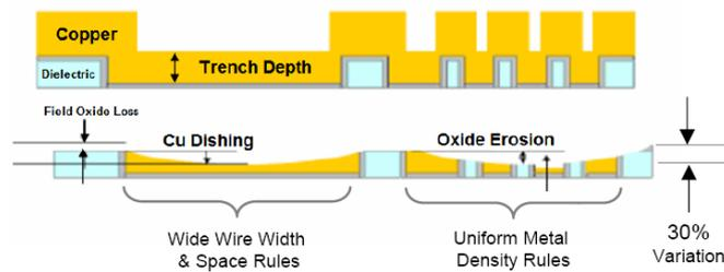
Figure B.24 – Dishing and erosion mechanisms.
