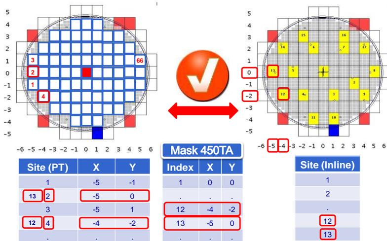
Figure F.3 – Site Level PT-Inline Mapping
