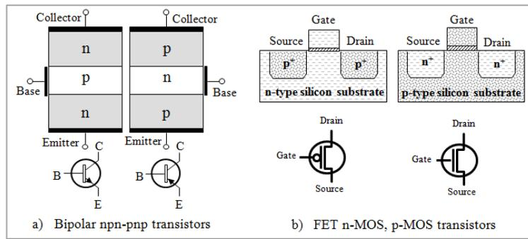
Figure B.1 – Bipolar and FET transistors structure [Quirk and Serda, 2000]
