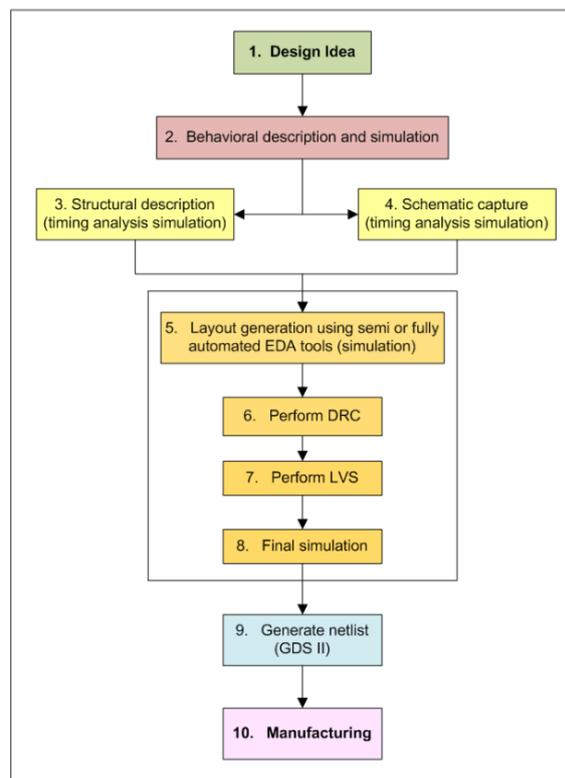
Figure 2.13 - Typical design flow within SI [Reddy, 2000]
