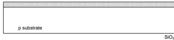
Figure C.12 – Oxidation layer on the raw wafer
