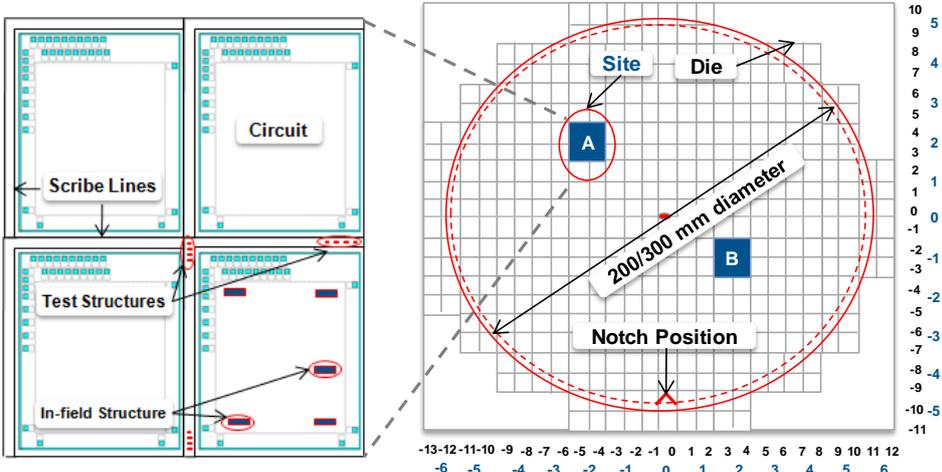
Figure 1.6 - Structure of the product wafer
