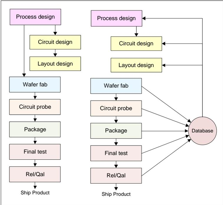
Figure 2.12 - Early semiconductor design flows with loop back [Reid, and Sanders, 2005]
