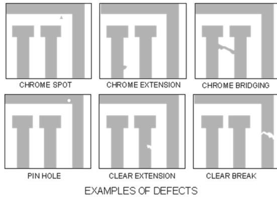
Figure B.8 - mask manufacturing defects
