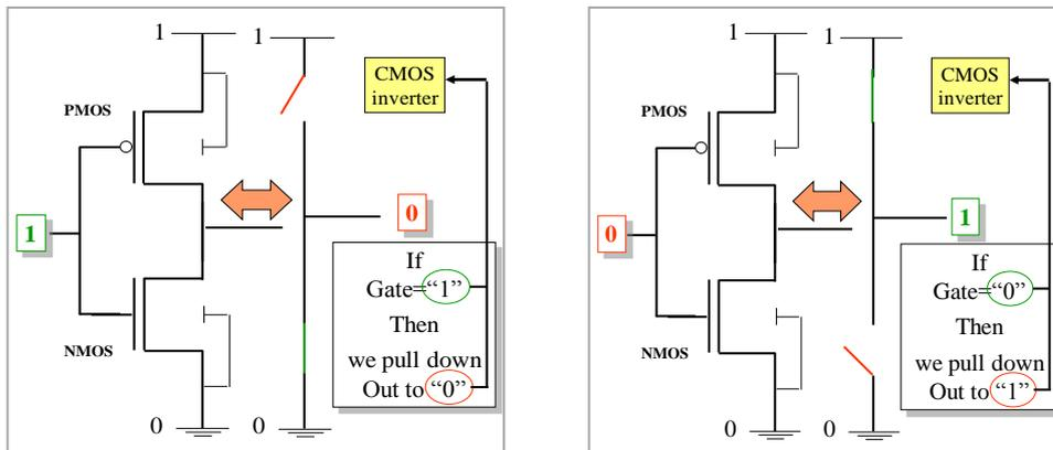
a) CMOS inverter with input 1
