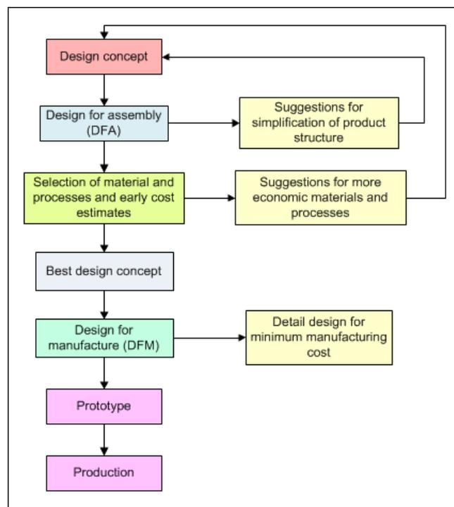
Figure 2.11 - DFMA (design for manufacturability and assembly) [Herrmann et al., 2004]
