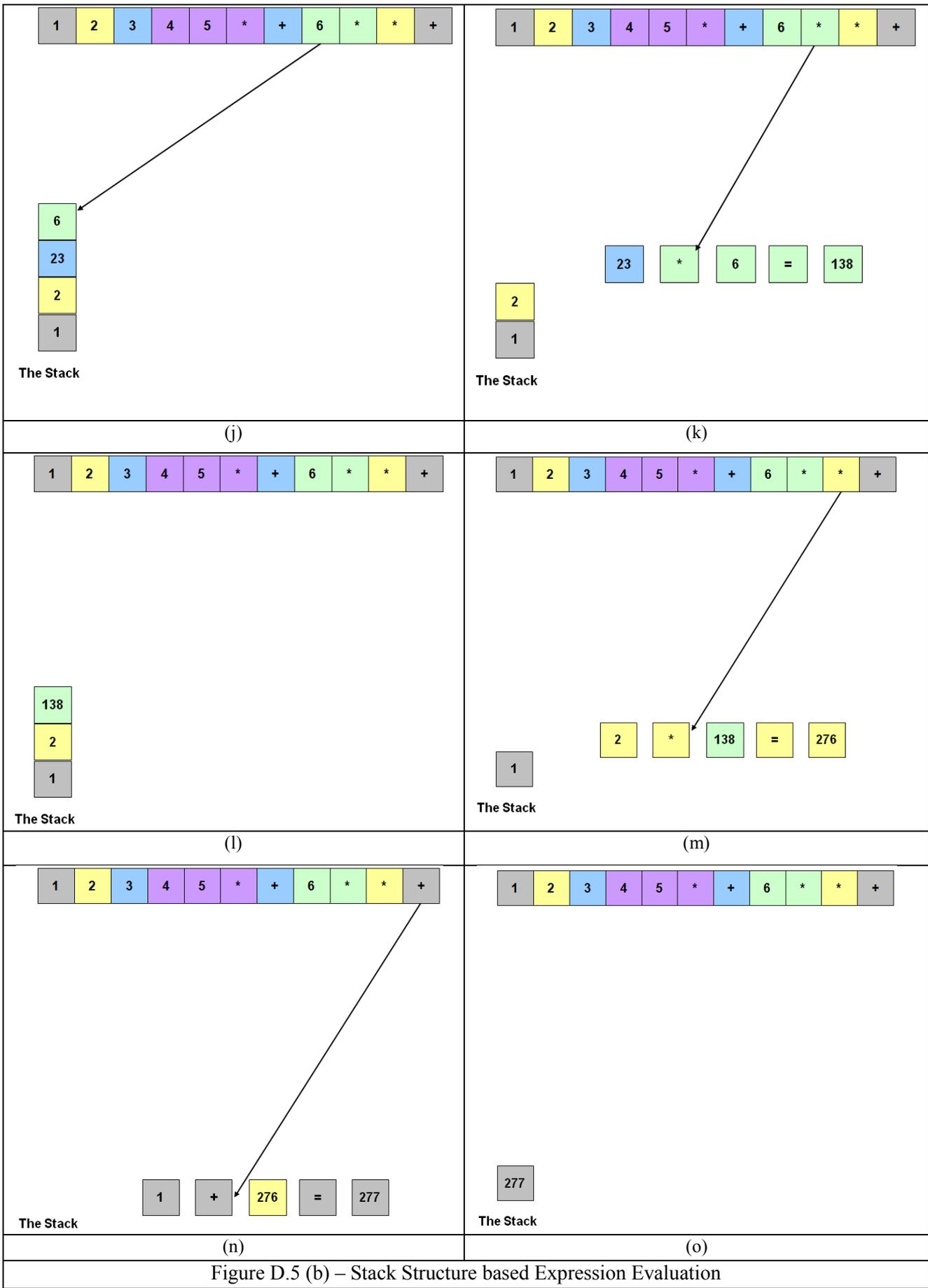
Figure D.5 (b) – Stack Structure based Expression Evaluation
