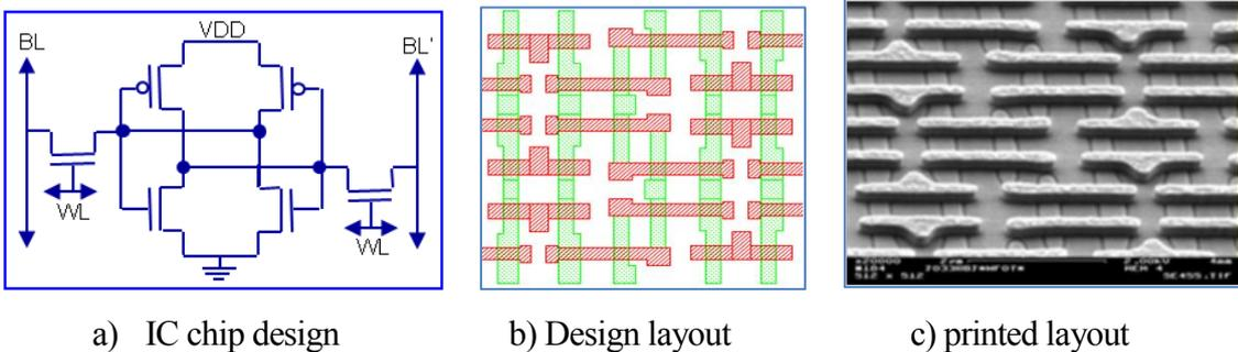
Figure 1.9 – Drifts in drawn features and printed images
