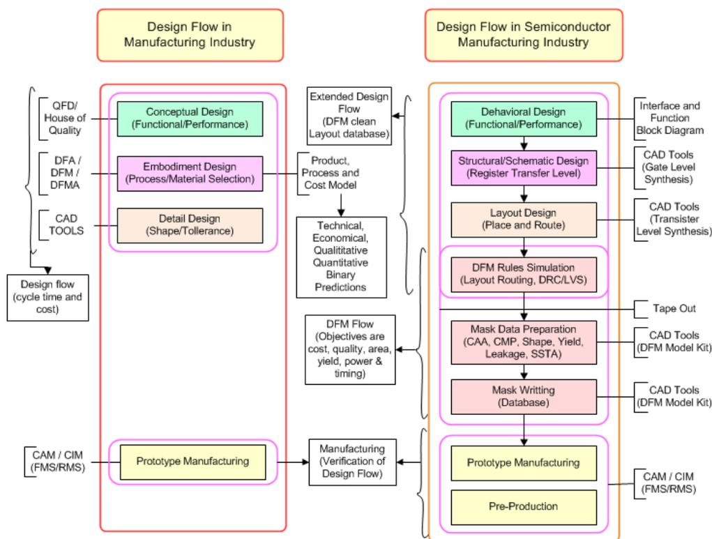
Figure 2.10 - Comparison of the design flows in manufacturing industries and SI
