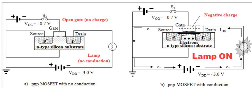
Figure B.13 – pnp MOSFET structure and current flow [Quirk and Serda, 2000]
