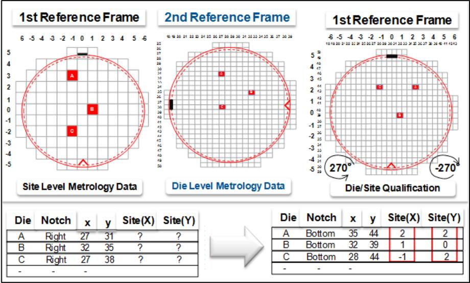
Figure 5.12 – Die/Site level qualifications and varying reference frames
