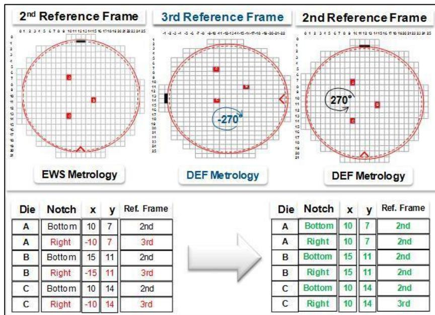
Figure 5.11 – Die/Die levels mismatches due to reference frames
