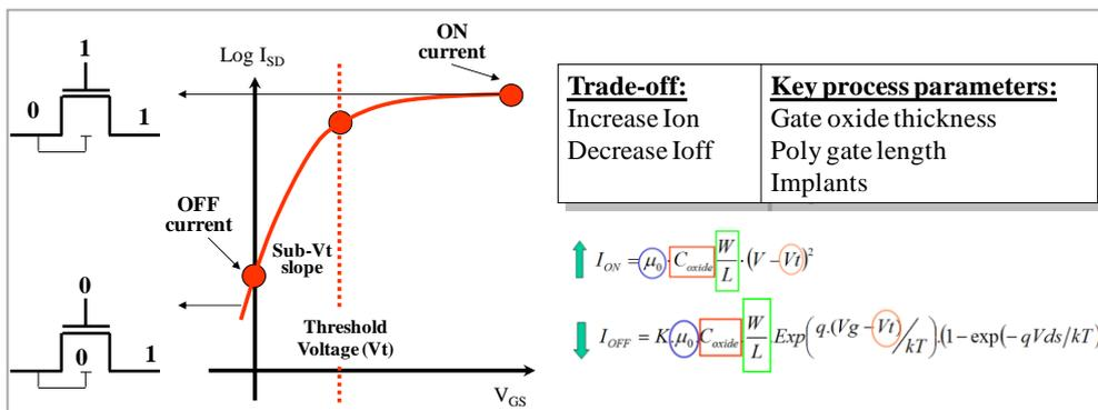
Figure C.3 –  $I_{on}$  and  $I_{off}$  currents and trade off
