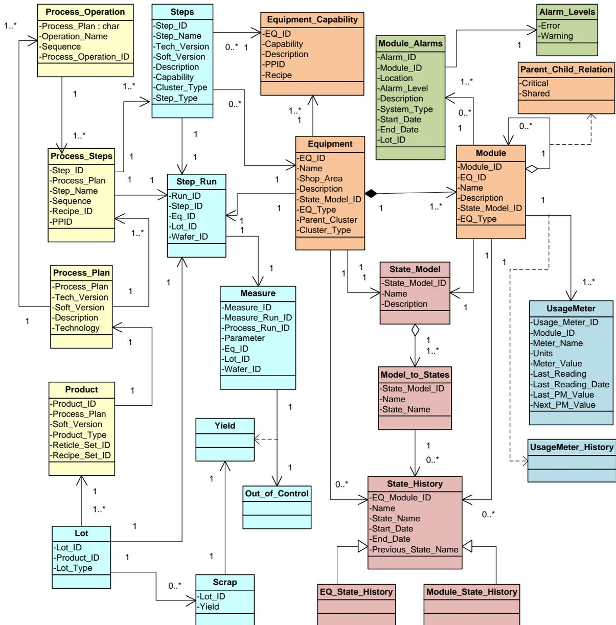
Figure 7.4 - Data model to support [PAM, PSM] models
