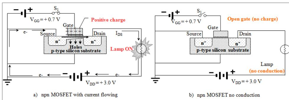
Figure B.12 – npn MOSFET structure and current flow [Quirk and Serda, 2000]
