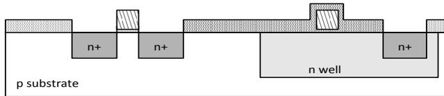
c) n+ diffusion and source, drain and n-well contact
