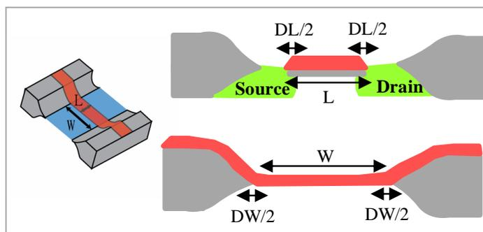
Figure C.8 – Delta in drawn length ( $DL$ ) and width ( $DW$ ) of transistor [Lee, 2005]
