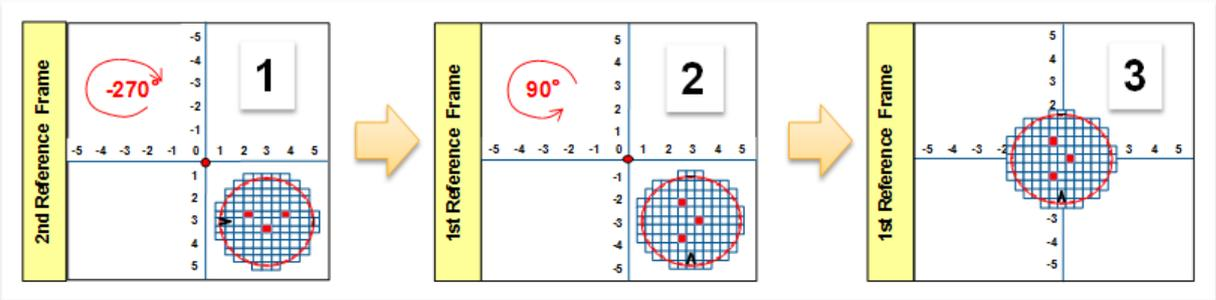
Figure 5.16 – Reference frame and notch position rotation with translation example
