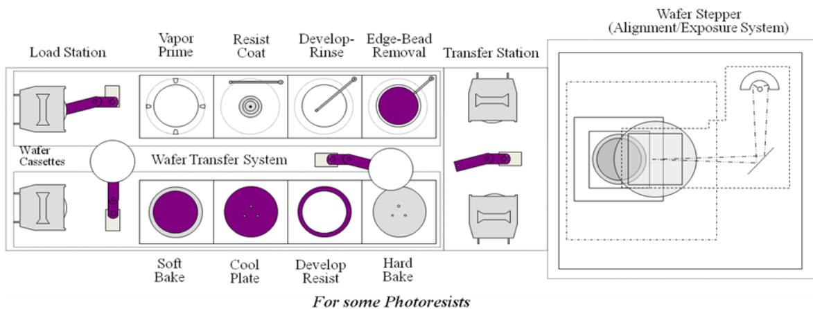
Figure B.19 – Structural description of the lithography equipment
