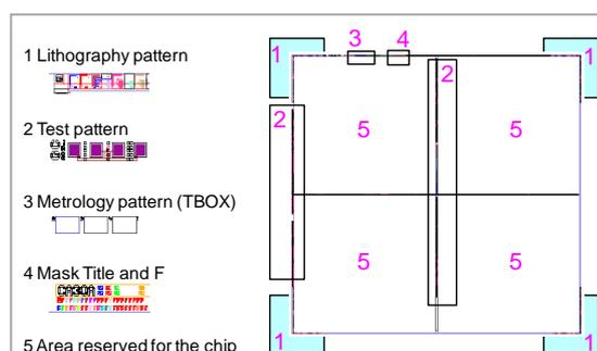
Figure C.9 – Frame structure of a mask
