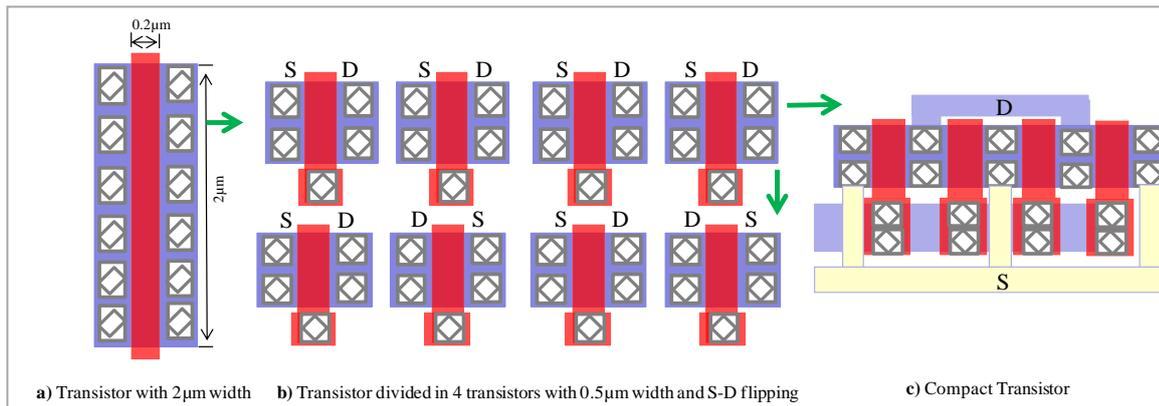
Figure C.7 – Layout optimization of CMOS inverter [Lee, 2005]
