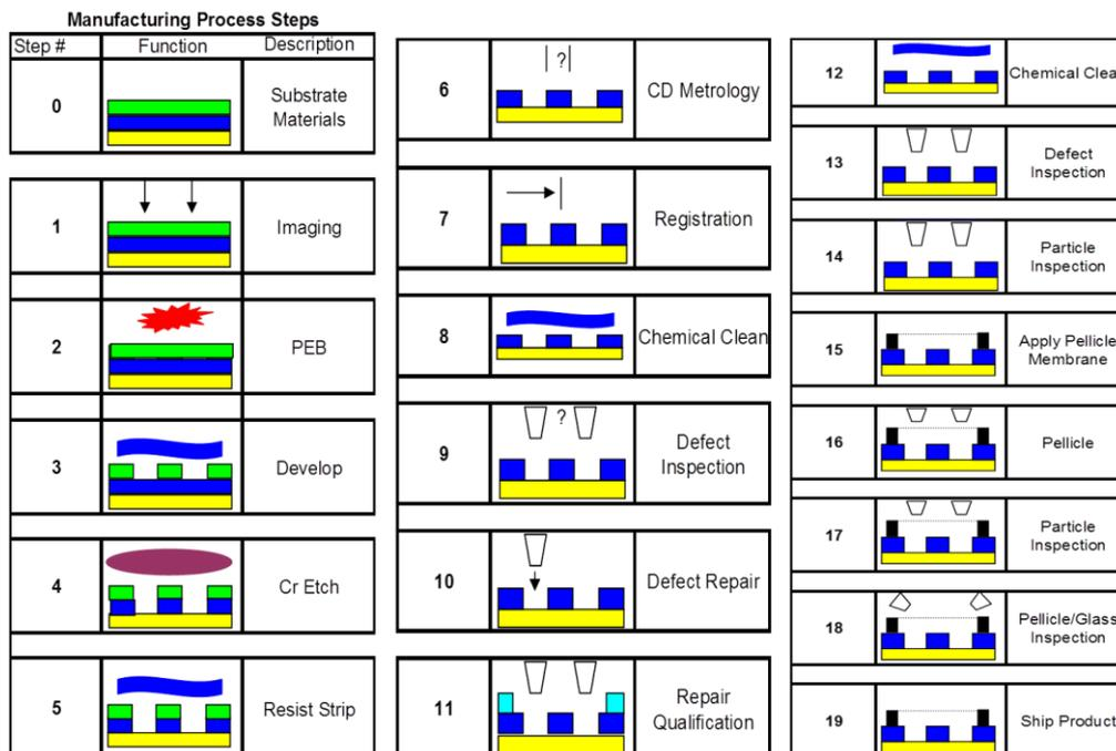
Figure B.7 - back-end mask manufacturing flow
