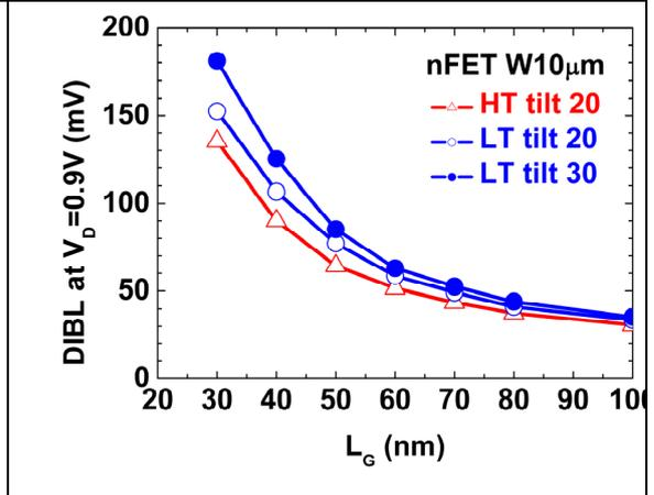
Fig.II.20 DIBL versus  $L_G$  roll-off of LT/HT nFETs with  $W=10\ \mu\text{m}$ . With the same LDD tilt of 20 °, similar DIBL- $L_G$  are observed for LT/HT nFETs. For LT splits, higher LDD implant tilt of 30 ° degrades the DIBL- $L_G$  characteristic, which indicates that higher LDD to gate overlap is obtained.
