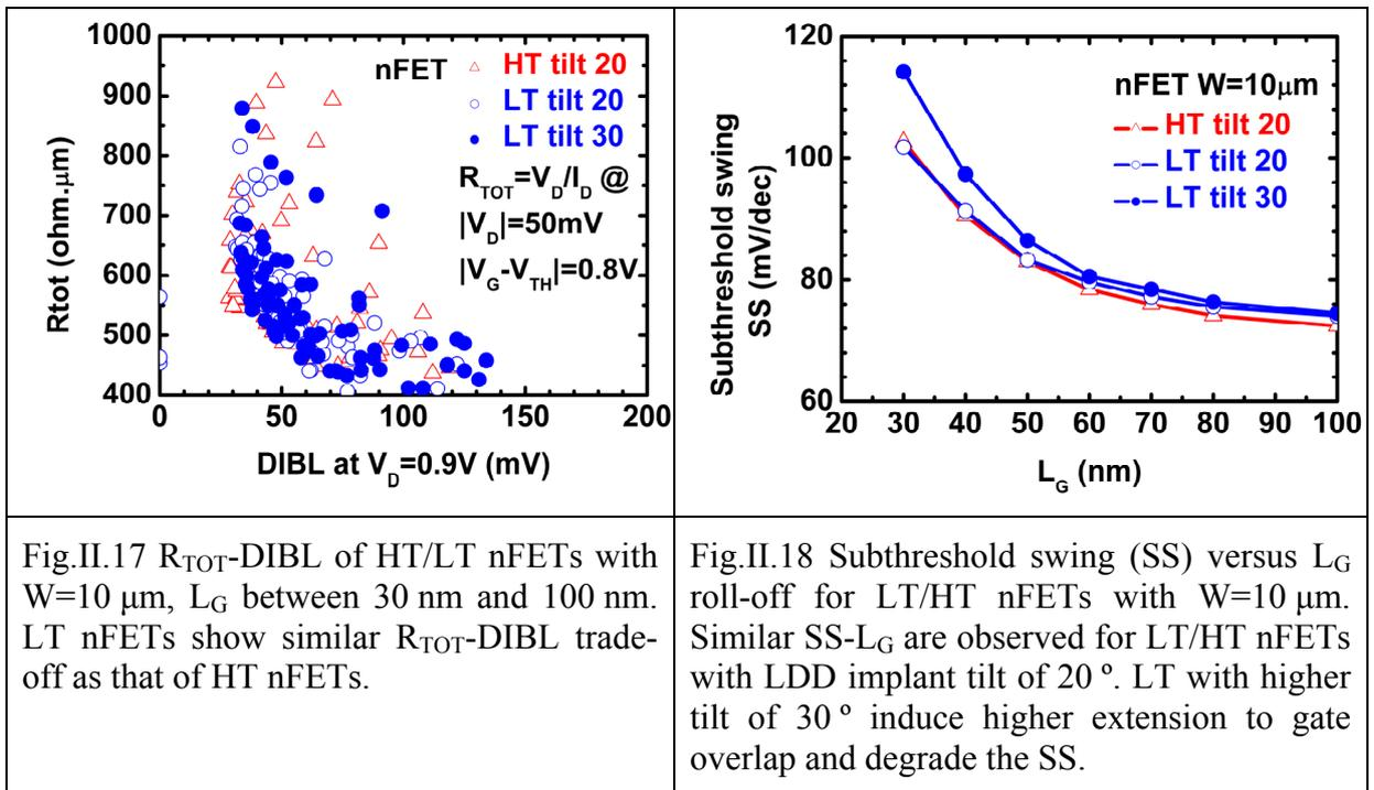
However, the two comparisons above are not sufficient to conclude about which implant tilt ( $20^\circ$  or  $30^\circ$ ) is better optimized for LT nFETs. In order to find the optimized LDD implant tilt, the SCE control of different nFET splits need to be compared and discussed in detail.
