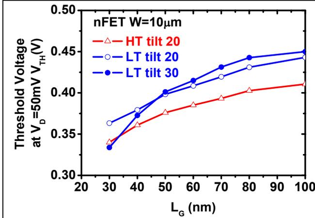
Fig.II.19  $V_{TH}$  versus  $L_G$  roll-off for LT/HT nFETs with  $W=10\ \mu\text{m}$ . Similar  $V_{TH}$ - $L_G$  are observed for LT/HT with tilt 20 °. For LT split with higher tilt of 30 °,  $V_{TH}$  roll-off is degraded due to the higher LDD to gate overlap.
