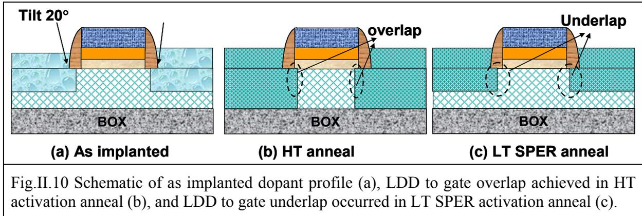
Fig.II.10 Schematic of as implanted dopant profile (a), LDD to gate overlap achieved in HT activation anneal (b), and LDD to gate underlap occurred in LT SPER activation anneal (c).
