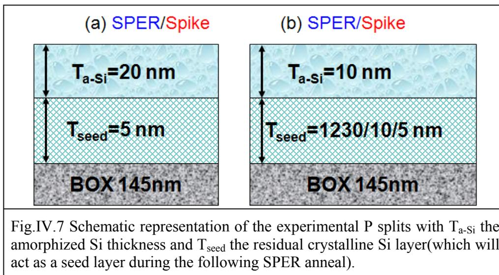
SOI wafers with a BOX of 145 nm and different Si thickness ( $T_{si}$ ) are used in the experiment. Different pre-amorphization implantations are used to achieve different amorphous Si thickness ( $T_{a-si}$ ) and seed thickness ( $T_{seed}$ ). The splits are schematically summarized in Fig.IV.7. For LT SPER activated splits, the EOR defects are located just below the a-c interface, so the distance from the top of EOR band to the BOX ( $T_{EOR\_BOX}$ ) can be approximated taken as  $T_{seed}$ .
