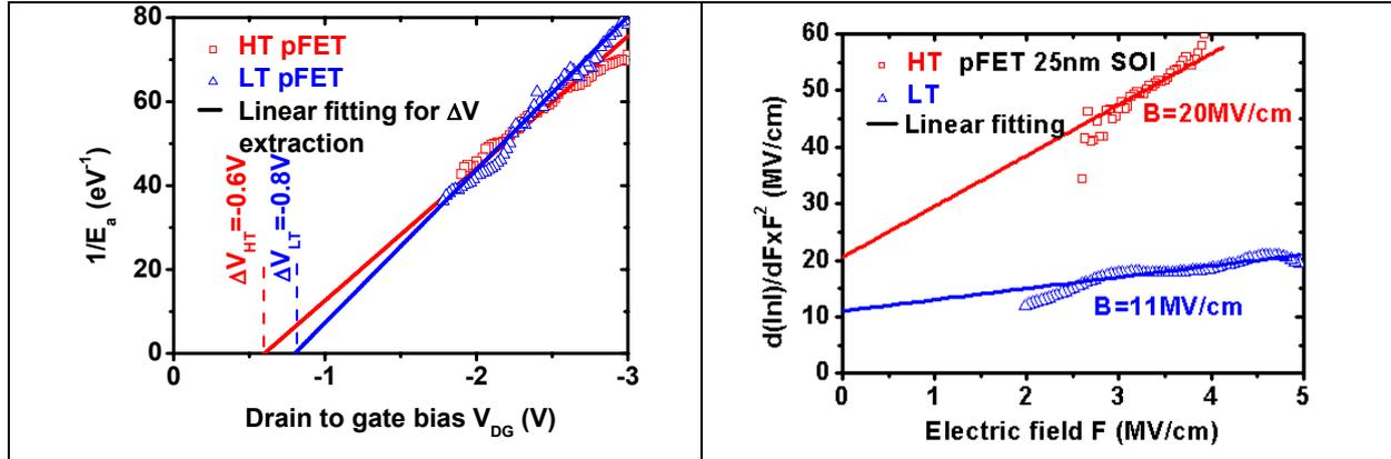
Fig.III.17. Extraction of  $\Delta V$  using the inverse of  $E_A$  versus drain-to-gate voltage ( $V_{DG}$ ) plot (pFETs with 25 nm Si channel).
