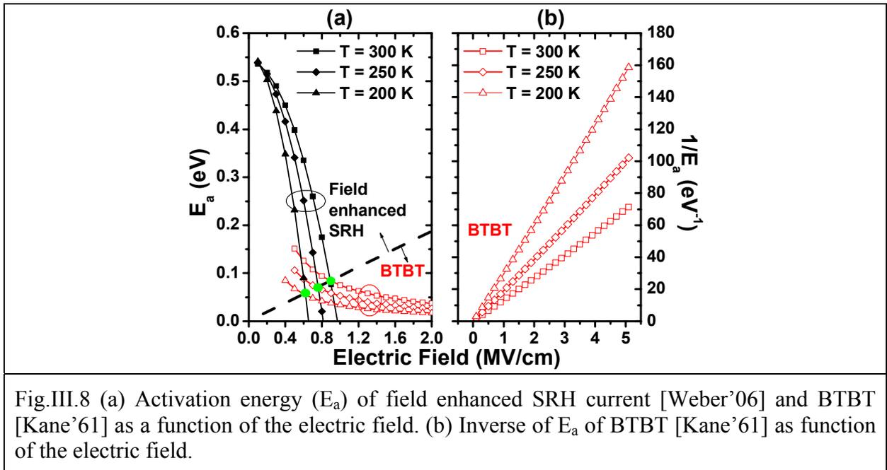
Fig.III.8 (a) Activation energy ( $E_a$ ) of field enhanced SRH current [Weber'06] and BTBT [Kane'61] as a function of the electric field. (b) Inverse of  $E_a$  of BTBT [Kane'61] as function of the electric field.
