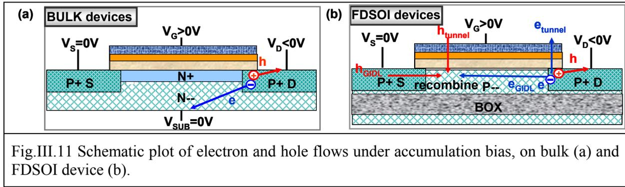
Fig.III.11 Schematic plot of electron and hole flows under accumulation bias, on bulk (a) and FDSOI device (b).
