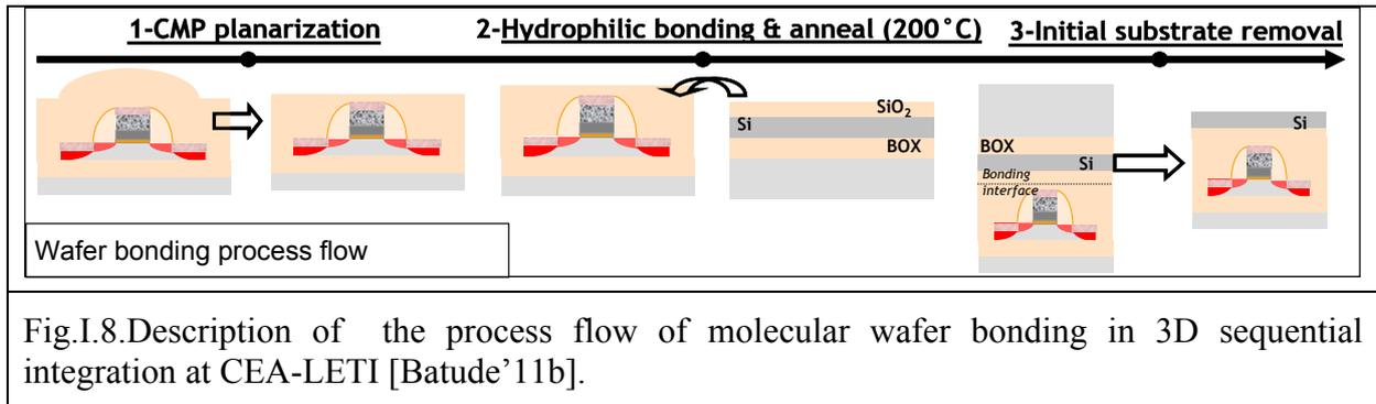
Fig.I.8. Description of the process flow of molecular wafer bonding in 3D sequential integration at CEA-LETI [Batude'11b].
