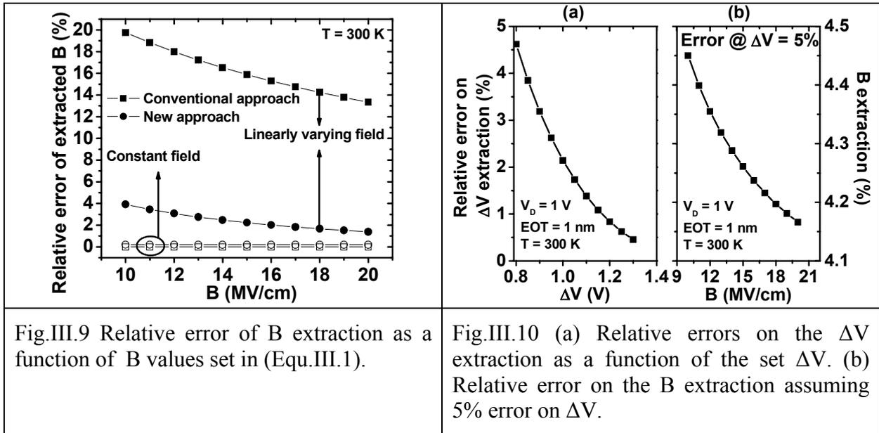
The small extraction error obtained with the new method tends to confirm that (Eq.III.2) can be approximated by (Eq.III.3) provided that the maximum field of the profile is used (e.g. instead of a mean field). In other terms, weak fields do not significantly contribute to the GIDL current compared to the maximum one, because of the steep exponential GIDL dependence with field.
