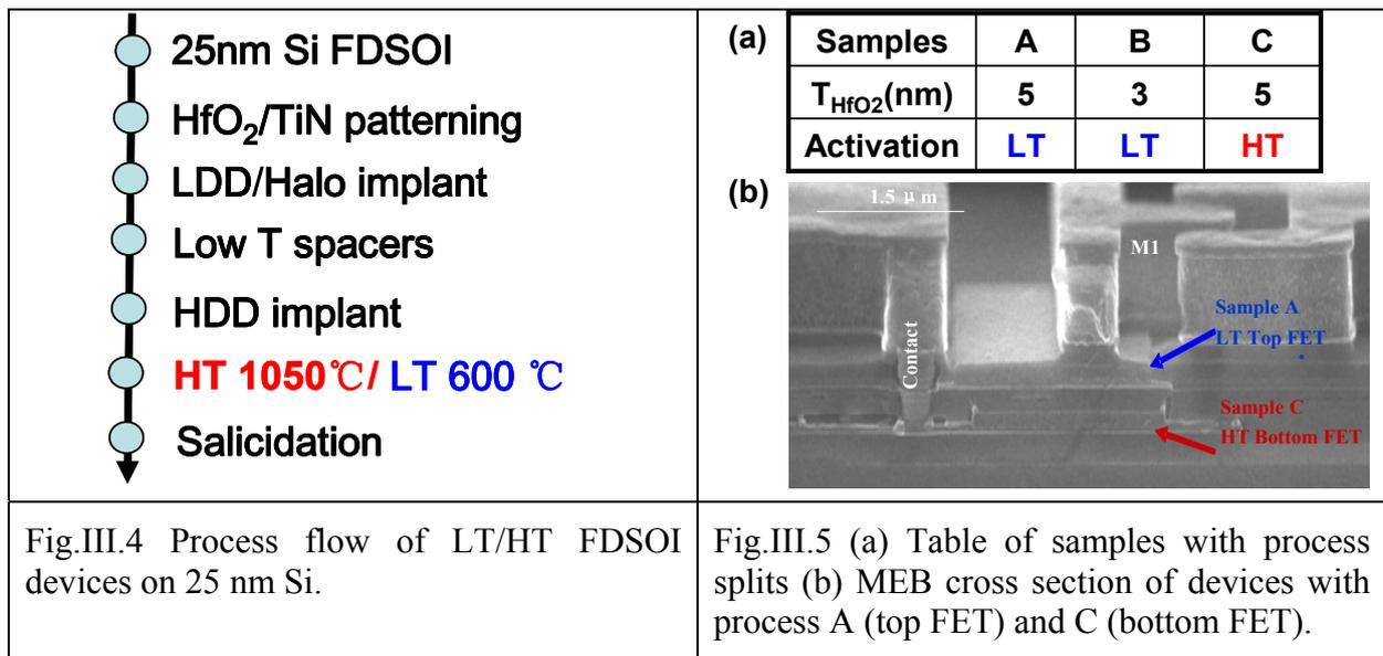
As discussed in Chapter II, the drain junction of LT SPER activated device has two properties: (1) highly doped abrupt junction; (2) EOR defects left below the junction. As a result, LT SPER can increase GIDL [Xu'10]. On one hand, the highly doped and abrupt junction results in high electric field and high BTBT leakage consequently. On the other hand, the residual EOR defects can increase the GIDL leakage by enhancing TAT and SRH recombination.
