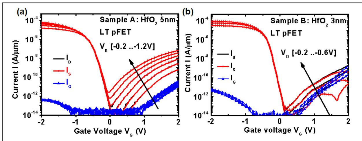
Fig.III.12 Absolute drain ( $I_D$ ), source ( $I_S$ ) and gate ( $I_G$ ) current for pFETs from process A with 5 nm  $HfO_2$  (a) and B with 3 nm  $HfO_2$  (b). The source is grounded and the drain is biased at -0.2 V to -1.2 V, with a step of -0.2 V.
