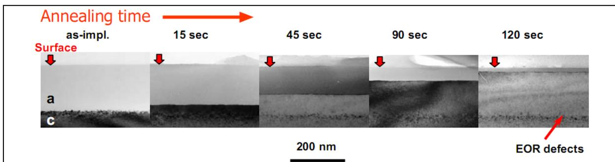
Fig.II.5 XTEM micrographs of SPER isothermally annealed at 600 °C [Colombeau'04a]. After LT SPET anneal, EOR defects are left below the a/c interface.
