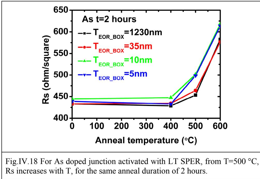
We can conclude that LT SPER activated arsenic are not stable during post anneal at  $500\text{-}600\text{ }^{\circ}\text{C}$ . In contrast with boron, on ETSOI samples, deactivation of LT SPER activated arsenic is enhanced. However, as shown in Section.IV.3.2, we still managed to achieve similar sheet resistance in LT SPER samples and standard HT process, which allows us to use LT SPER in 3D sequential integration for FDSOI nFETs on both the top and bottom layers in 3D sequential integration.
