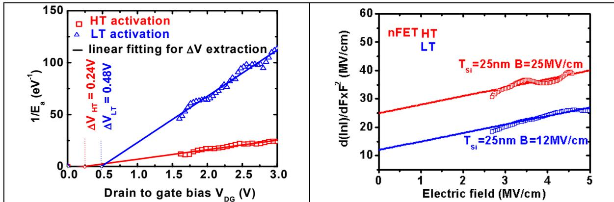
Fig.III.19. Extraction of  $\Delta V$  using the inverse of  $E_A$  versus drain-to-gate voltage ( $V_{DG}$ ) plot (nFETs with 25 nm Si channel).
