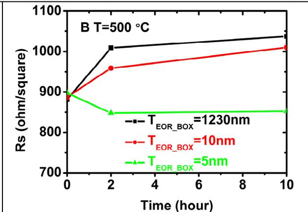
Fig.IV.10 Sheet resistance evolution of boron doped junction as a function of anneal time at 500 °C. During the initial phase of anneal,  $R_s$  increases for  $T_{EOR\_BOX} = 1230\text{ nm}$  and  $10\text{ nm}$ , whereas it decreases for  $T_{EOR\_BOX} = 5\text{ nm}$ .
