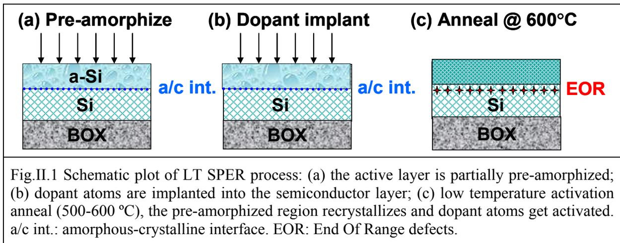
(a) *Pre-Amorphization*- During ion implantation into single crystalline Si, the implanted ions tend to lose energy initially through elastic collisions with electrons of Si atoms
