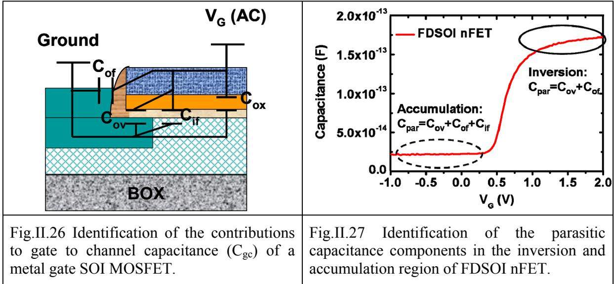
$C_{ox}$ : gate capacitance, due to gate dielectric.  $C_{ox}$  depends on the thickness of gate dielectric and its dielectric constant. Also, quantum effect can decrease the gate capacitance slightly.
