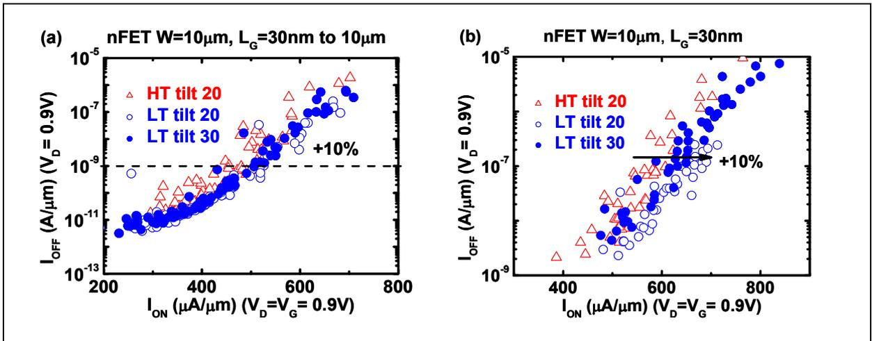
Fig.II.16  $I_{OFF}$ - $I_{ON}$  trade-off of HT/LT nFETs with  $W=10$   $\mu$ m,  $L_G$  between 30 nm and 10  $\mu$ m in (a). For  $W=10$   $\mu$ m,  $L_G=30$  nm, the  $I_{OFF}$ - $I_{ON}$  trade-off is highlighted in (b). At a constant  $I_{OFF}$  of  $10^{-9}$  A/ $\mu$ m,  $I_{ON}$  of LT nFETs are  $\sim 10\%$  higher than that of HT nFETs.
