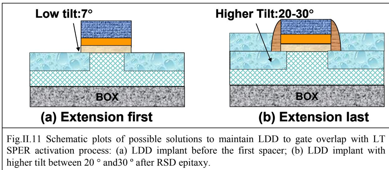
Fig.II.11 Schematic plots of possible solutions to maintain LDD to gate overlap with LT SPER activation process: (a) LDD implant before the first spacer; (b) LDD implant with higher tilt between  $20^\circ$  and  $30^\circ$  after RSD epitaxy.
