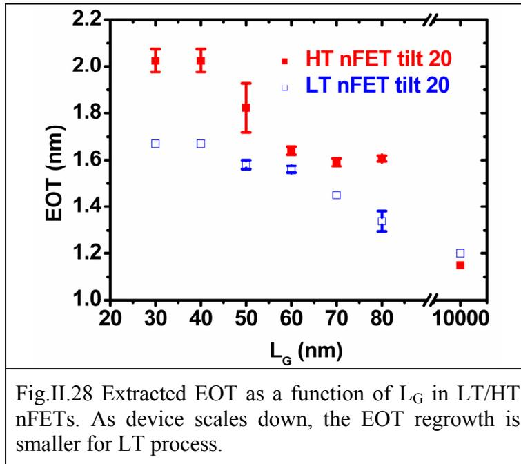
It is obvious that for both LT and HT devices, there is an increase of EOT as devices scale down, which is consistent with the assumption that the SiO<sub>2</sub> regrows mainly in the boundary of the gate to channel interface. However, the EOT increment of LT split is lower than that of HT split. This phenomenon is consistent with the better control of interfacial SiO<sub>2</sub> regrowth in LT process [Batude'09c, Ragnarsson'06].
