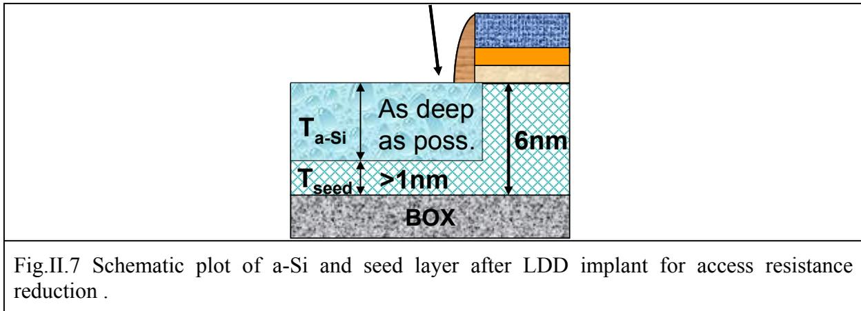
Fig.II.7 Schematic plot of a-Si and seed layer after LDD implant for access resistance reduction .
