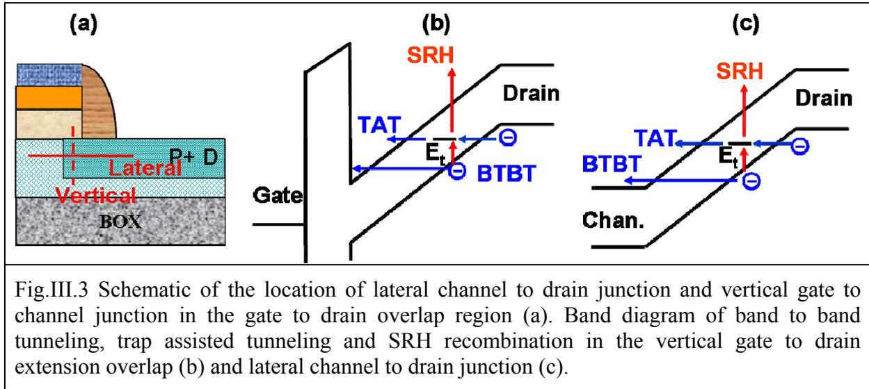
Fig.III.3 Schematic of the location of lateral channel to drain junction and vertical gate to channel junction in the gate to drain overlap region (a). Band diagram of band to band tunneling, trap assisted tunneling and SRH recombination in the vertical gate to drain extension overlap (b) and lateral channel to drain junction (c).
