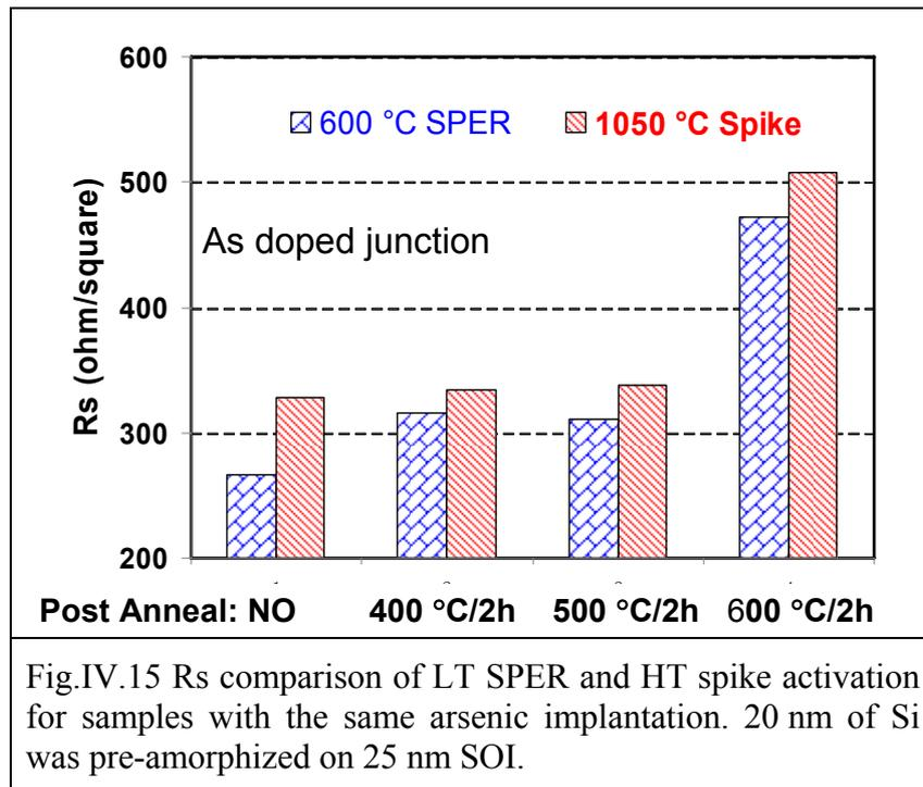
In Fig.IV.15, the sheet resistance values of LT SPER and spike activated samples are compared, before and after different post activation anneals. It is found that the sheet resistance of LT SPER and HT spike samples are similar, both just after the activation (no post anneal) and after post activation anneals. Since this implant condition is close to the LDD implant in standard FDSOI nFETs, and we can conclude that LT SPER can provide similar or
