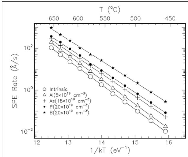
Fig.II.3 Arrhenius plot showing the temperature dependence of the SPER rate for intrinsic and uniformly doped a-Si layers. The incorporation of aluminum (Al), arsenic (As), phousphorous (P) and boron (B) increases the regrowth speed [Johnson’07].
