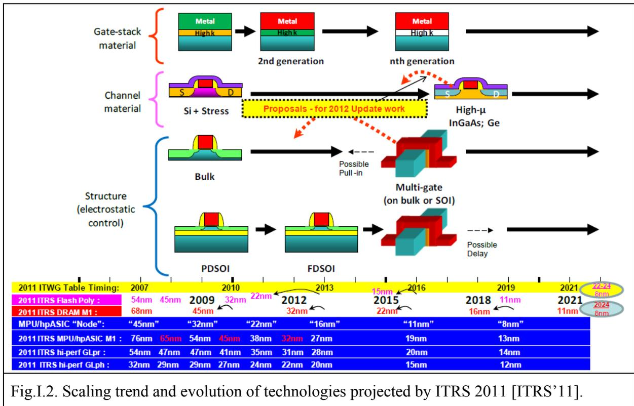
Fig.I.2. Scaling trend and evolution of technologies projected by ITRS 2011 [ITRS'11].
