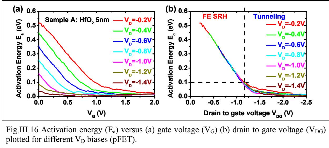
Fig.III.16 Activation energy ( $E_a$ ) versus (a) gate voltage ( $V_G$ ) (b) drain to gate voltage ( $V_{DG}$ ) plotted for different  $V_D$  biases (pFET).
