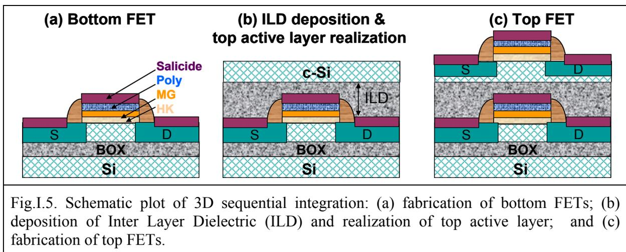
Depending on how the top crystalline active layer is achieved, there are mainly two approaches of 3D sequential integration: the concept will be briefly introduced in the following sub-sections. In [Batude'09a], detailed review of the history of 3D sequential integration is made. In 3D sequential integration, the alignment between top and bottom layers is limited by lithography. Alignment around 10 nm can be achieved, which is much better than that of 3D parallel integration [Batude'11b].
