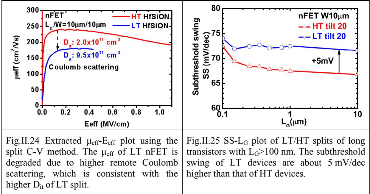
In LT process, the lack of HT activation anneal degrade the gate to channel interface quality, mobility and SS performances as a consequence. For our future study, to further improve the gate to channel interface quality, forming gas anneal (FGA) should be optimized. Indeed, higher pressure FGA with pure  $\text{H}_2/\text{D}_2$  anneal has been reported to be effective to reduce  $D_{\text{it}}$  [Diouf'12, Park'05].
