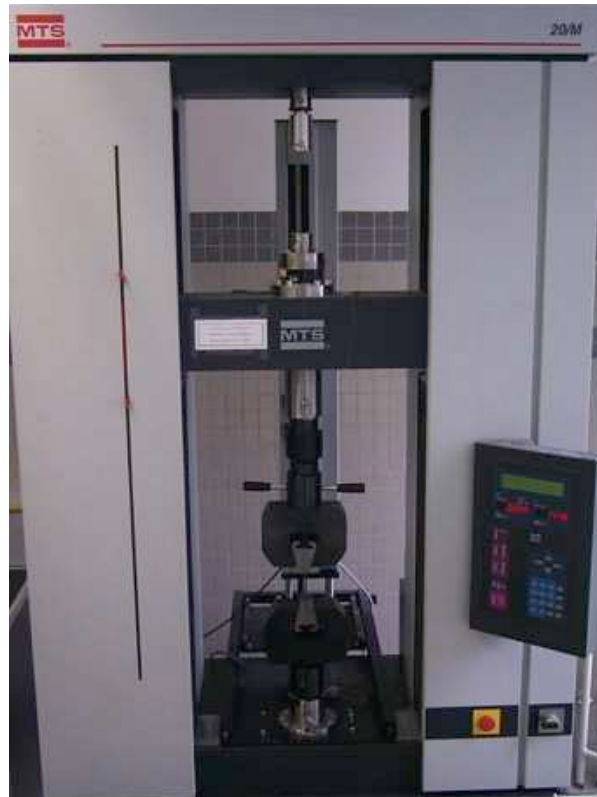
Figure 4.9: DMA machine used for the compression tests on the polyurethane foams.
