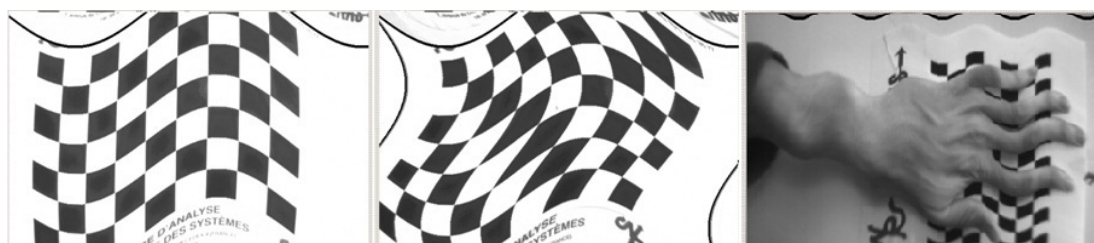
Figure 5.4: Sinusoidal transformation - The input image is transformed using a table encoding a sinusoidal transformation. This way, we tested the correct operation of the module.
