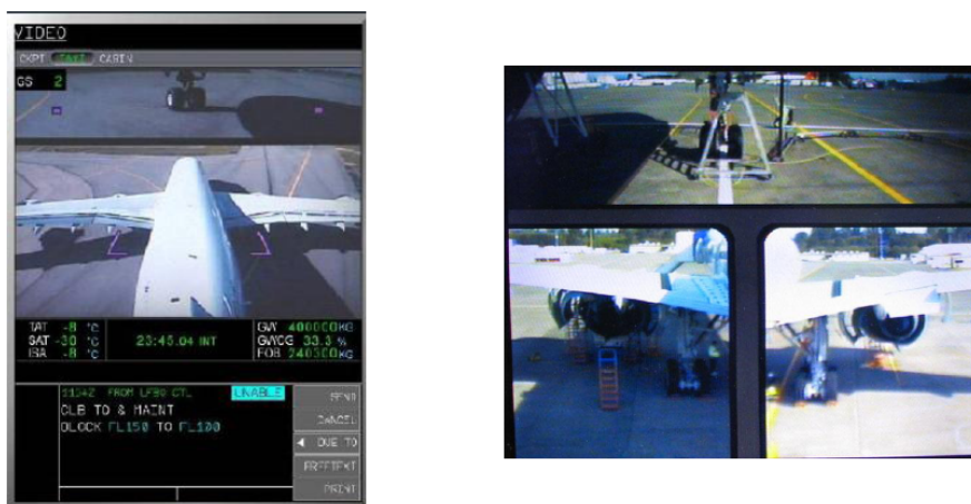
Figure 1.2: Camera navigation systems - On the left, ETACS display appearance (taken from [8]). On the right, GMCS display appearance (taken from [7])
