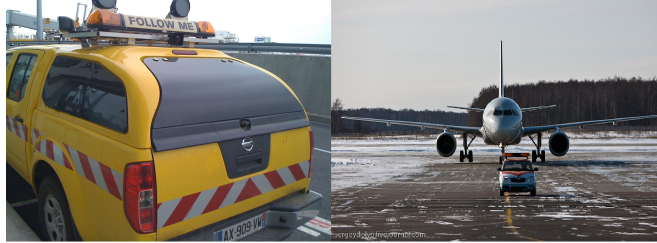
Figure 1.1: Follow me vehicle - Safety procedure used in many airports to guide the aircrafts. Taken from [4]
