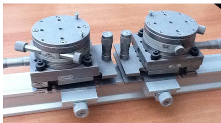
Figure 2.12: Configurable mechanic base for stereo vision -
