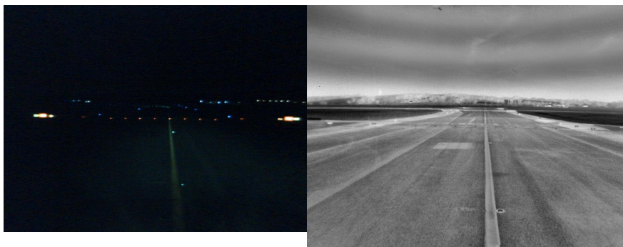
Figure 2.10: Infrared and visible image of the stop bar in an airport context. - Infrared image was equalized using CLAHE
