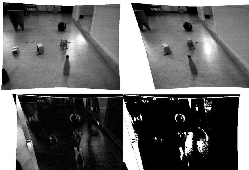
Figure 5.17: SIPM results - Top-left: Left image undistorted. Top-right: Right Image undistorted. Bottom-left: Homography of right image undistorted. Bottom right: I_{right} - H[I_{left}]
