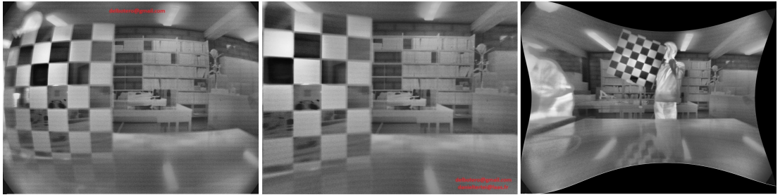
Figure 5.36: Infrared Image SART Camera - On the left, the original distorted image. On the right, the image after distortion correction. In all images contrast was enhanced using CLAHE
