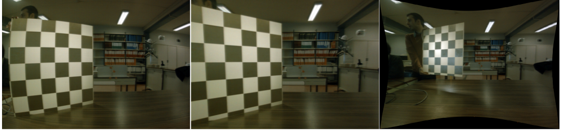
Figure 5.35: Visible Image SART Camera - On the left, the original distorted image. On the right, the image after distortion correction
