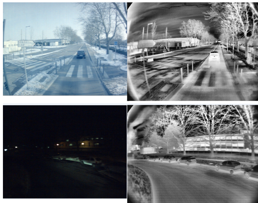
Figure 2.8: Infrared and visible view of a day and night scene - Infrared image was equalized using CLAHE
