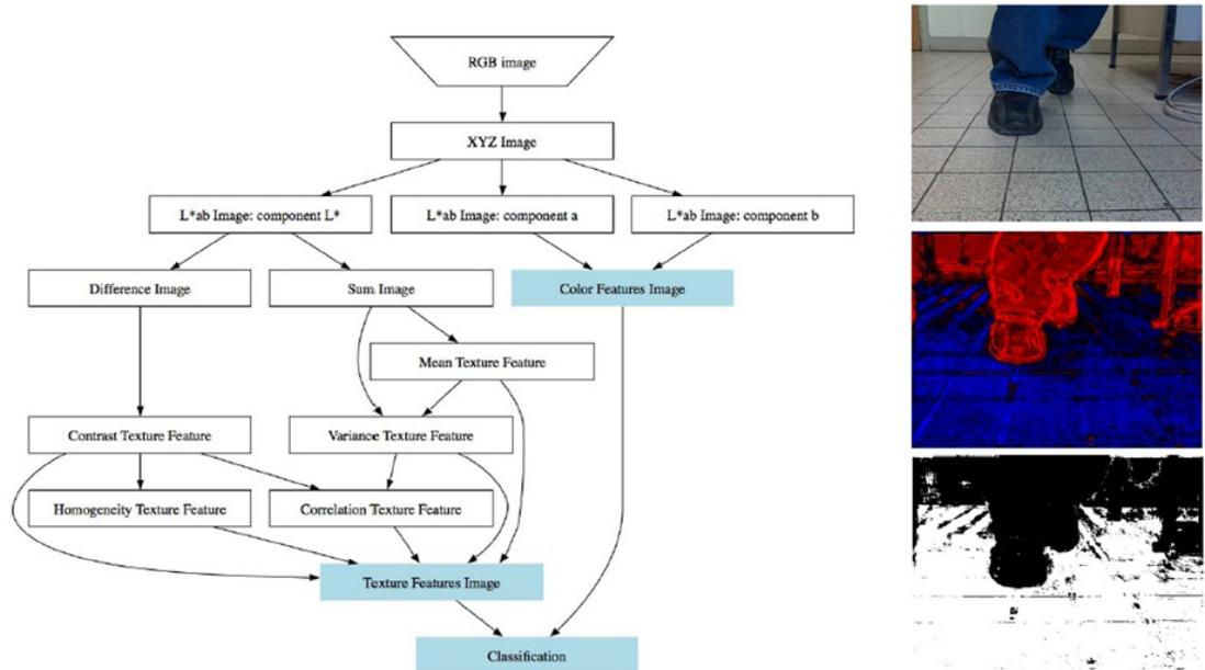
Figure 2.13: Texture object detection algorithm - Taken from [11]
