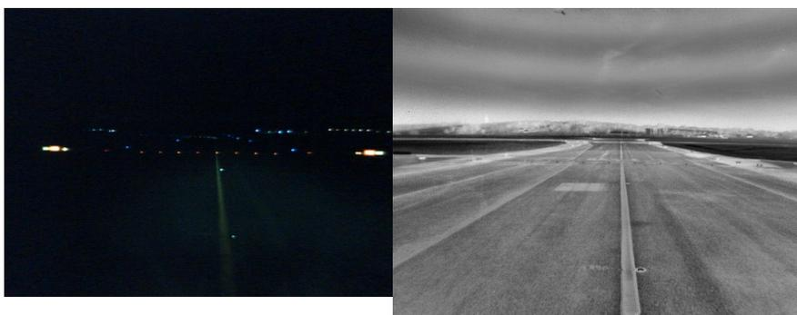
**Figure 2.10: Infrared and visible image of the stop bar in an airport context.** - Infrared image was equalized using CLAHE
