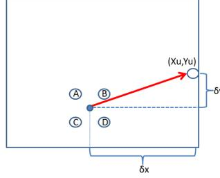
**Figure 4.1: Distortion correction pixel interpolation** - Pixel in coordinates  $X_u, Y_u$  is computed using the interpolation of four vicinity pixels (A, B, C and D) indexed using the information encoded in  $\delta_x$  and  $\delta_y$ .
