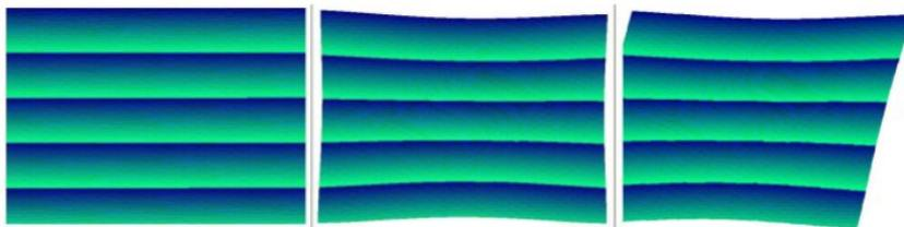
**Figure 5.16: SIPM tables encode homography and distortion correction simultaneously.** - On the left, the input table which represents a null transformation. In the middle, the table which encodes correction distortion. On the right, the table which encodes distortion correction and homography simultaneously.
