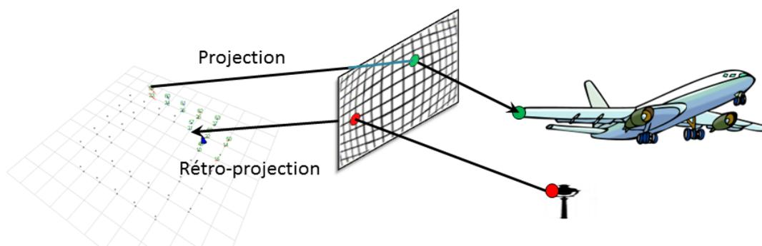
**Figure 2.17:** Calibration necessity for SLAM projection, illustrates the projection, retro-projection operations done during the SLAM algorithm. -
