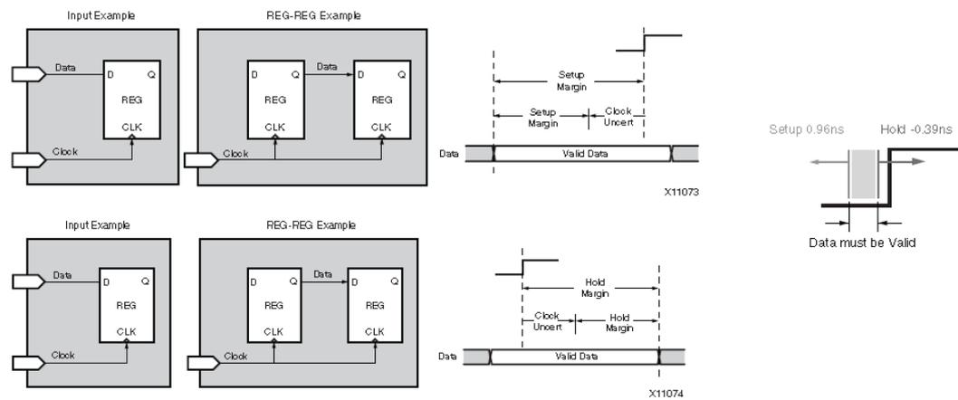
Figure 3.9: Setup and Hold - Taken from [64]
