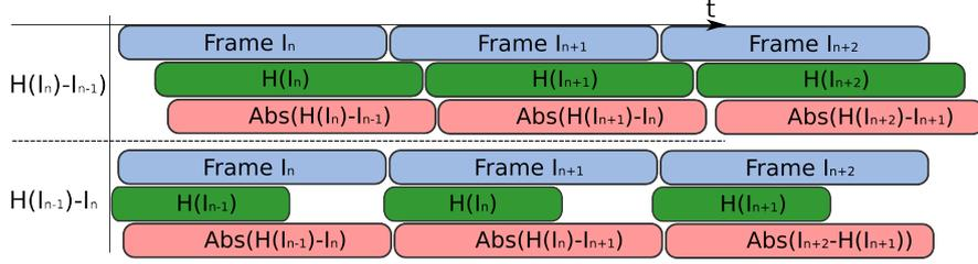
**Figure 4.20: Gantt chart to compare latency of both MIPM methods** -  $H[I_{n-1}]$  can be built at the start of frame of  $I_n$ . To build  $H[I_n]$  some lines of  $I_n$  must be already in memory, which implies an extra latency
