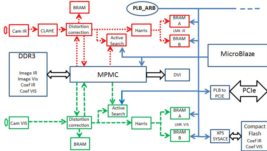
**Figure 4.29: SLAM accelerator block diagram** - The red dotted line represents the data flow of the infrared images, the green dotted line represents the data flow of the visible images and the blue one represents the PLB Bus
