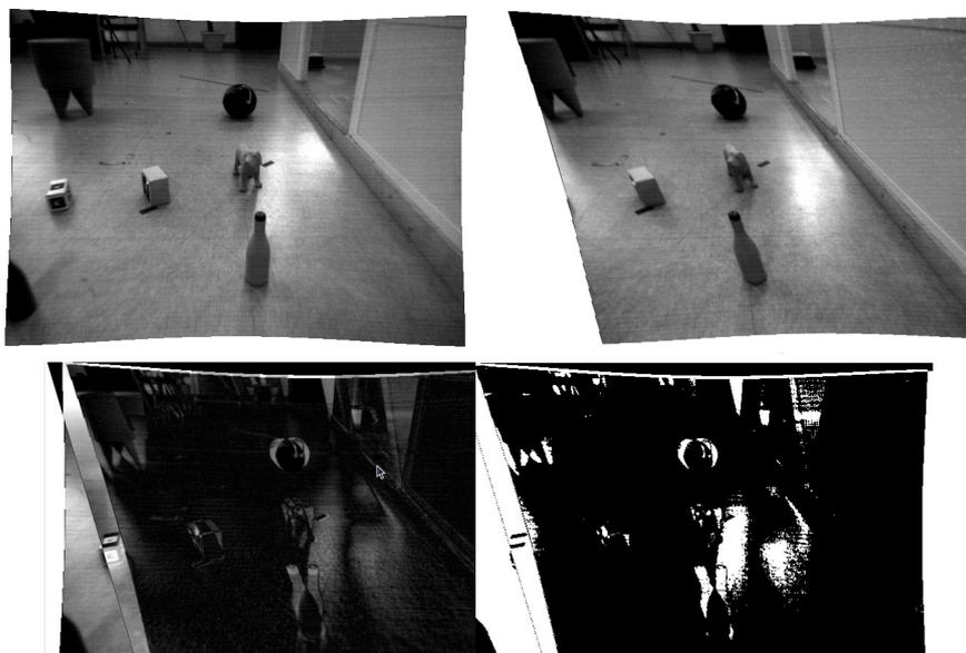
**Figure 5.18: Shadow effects in SIPM** - Top-left: Left image undistorted. Top-right: Homography of right image undistorted. Bottom-left:  $\text{Abs}(I_{right} - H[I_{left}])$ . Bottom right: Output SIPM, threshold of  $\text{Abs}(I_{right} - H[I_{left}])$
