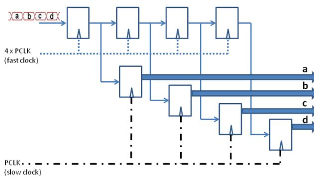
**Figure 4.7: Serial to parallel Distortion Correction module** - Vicinity pixels are read at 4xpclock, then they are processed in parallel at the pclk frequency.
