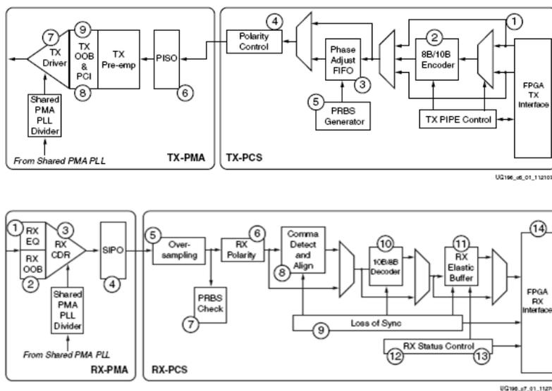
Figure 3.6: GTP block diagrams - Taken from [60]
