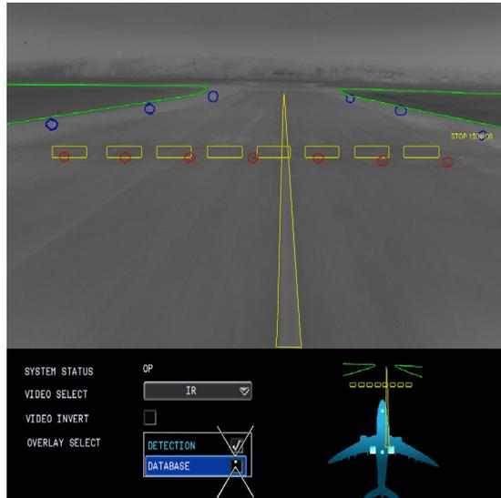
**Figure 5.31: SART HMI displayed image** - Using the estimated position predicted with the SLAM algorithm and the airport database, a synthetic image will be created with the superposition of the acquired-processed image and the database information.
