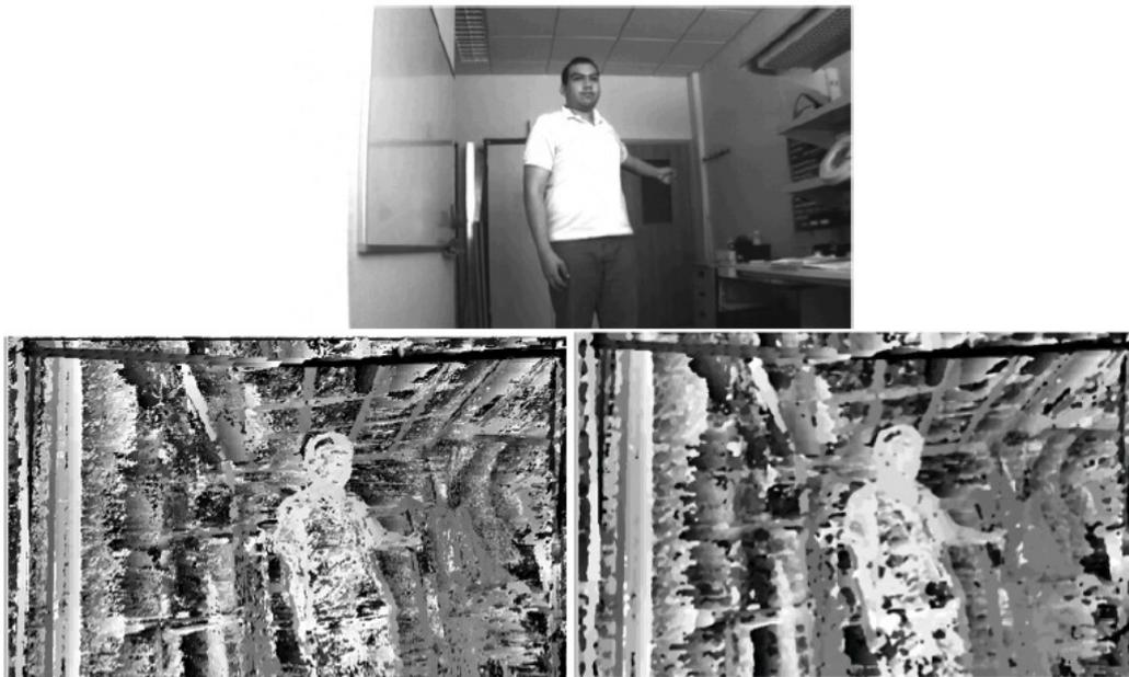
**Figure 5.24: Disparity map after distortion correction** - On the top, the input image. On the bottom-left, the disparity map generated at 100 fps. On the bottom-right, the disparity map after a post-processing to eliminate noise.
