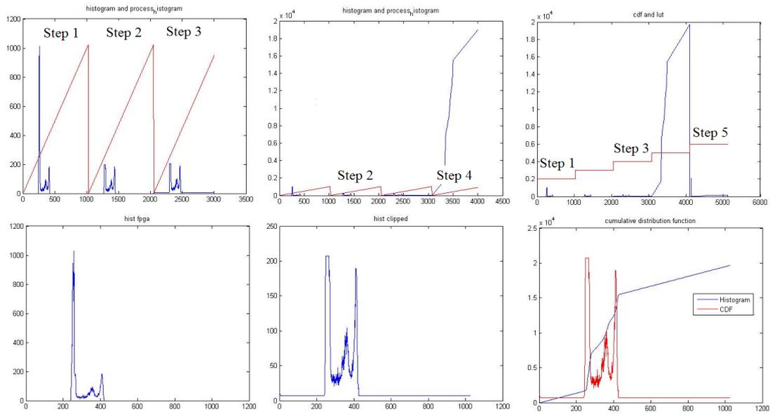
**Figure 5.6: CLAHE System generator simulation** - On the top, the images illustrates the five steps done to compute the LUT. On the bottom, the left image shows the original histogram, the middle image shows the clipped histogram, and the right image shows the histogram and the CDF.
