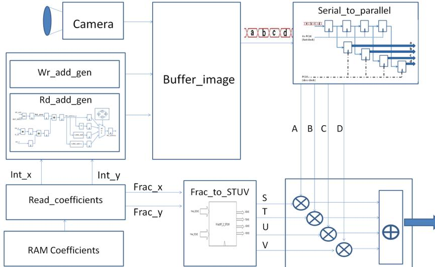
**Figure 4.3: Distortion Correction architecture** - This module uses two memories, one is used to store some lines of the image stream (buffer image) and the other one is used to read the coefficients (RAM COEF).
