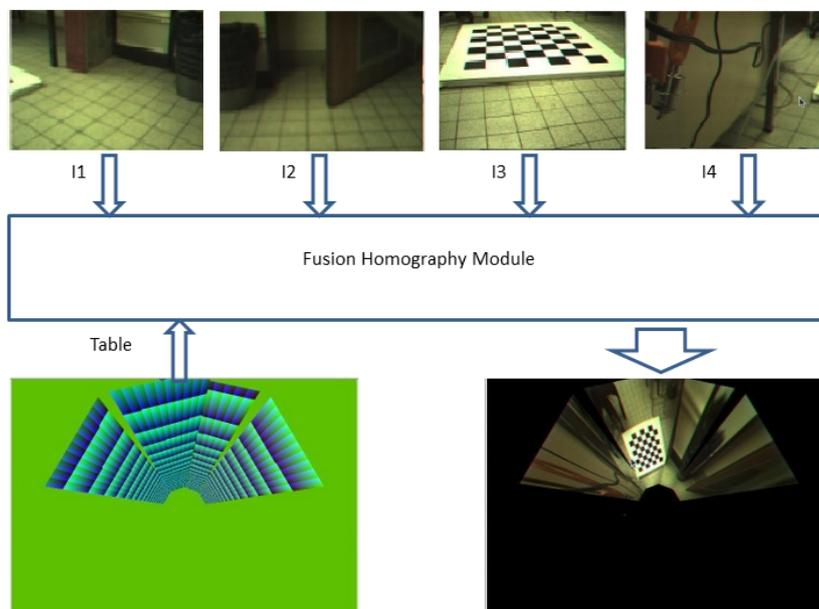
**Figure 5.20: COMMROB Multicamera fusion image** - Information from four cameras are acquired and a fusion image is built using a table. The module Fusion Homography module generates the Bird's eye view at 30 fps.
