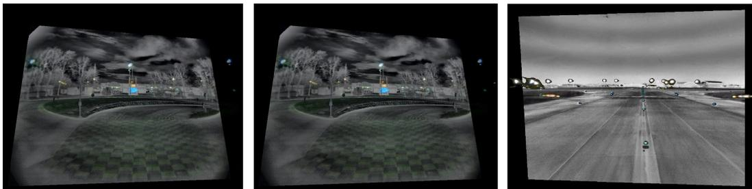
**Figure 5.13: Fusion IR and VIS in different color spaces** - On the left, Fusion using RGB color space. In the middle, Fusion using HSV color space. On the right, Fusion using YCbCr color space
