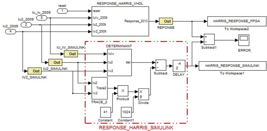
**Figure 5.25: Harris module in system generator and the Simulink model** - On the top, a black box containing the VHDL module of the Harris Arithmetic unit. On the bottom, the Simulink model; the Simulink model includes delay blocks to take into account the latency generated by the pipeline of the VHDL model. Both models are stimulated with the same input. Then, the output responses from the two models are compared to verify the correct operation of the module.
