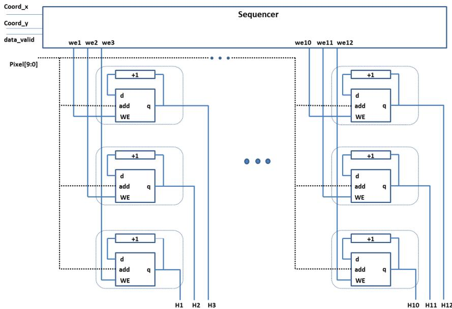
**Figure 4.9: CLAHE histogram array architecture** - When a new pixel arrives, just one of the histogram sub-modules is enabled, and the corresponding bin count will be incremented according to the pixel value. The histogram sub-module is enabled according to the coordinate of the arriving pixel.
