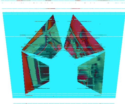
**Figure 5.12: Homography necessity of pipelining.** - This image corresponds to the occupancy grid generated in the COMMROB project, here we implemented all the arithmetic operations corresponding to the homography in one clock cycle (without pipeline). Because of the setup and hold violations due to the long paths, the output image is noisy.
