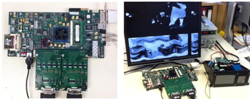
**Figure 5.45: Hardware Platform used to develop SLAM Accelerator** - On the left, the ML605 development kit, with the custom FMC boards to connect the cameras. On the right, the platform with the camera and a screen where we visualize the output images.
