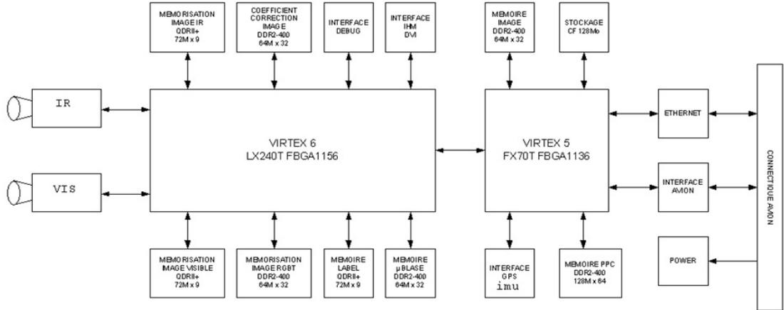
**Figure 5.40: Block diagram SART System** - The system is based on two FPGAs connected through the Gigabit transceivers.
