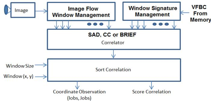
**Figure 4.43: Block diagram of the Active Search module.** - The output of this module are the coordinates ( $I_{obs}, J_{obs}$ ) and the score of correlation
