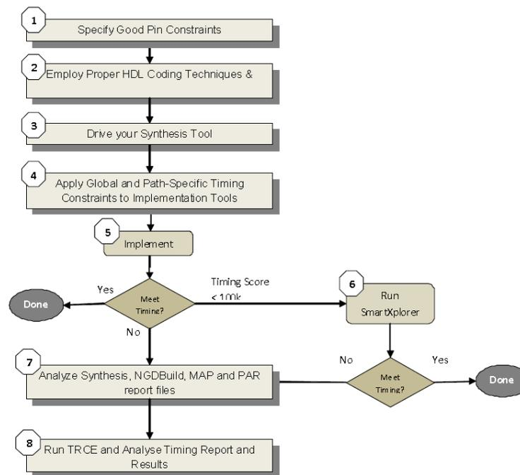
Figure 7-1: Timing Closure Flowchart
