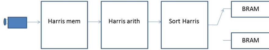
**Figure 4.38: Harris detection block diagram** - The system is composed of three main blocks: memory unit, arithmetic unit and Sort unit. The Sort Unit detect the best computed score in each subimage. Result is written in a pair of BRAM's used like ping pong buffers.
