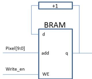
**Figure 4.8: Histogram tile block diagram** - Each histogram is computed using a BRAM memory and a counter. The input pixel is used to address the memory and increment the current count stored. Before beginning to implement the histogram, the memory is written with zeros to initialize the count.
