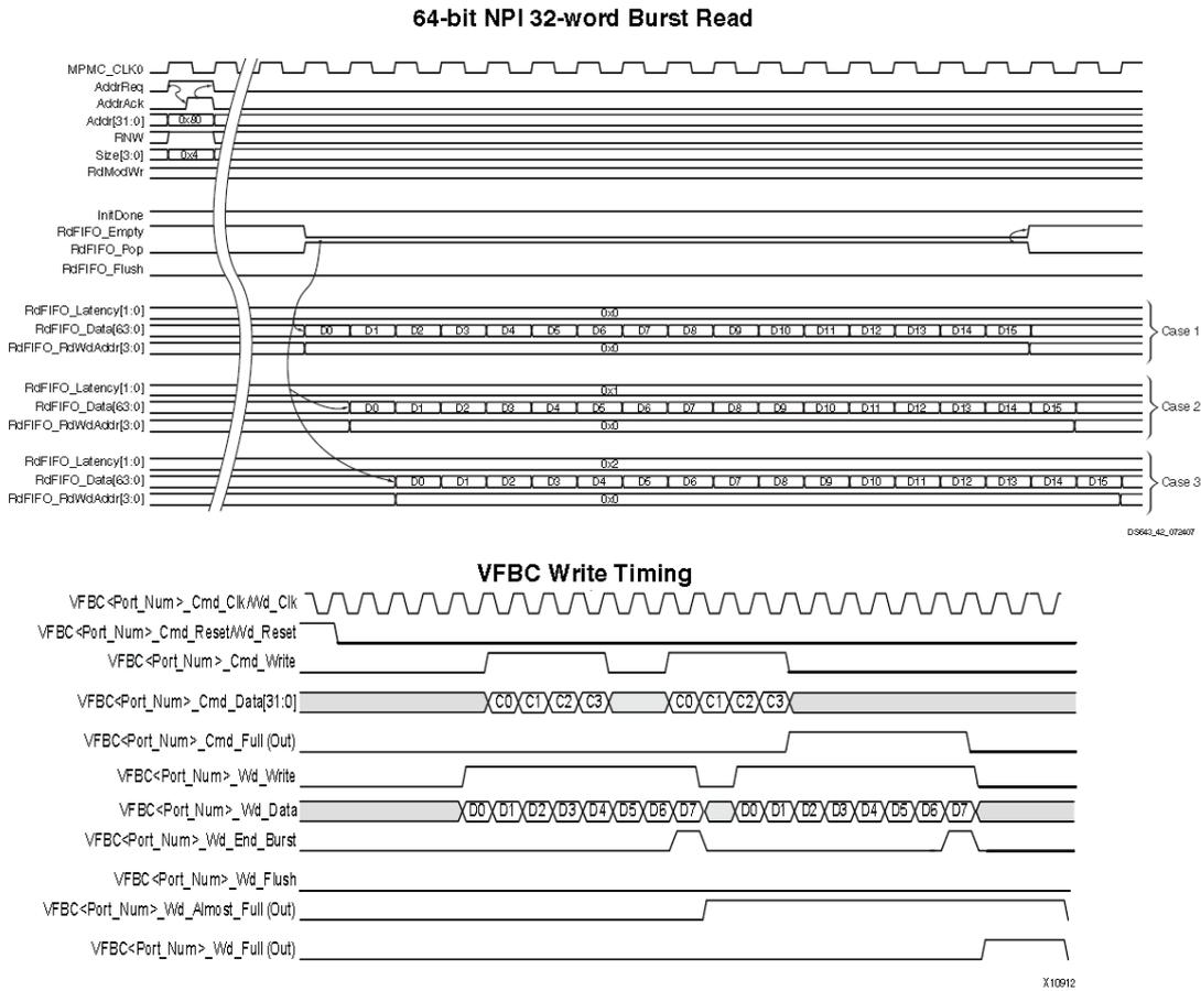
**Figure 3.14:** MPMC transaction timing diagrams - On the top, NPI transaction timing diagrams for a 32-word Burst Read. On the bottom, VFBC transaction timing diagrams for a VFBC write. Taken from [66].
