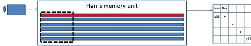
**Figure 4.39: Harris memory unit.** - In five BRAMS will be stored the last five lines of the images. This BRAMS are swept to generate a window of size 5x5, to feed continuously the Harris arithmetic unit.
