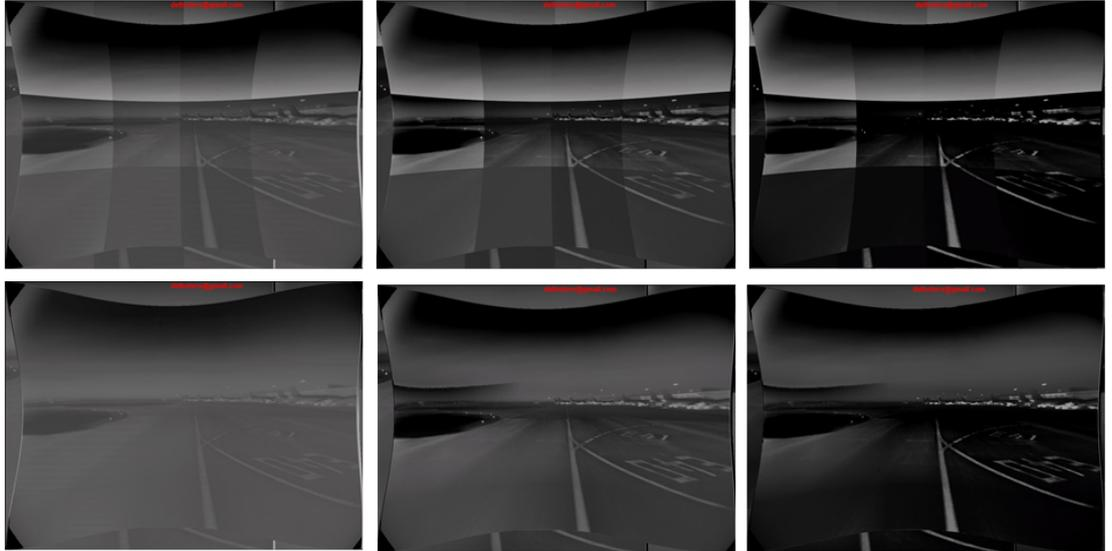
**Figure 5.8: CLAHE output images with different Clip Limits** - On the top, the images before interpolations. On the bottom, the images after the interpolation. From left to right, the Clip Limit is increased.
