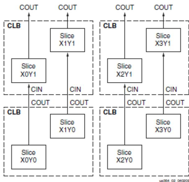
Figure 3.3: CLB block diagram - Taken from [57]
