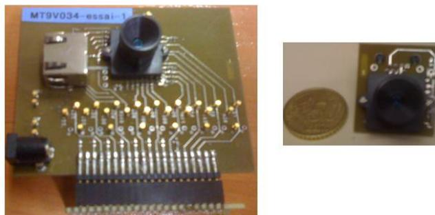
**Figure 5.22: Micro camera developed at LAAS for the camera Belt** - For a future upgrade, we would like to replace the Terasic cameras with smaller cameras with a LVDS connection allowing for longer separation distances between the cameras
