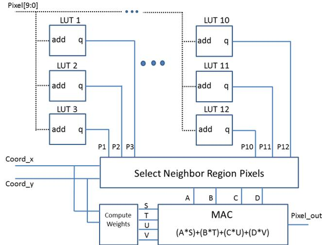
**Figure 4.11: CLAHE LUT interpolation** - The diagram represents the 12 LUT's used to transform the input pixel. Each new pixel is transformed simultaneously using the 12 LUT's. From the 12 transformed pixels, a module selects the necessary pixels to implement an interpolation. The selection and the weight of this pixels depends of the coordinates  $(Coord_x, Coord_y)$ .
