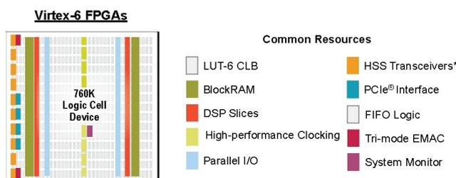
Figure 3.4: Virtex 6 column architecture. - Taken from [58]
