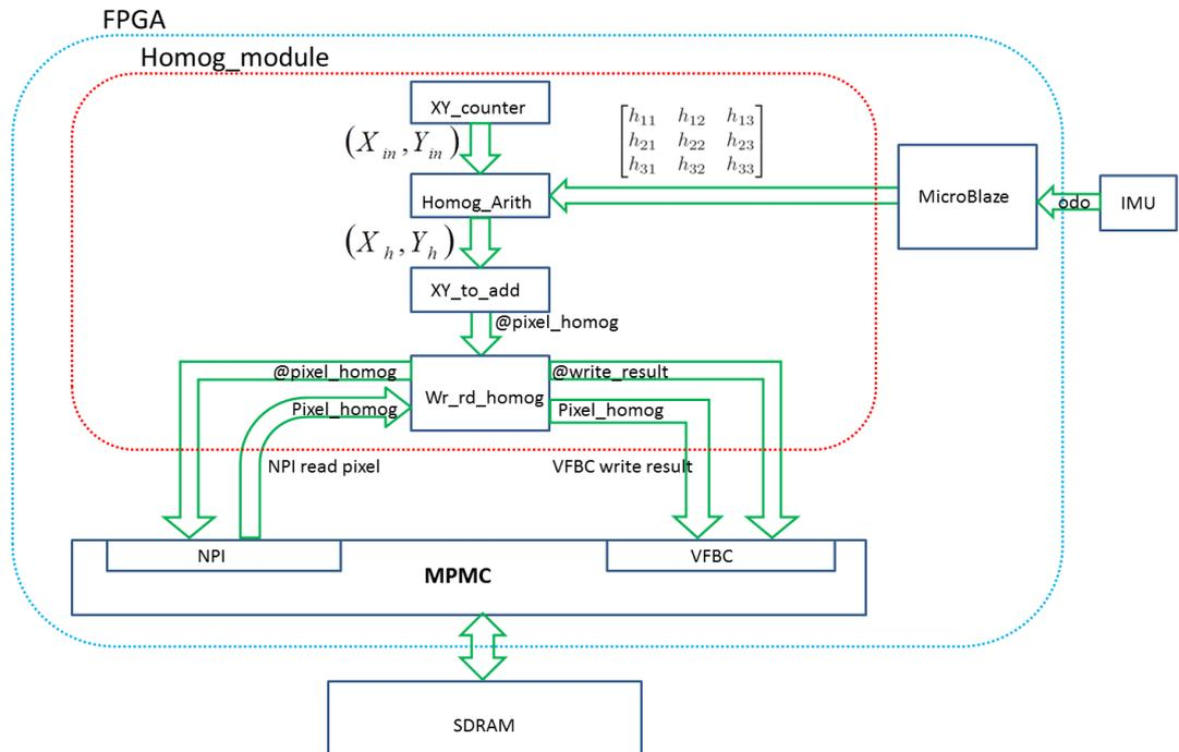
**Figure 4.15: Homography module without Cache memory** - This module implements the homography of an image. The main disadvantage of this module is that the accesses to the memory SDRAM are done in byte mode, with random access, which implies a time penalization.
