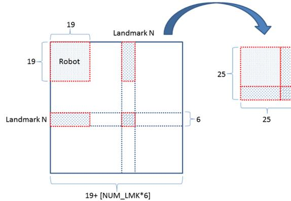
**Figure 2.18: RT-SLAM decomposition of  $P$  before implementing  $HPH^t$**  - Instead of process the entire matrix, in RT-SLAM each landmark is processed individually. This way only a sub-matrix of  $25 \times 25$  must be processed. The sub-matrix is composed of a  $19 \times 19$  matrix, which corresponds to the robot representation, plus the elements corresponding to the interest landmark.
