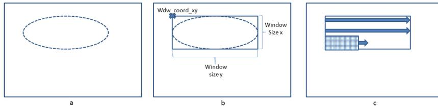
**Figure 4.42: Active Search** - On the left (a), the uncertainty ellipse. On the middle (b), the ellipse is approximated with a rectangle. On the right (c), the rectangle is swept to implement the correlations with the signature of the interest Landmark.
