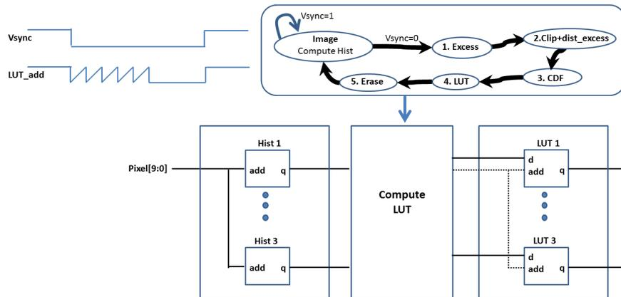
**Figure 4.10: CLAHE histogram processing architecture** - A two set of BRAMS are used in the CLAHE implementation: The first set is used to compute the histograms for each sub-image, and second set is used to store the LUTs for each sub-image.
