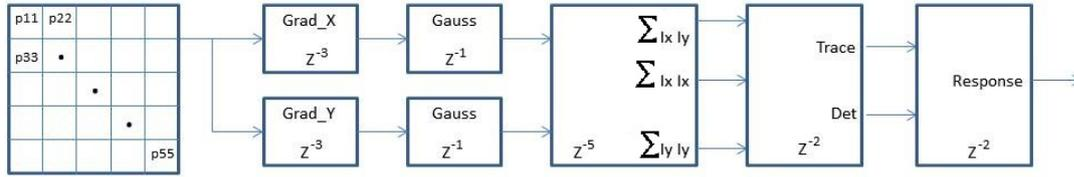
**Figure 4.40: Harris Arithmetic Unit** - This module implements all the arithmetic operation necessary to compute the Harris response given by the equation 2.33. For each pixel, using the window around the interest pixel, a response will be computed on the fly.
