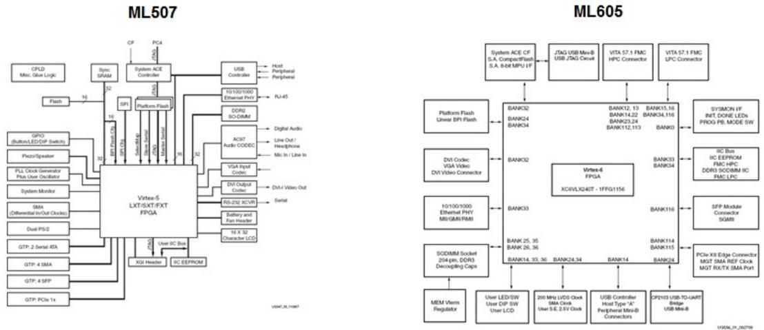
**Figure 5.44: ML507 and ML605 Block diagrams** - On the left the ML507 block diagram, this development kit includes a Virtex 5 FPGA (with PowerPC processor), a DDR2 Memory, Compact Flash memory, PCIe connectors, Ethernet connectors, etc. On the right, the ML605 Block diagram, this development kit includes a Virtex 6 FPGA, a DDR3 Memory, Compact Flash memory, PCIe connectors, Ethernet connectors, etc.
