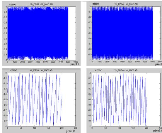
**Figure 5.10: Graphic of quantization error of the homography module** - The difference between the VHDL and the Simulink model response corresponds to the fractional part discarded in the FPGA implementation. For this test the parameters of the homography matrix were constant.
