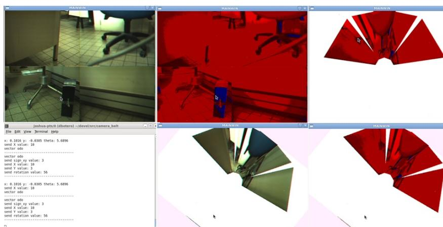
**Figure 5.21: Occupancy grid** - Using the four cameras, the algorithm developed by [86] was applied to each one of the four cameras. Then using a table, an occupancy grid was generated with the information of the obstacles. The occupancy grid was rotated and translated according to the information acquired from the odometry of the robot.
