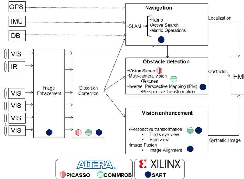
**Figure 1.3: Block diagram of modules and projects** - In this thesis we show different architectures for tasks involved in ADAS. Architectures for Navigation, Obstacle detection and Vision enhancement are described.
