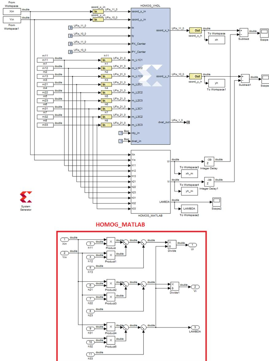
**Figure 5.9: Simulink homography verification diagram** - Verification of the arithmetic unit of the Homography module using System generator of Xilinx. Output from a black box with the VHDL is compared with a Simulink model
