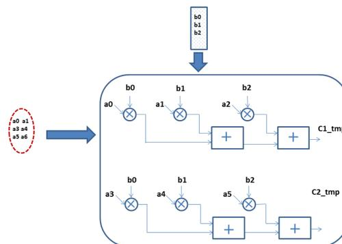
Figure 4.35: Multiplication Systolic Array - A systolic array composed of floating point additiners and multipliers.
