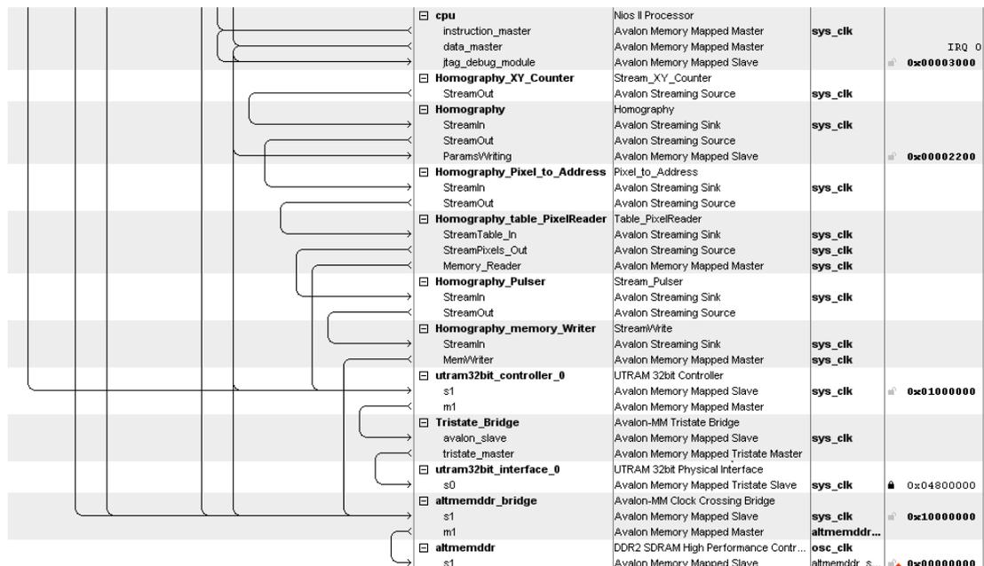
**Figure 3.19: Avalon Switch Fabric** - The diagram was generated with SOPC builder of Altera, this system implements a Homography of an image. The NIOS2 processor configures the Homography parameters through an Avalon Memory Mapped Interface. In this system, there are two memory components, a DDR2 memory and a SRAM memory, both of them are Avalon Memory Slaves.
