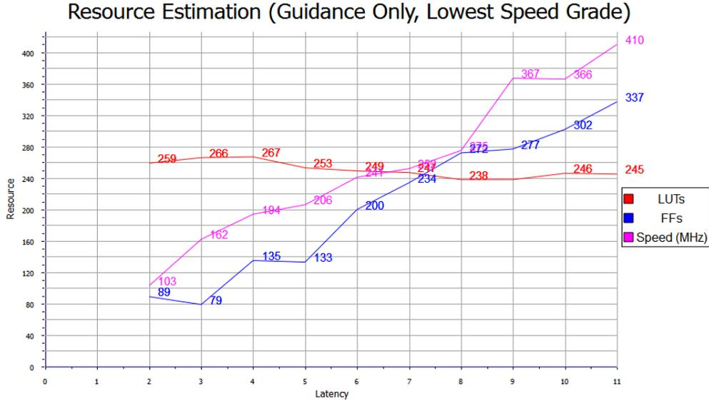
**Figure 3.12: Floating point addition latency, operation frequency and resources** - The graph represents latency, maximum operation frequency and resources for different configurations of the single precision floating point addition generated with the Xilinx IPCore tool.
