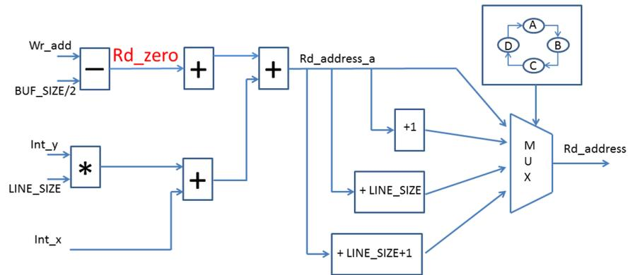
**Figure 4.5: Read Address generator** - The read addresses are generated using the write address ( $\text{Wr\_add}$ ), the integer parts of the coefficient ( $\text{Int\_x}$  and  $\text{Int\_y}$ ), the line size and the buffer size.
