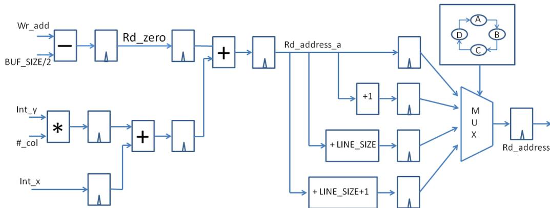
**Figure 4.6: Read Address generator fully pipelined** - This module implements the same function than its version without pipeline, but because the critical path is smaller, it can work at higher frequencies.
