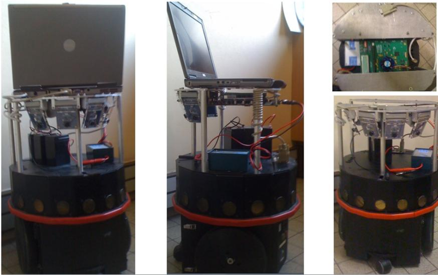
**Figure 5.46: Commrob platform** - The platform was mounted in a Scout robot. We installed a Stratix 3 development kit connected with four Terasic cameras. The result images were displayed in a computer.
