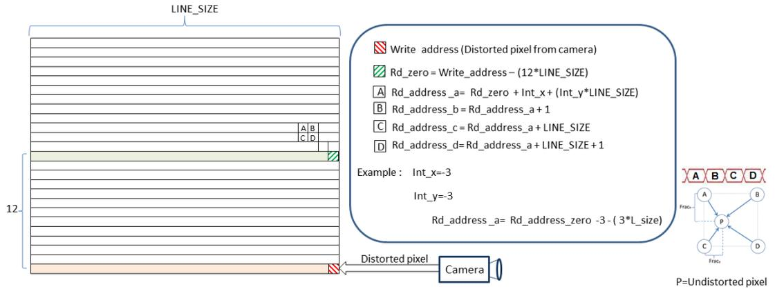
**Figure 4.4: Internal Memory Management** - When a new pixel arrives from the camera, it is stored in the memory. At the same time, an undistorted pixel will be generated using the interpolation of the vicinity pixels (A, B, C and D). This figure represents an illustrative example using a small buffer size of 24 lines. The final implementation has a buffer size of 256 lines to support a max distortion of  $\pm 128$  lines.
