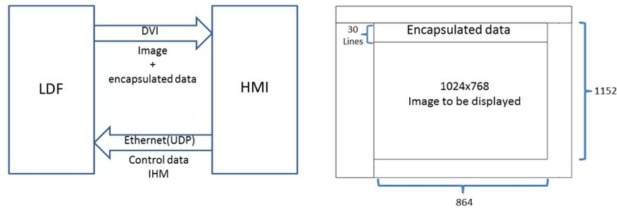
**Figure 5.33:** Interface HMI and LDF - .
