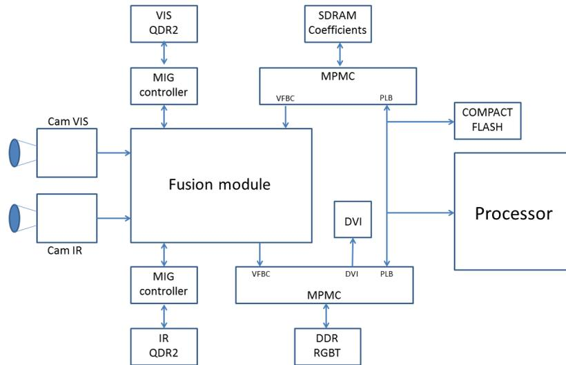
Figure 4.17: Fusion IR and VIS using QDR2 memory -
