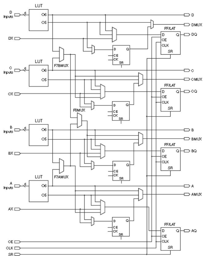
Figure 3.2: SLICE Virtex 6 simplified block diagram - Taken from [57]
