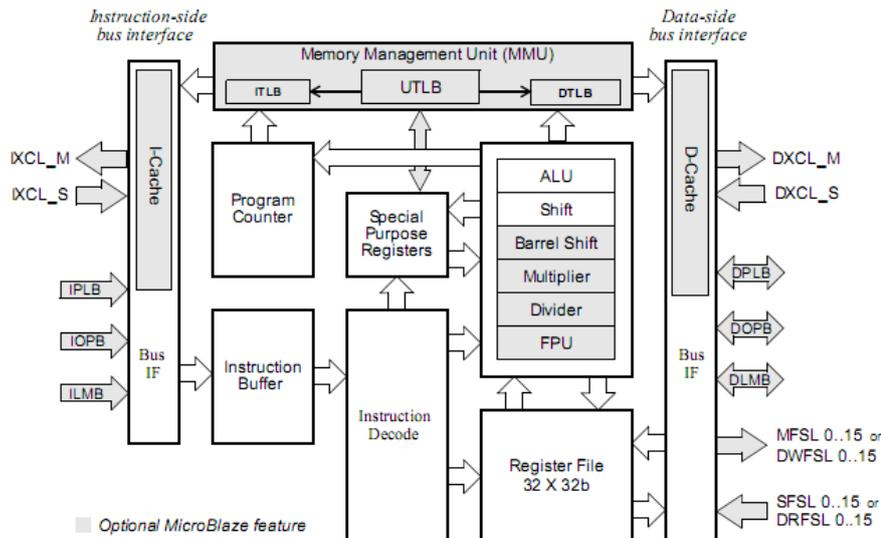
Figure 3.15: MicroBlaze block diagram - Taken from [70].
