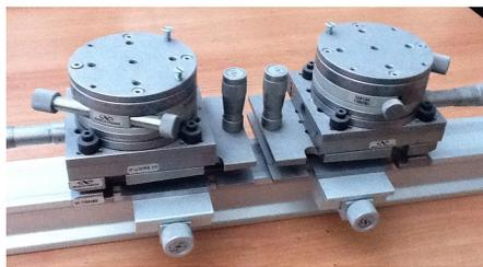
**Figure 2.12: Configurable mechanic base for stereo vision -**
