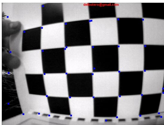
Figure 5.28: Harris point detector output - The corners are highlighted with a square.
