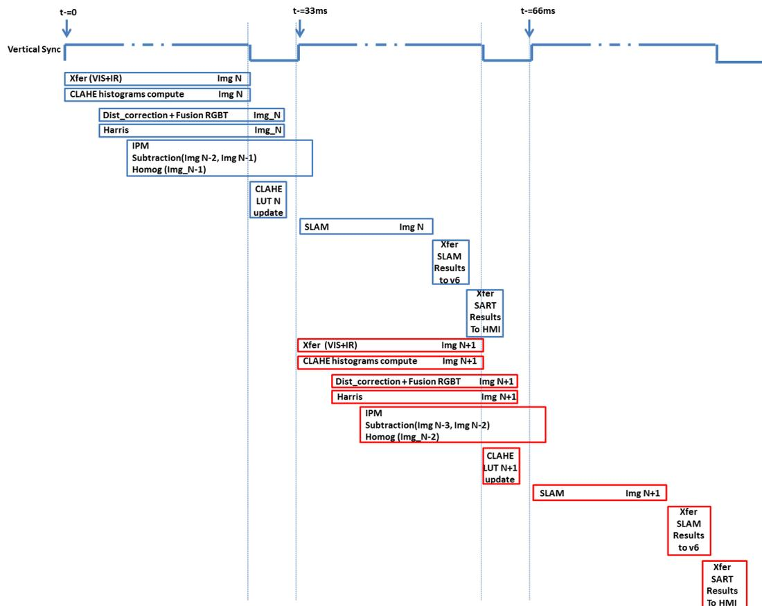
Figure 5.38: Timing representation of SART processing algorithms. - .
