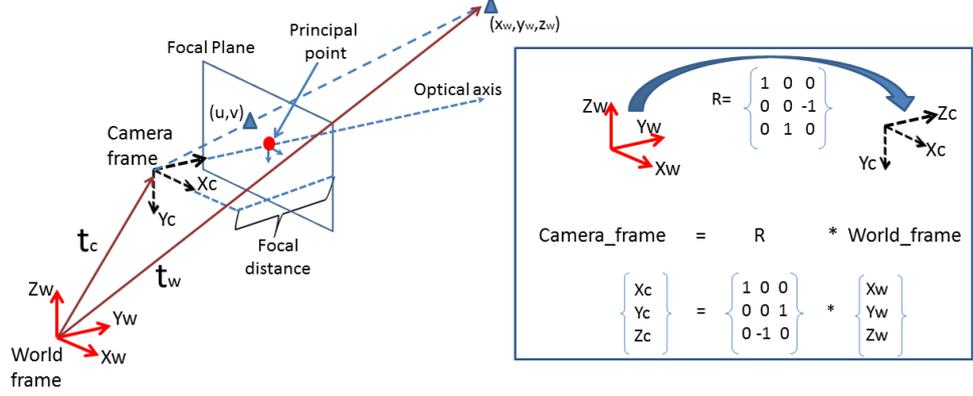
**Figure 2.1: Pinhole Camera Model** - In the figure, the camera frame is parallel to the world frame. For this reason, in this ideal example, the components of the rotation Matrix  $R$  are just 1, 0 and -1. Physically, it corresponds to have the camera parallel to the ground plane and the optical axis aligned with the Y-axis of the world frame.
