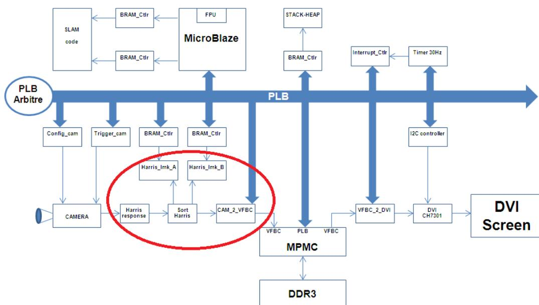
**Figure 4.41: Harris unit integrated to the PLB system** - In the ellipse on the bottom left, we highlight the Harris pipeline. Images coming from the camera are processed on the fly. The module sort Harris, organize the response to choose the best response in each sub-image. A ping pong schema is used to send the Harris information to the Host processor.
