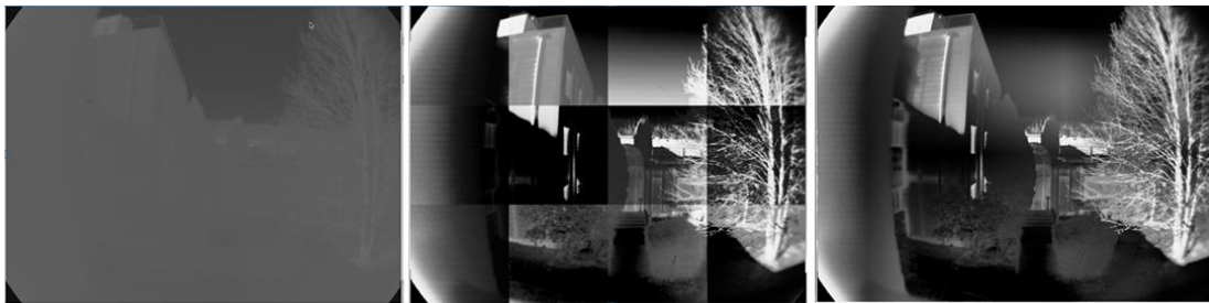
Figure 5.7: CLAHE intermediary images - On the left, the input image. In the middle, the intermediary image, here each sub-image is processed independently. On the right, the output image after implementing interpolations.
