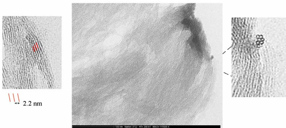
Figure 1.- TEM micrographs of synthetic imogolite.
