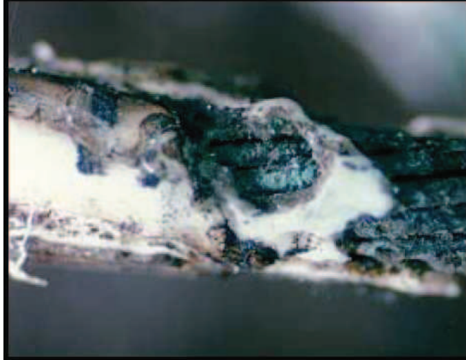
Figure 1.12: A damaged cable due to its presence in a high moisture environment.
