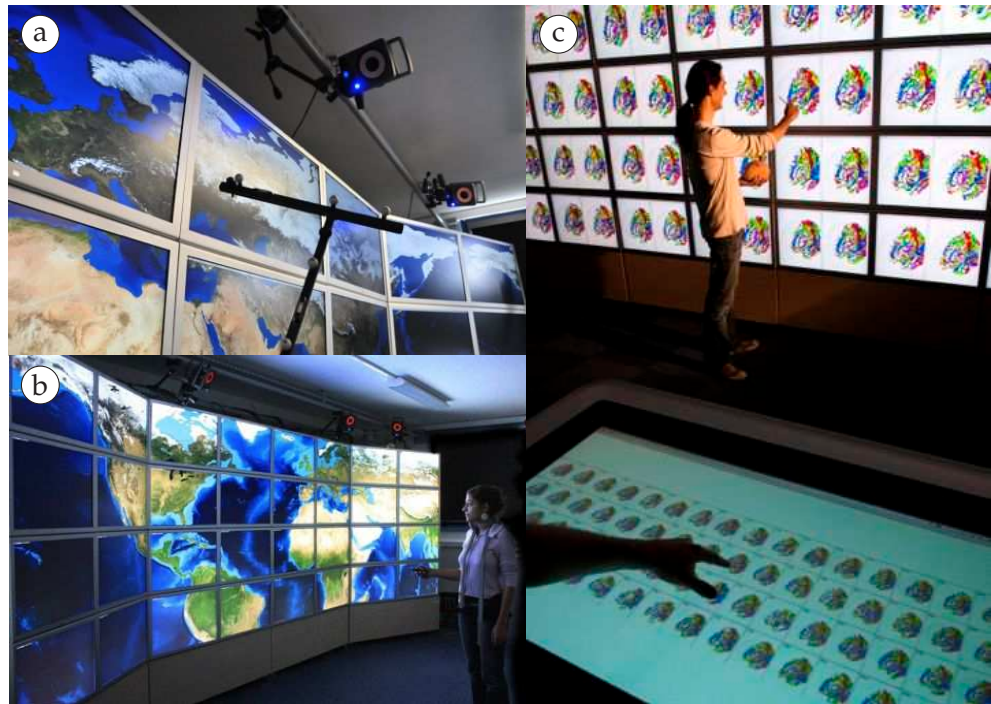
Figure A.1: The wild platform: a) VICON tracking system, b) user pointing to the wall with a hand-held device, c) a large wall display used in combination with an interactive table.
