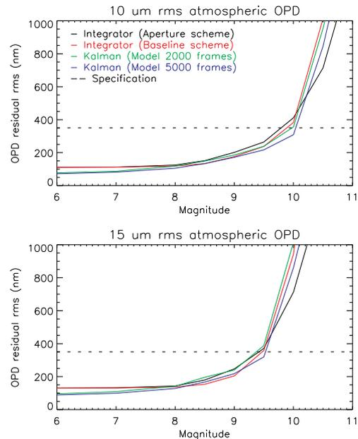
**Fig. 8.** OPD residuals as a function of magnitude. The simulated atmospheric OPD are 10  $\mu\text{m}$  rms (top) and 15  $\mu\text{m}$  rms (bottom). The vibration level is 150 nm rms per baseline, and flux variations are due to 15 mas rms residual tip-tilt of the beams.
