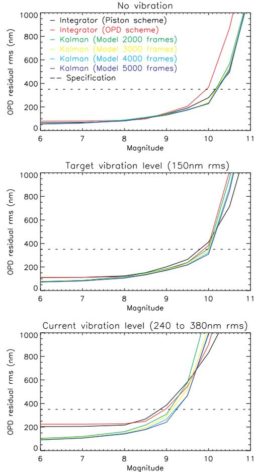
**Fig. 6.** OPD residuals as a function of magnitude. Top: no vibration; middle: Expected vibration level at VLTI; bottom: Current vibration level at VLTI. The atmospheric OPD level is 10  $\mu\text{m}$  rms and, the residual tip-tilt of the beams is 15 mas rms.
