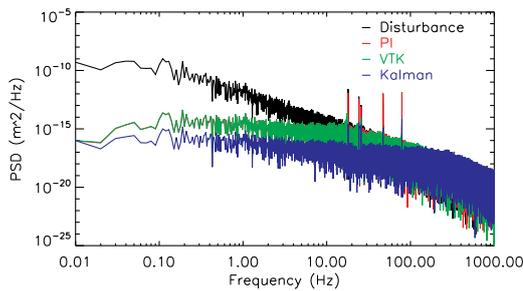
**Fig. 12.** Power spectrum density of the disturbance and of the OPD residuals using the three controllers, for star of magnitude 6, with no flux variation. The simulated disturbance are the atmospheric OPD and the 5 sinusoidal vibrations described in Table 8, scaled to a total standard deviation of 350 nm rms.
