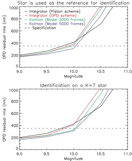
**Fig. 9.** OPD residuals as a function of magnitude, for  $10 \mu\text{m}$  rms atmospheric OPD,  $150 \text{ nm}$  rms vibration OPD, and  $15 \text{ mas}$  rms residual tip-tilt of the beams. Top: disturbance model is computed from a POL sequence acquired on the star itself. Bottom: the model is computed observing a brighter object ( $K = 7$ ).
