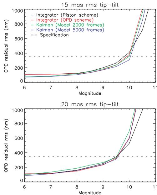
**Fig. 7.** OPD residuals as a function of magnitude, with flux variations due to 15 mas rms (top) and 20 mas rms (bottom) residual tip-tilt. The OPD disturbances are 10  $\mu\text{m}$  rms atmospheric OPD and 150 nm rms vibration OPD.
