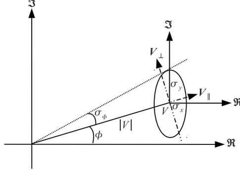
**Fig. A.1.** Representation of the complex visibility  $V$  and of the noise  $\sigma_v$  in the complex plane ( $V$ ,  $\Re$ ,  $\Im$ ) and in the radial basis ( $V$ ,  $V_{\parallel}$ ,  $V_{\perp}$ ).
