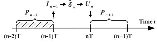
Fig. 5. Representation of the simulated discretized time-scheme. At iteration  $n$ , the OPDs  $\hat{\delta}_n$  are estimated from the image  $I_{n-1}$  delivered at the end of the previous iteration, which is representative of piston disturbances  $P_{n-1}$  integrated between time steps  $n-2$  and  $n-1$ . The corresponding correction on the delay lines  $U_n$  is applied during the following iteration.
