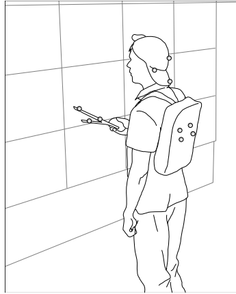
Figure C.1: Apparatus of the experiment: participants wore a hat and a backpack mounted with passive infrared markers. A handheld device was also tracked for pointing.
