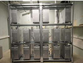
A cluster of 16 computers that communicate via a dedicated high-speed network through a front-end computer; each has two high-end nVidia 8800GT graphics cards and drives two screens of the wall display.
