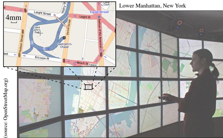
**Figure 4.1:** The interactive wall-sized (5.5m × 1.8m) ultra-high-resolution (20 480 × 6 400 = 131 million pixels) display used for our studies. Inset: magnification of a 9cm × 5cm area.
