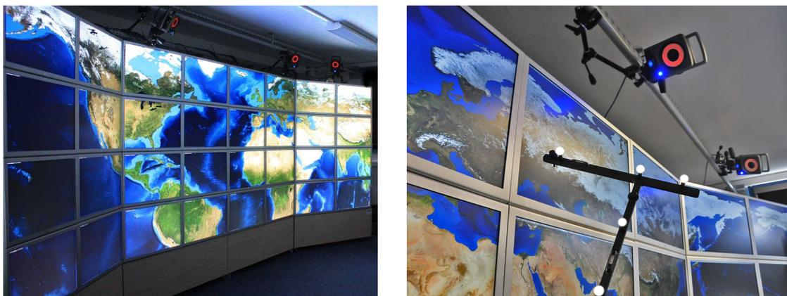
**Figure 4.6:** The platform used for the experiment: thirty-two 100 ppi screens (left picture), VICON cameras and VICON markers (white dots on the foreground object, right picture).
