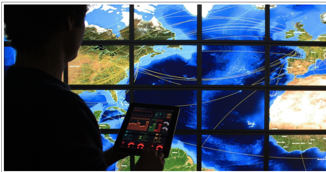
Figure 6.1: Interacting with a wall-sized display using a tablet that features both control widgets and an area dedicated to high-precision remote pointing (top-left).
