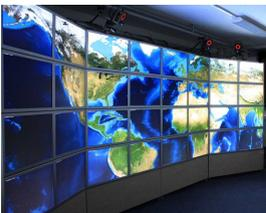
An ultra-high-resolution  $5.5 \times 1.8$ -meter display made of  $8 \times 4$  tiled 30" desktop screens at approximately 100 ppi; it provides a unified  $20480 \times 6400$  pixels display, or  $22080 \times 7360$  pixels if we consider "virtual" pixels under the screen bezels.
