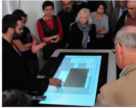
A  $2 \times 1$  meter interactive table with FTIR technology that can track up to 32 simultaneous contact points with an output  $1920 \times 1080$  resolution.
