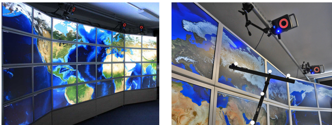
Figure 4.6: The platform used for the experiment: thirty-two 100 ppi screens (left picture), VICON cameras and VICON markers (white dots on the foreground object, right picture).
