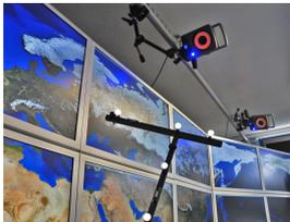
A VICON<sup>2</sup> motion-capture system with 8 to 10 200 Hz cameras that track passive IR retro-reflective markers with sub-millimeter accuracy; the location and orientation of physical objects mounted with these markers can thus be tracked very precisely.
