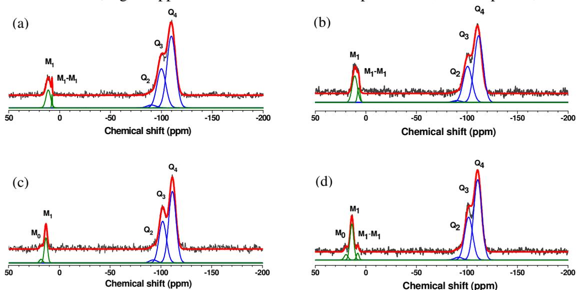
Figure 17  $^{29}\text{Si}$  MAS NMR spectra of the materials (a) LUSC0-E\_rt, (b) LUS-T0-E\_rt, (c) LUSC0-E\_rt-OH, (d) LUS-T0-E\_rt-OH; M1-M1 stands  $M_1''$  at 7 ppm at the right hand side of the  $M_1$  signal.
