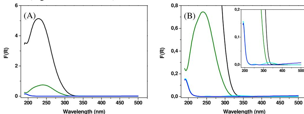
Figure 1 UV spectra of Ti incorporated silica materials and after dilution using LUS-cal as diluent. Black line: initial sample; green line: initial sample after dilution; blue line: LUS without surfactant calcined at 550 °C for 10 h; cyan line: LUS with surfactant TMABr calcined at 550 °C for 10 h.
