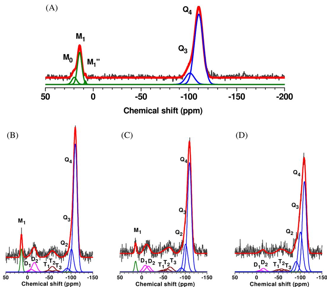
Figure 6  $^{29}\text{Si}$  MAS NMR spectra of the materials (A) LUS-100E, (B) LUS-100E-380, (C) LUS-100E-480, and (D) LUS-100E-580. Peak position (ppm):  $Q_4 = -111.0 \pm 0.3$ ,  $Q_3 = -101.9 \pm 0.3$ ,  $Q_2 = -91.8 \pm 0.4$ ;  $M_1 = 14.1 \pm 0.1$ ,  $M_0 = 18.6 \pm 0.4$ ,  $M_1'' = 6.7 \pm 0.1$ ,  $T_3 = -65.4 \pm 0.2$ ;  $T_2 = -57.1 \pm 0.1$ ;  $T_1 = -49.0 \pm 0.1$ ;  $D_2 = -15.4 \pm 0.4$ ;  $D_1 = -8.2 \pm 0.1$ .
