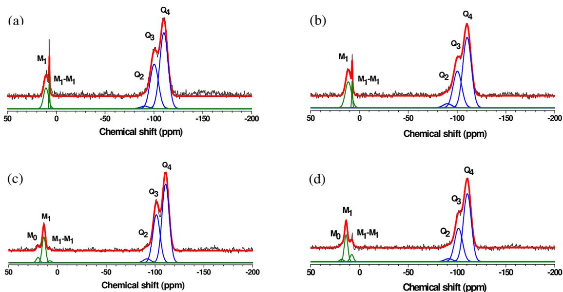
Figure 11 Single echo  $^{29}\text{Si}$  MAS NMR spectra of the materials (a) LUS-C0-E, (b) LUS-T0-E, (c) LUS-T0-E-OH, (d) LUS-T0-E-OH. Gray line: raw curve, red line: cumulative curve, blue lines: fits of  $Q_n$  species silicon, green lines: fits of  $M_n$  species silicon.
