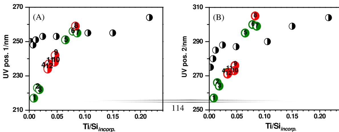
Figure 23 The relevance between the incorporation amount of Ti and UV absorption at (A) pos. 1 and (B) pos. 2 (black circle: LUS-Ti-n; green and red circles: LUS-E-Ti-n).
