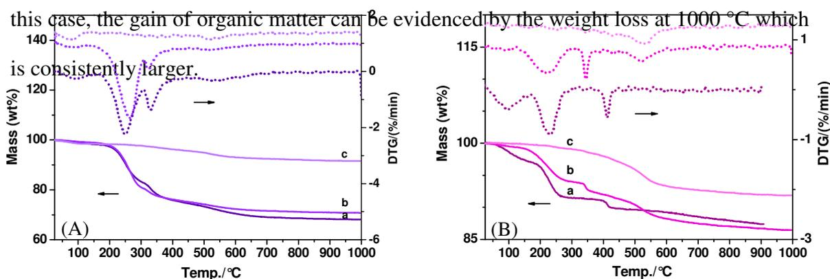
Figure 15 TG-DTG traces of materials functionalized by EBDMS at room temperature with (A) CTA<sup>+</sup> and (B) TMA<sup>+</sup> as protecting group. In (A): a, LUS-C50; b, LUS-C50-E<sub>rt</sub>; c, LUS-C50-E<sub>rt</sub>-OH; In (B): a, LUS-T50; b, LUS-T50-E<sub>rt</sub>; c, LUS-T50-E<sub>rt</sub>-OH.
