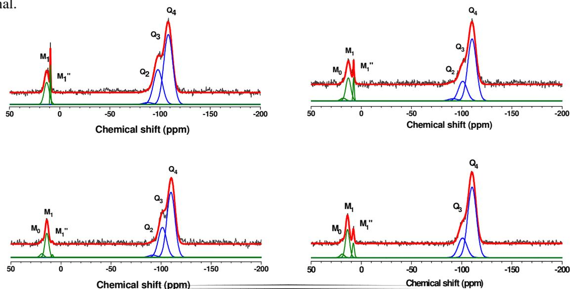
Figure 18  $^{29}\text{Si}$  MAS NMR spectra of materials (a) LUS-C50-E<sub>rt</sub>, (b) LUS-T50-E<sub>rt</sub>, (c) LUS-C50-E<sub>rt</sub>-OH, (d) LUS-T50-E<sub>rt</sub>-OH.
