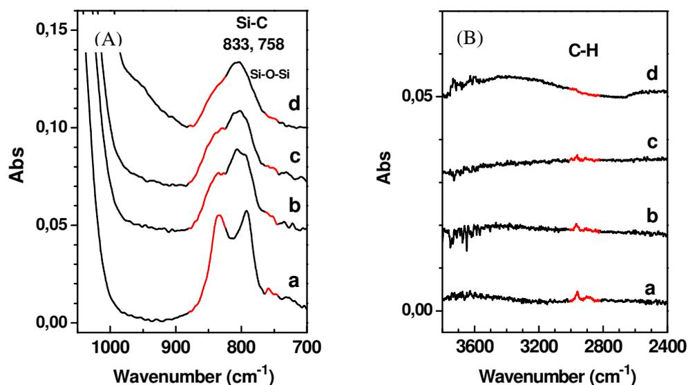
Figure 4 FT-IR spectra monitoring the thermal treatment to the materials LUS-100E in the (A) inorganic region and (B) organic region, respectively. a, LUS-100E; b, LUS-100E-380; c, LUS-100E-480; d, LUS-100E-580.
