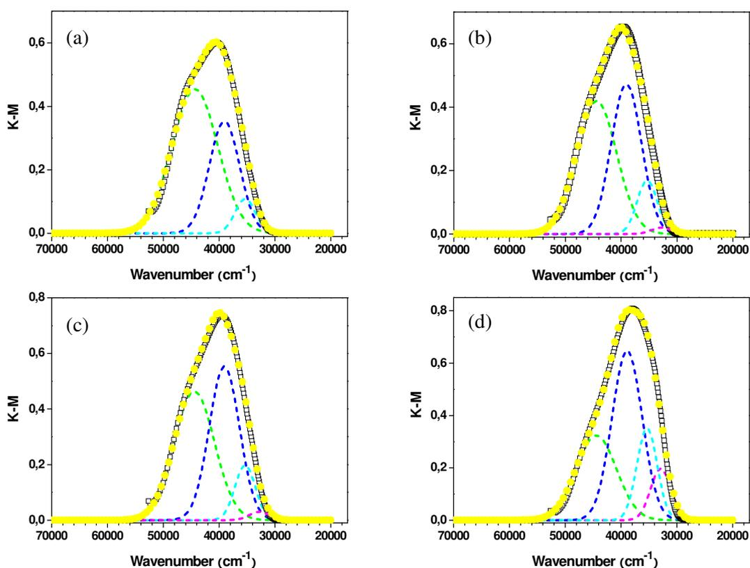
Figure 6 UV-vis spectra deconvolution for LUS-Ti with Ti/Si ratio of (a) 0.0072 (0.46 wt%), (b) 0.0240 (1.55 wt%), (c) 0.0487 (3.01 %), (d) 0.2160 (10.65 wt%), Ti weight percentage in the parentheses. Hollow square for the raw curve, yellow circle for the cumulative curve, dash lines for fits (detail in Table 1).
