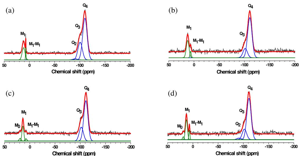
Figure 10 Single echo  $^{29}\text{Si}$  MAS NMR spectra of the materials (a) LUS-C50-E, (b) LUS-T50-E, (c) LUS-C50-E-OH, (d) LUS-T50-E-OH. Gray line: raw curve, red line: cumulative curve, blue lines: fits of  $Q_n$  silicon species, green lines: fits of  $M_n$  silicon species.
