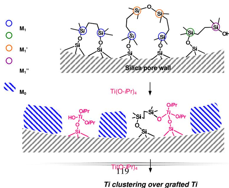
Scheme 4 Possible heterogeneous surface functionalized by EBDMS group and Ti species. M<sub>1</sub> and M<sub>1</sub>" refer to the Si signals observed in <sup>29</sup>Si-NMR.
