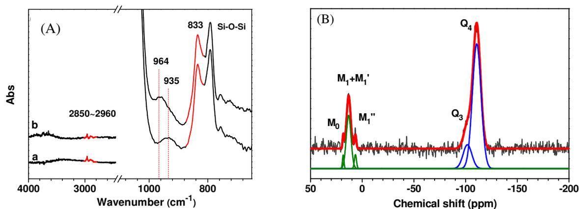
Figure 19 (A) FT-IR spectra of materials (a) LUS-E-OH, (b) LUS-E-Ti-11 and (C)  $^{29}\text{Si}$  MAS NMR of LUS-E-Ti-11. Normalized intensity of  $833\text{ cm}^{-1}$   $\nu_{\text{Si-O}}$  peak: (a)  $0.28 \pm 0.01$ , (b)  $0.31 \pm 0.01$ .
