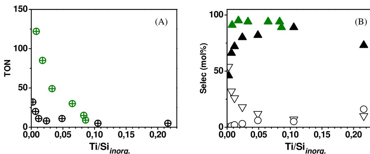
Figure 24 (A) The TON per Ti atom and (B) selectivity of epoxidation of cyclohexene on the Ti/Si incorporated ratios of LUS-E-Ti and LUS-Ti. In (A), green circles: LUS-E-Ti- $n$  ( $n = 1, 3-5, 7-8$ ); black circle: LUS-Ti- $n$  ( $n = 1-7$ ). In (B), green solid triangle: epoxide product on LUS-E-Ti- $n$ ; black solid triangle: epoxide product on LUS-Ti- $n$ , black inverted triangles: allylic by-products on LUS-Ti- $n$ , black circle: diol by-products on LUS-Ti- $n$ .
