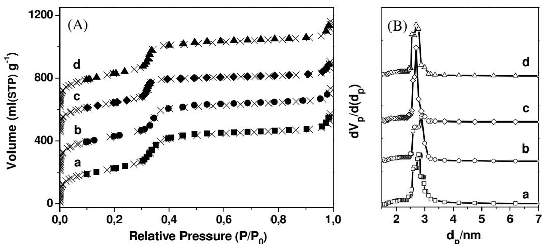
Figure 3 (A) N<sub>2</sub> sorption isotherms and (B) pore size distribution of (a) LUS, (b) LUS-550 (offset of + 200 ml (STP) g<sup>-1</sup>), (c) LUS-100E-580 (offset of + 450 ml (STP) g<sup>-1</sup>) and (d) LUS-100TMS-600 (offset of + 600 ml (STP) g<sup>-1</sup>).
