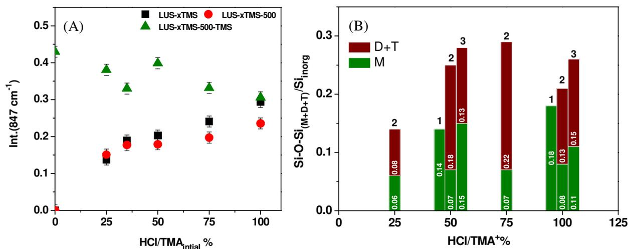
Figure 14 Evolution of TMS coverage versus HCl/TMA% reported in molar ratio by (A) the IR intensity of peak at 847 cm<sup>-1</sup> and (B) the quantitative <sup>29</sup>Si MAS NMR spectra. In (B), Si-O-Si<sub>(M+D+T)</sub>/Si<sub>inorg</sub> =  $\Sigma[1*(M_1+D_1+T_1)+2*(D_2+T_2)+3*T_3] / \Sigma Q_i$  (i = 2-4); bar marked 1: LUS-xTMS, marked 2: LUS-xTMS-500, marked 3: LUS-xTMS-500-TMS.
