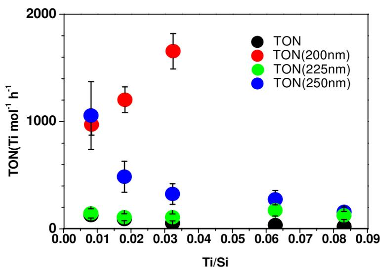
Figure 9 Recalculated TON of the epoxidation of cyclohexene on the LUS-E-Ti-n materials has been recalculated using the coefficient constant  $\varepsilon_n$ . Black square line: TON; pink square line: TON/(200+225 nm) Ti mol%; green triangle line: TON/(225 nm) Ti mol%; TON/(200+225+255 nm) Ti mol%.
