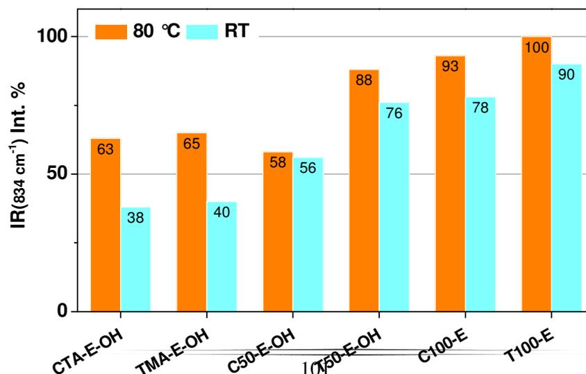
Figure 16 Evolution of the normalized IR band at  $834\text{ cm}^{-1}$  depending on the nominal masking level and the type of ammonium after EBDMS grafting at 25 or 80 °C and mask removal.
