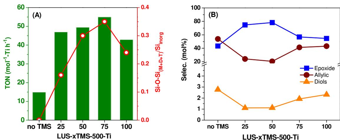
Figure 17 Dependence of (A) the TON consistent with Si-O-Si linkage from organic moieties and (B) the products selectivity on the LUS-xTMS-500-Ti (x = 0, 25, 50, 75 and 100).
