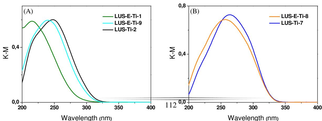
Figure 22 UV-vis spectra for (A) the similar Ti incorporation loading and (B) the same UV-vis spectra for the different Ti incorporation loading on the LUS-TiPr and LUS-E-TiPr.
