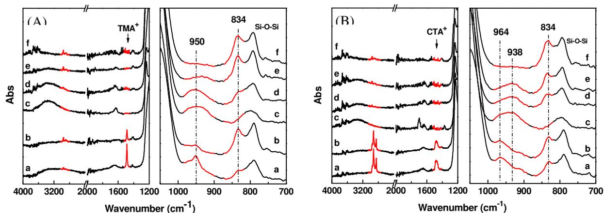
Figure 14 FT-IR spectra for monitoring the synthesis of materials using (A)  $\text{CTA}^+$  and (B)  $\text{TMA}^+$  as surface protecting groups to silylation at room temperature. In (A): a, LUS-T0-E<sub>rt</sub>; b, LUS-T50-E<sub>rt</sub>; c, LUS-T100; d, LUS-TMA-E<sub>rt</sub>-OH; e, LUS-T50-E<sub>rt</sub>-OH; f, LUS-T100-E<sub>rt</sub>; a, LUSC0-E<sub>rt</sub>; b, LUS-C50-E<sub>rt</sub>; c, LUS-C100; d, LUS-CTA-E<sub>rt</sub>-OH; e, LUS-C50-E<sub>rt</sub>-OH; f, LUS-C100-E<sub>rt</sub>.
