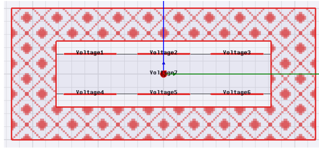
Figure 3.26. Simulation model for the 6-conductor PCB structure
