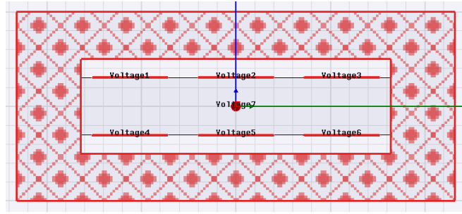
Figure 3.26. Simulation model for the 6-conductor PCB structure
