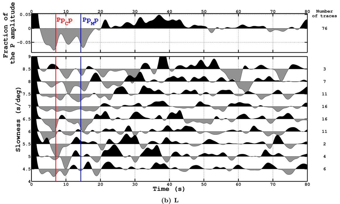
**Figure 4.4:** (a) Q and (b) L components RFs for station AML stacked in several slowness windows, corrected for the (a)  $P_{Ms}$  and (b)  $Pp_{Mp}$  moveouts with a reference slowness of  $6.5 \text{ s}/^\circ$ . The top trace is the stack of the whole data set. The numbers on the right give the numbers of records stacked in each slowness window. The colored lines give the traveltimes computed with the method described in Sec. 4.4.1.
