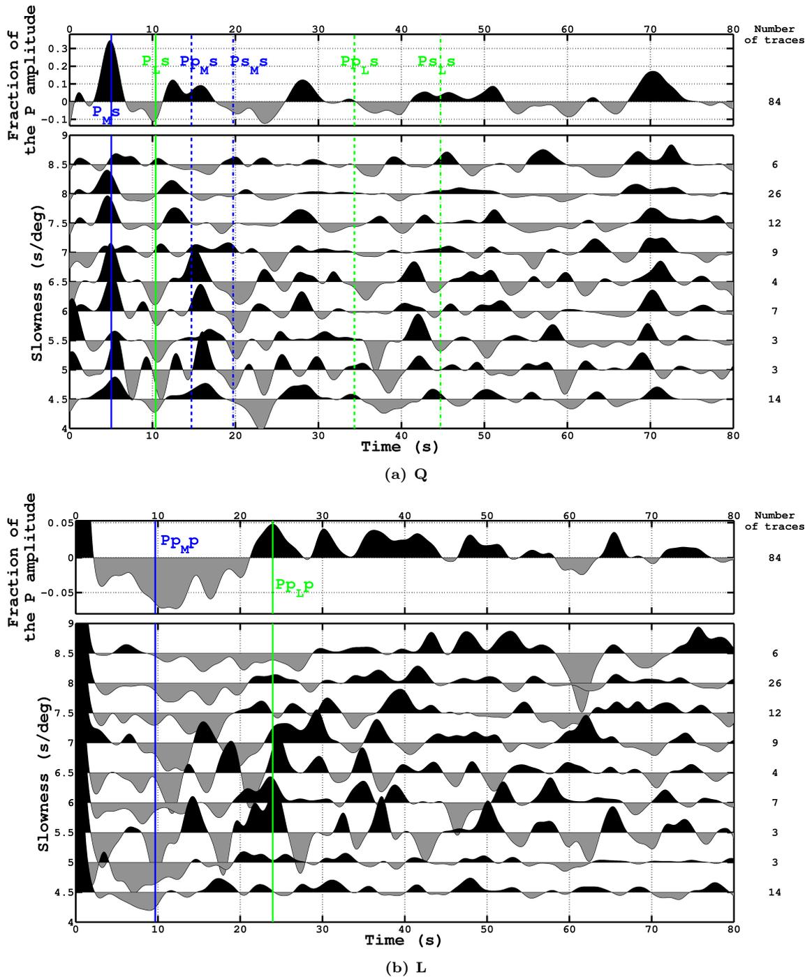
**Figure 4.5:** (a) Q and (b) L components RFs for station BJT stacked in several slowness windows, corrected for the (a)  $P_{Ms}$  and (b)  $P_{PMP}$  moveouts with a reference slowness of  $6.5 \text{ s/deg}$ . The top trace is the stack of the whole data set. The numbers on the right give the numbers of records stacked in each slowness window. The colored lines give the traveltimes computed with the method described in Sec. 4.4.1.
