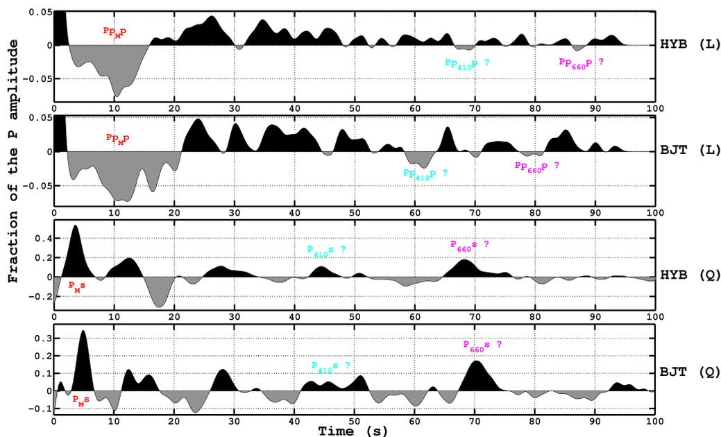
**Figure 4.8:** Most probable positions of the  $P$ -to- $S$  conversions and  $P$  reflections at 410 km (cyan) and 660 km (magenta) MZT discontinuities at HYB (first and third traces) and BJT (second and fourth traces) seismological stations.
