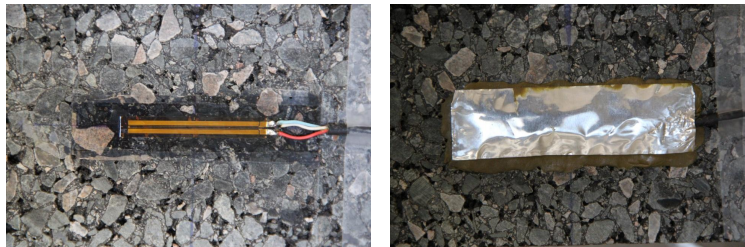
FIGURE 6.1 – Protection de jauge
