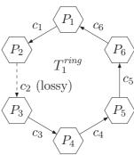
Figure 5.1: Unidirectional ring topology with a lossy channel
