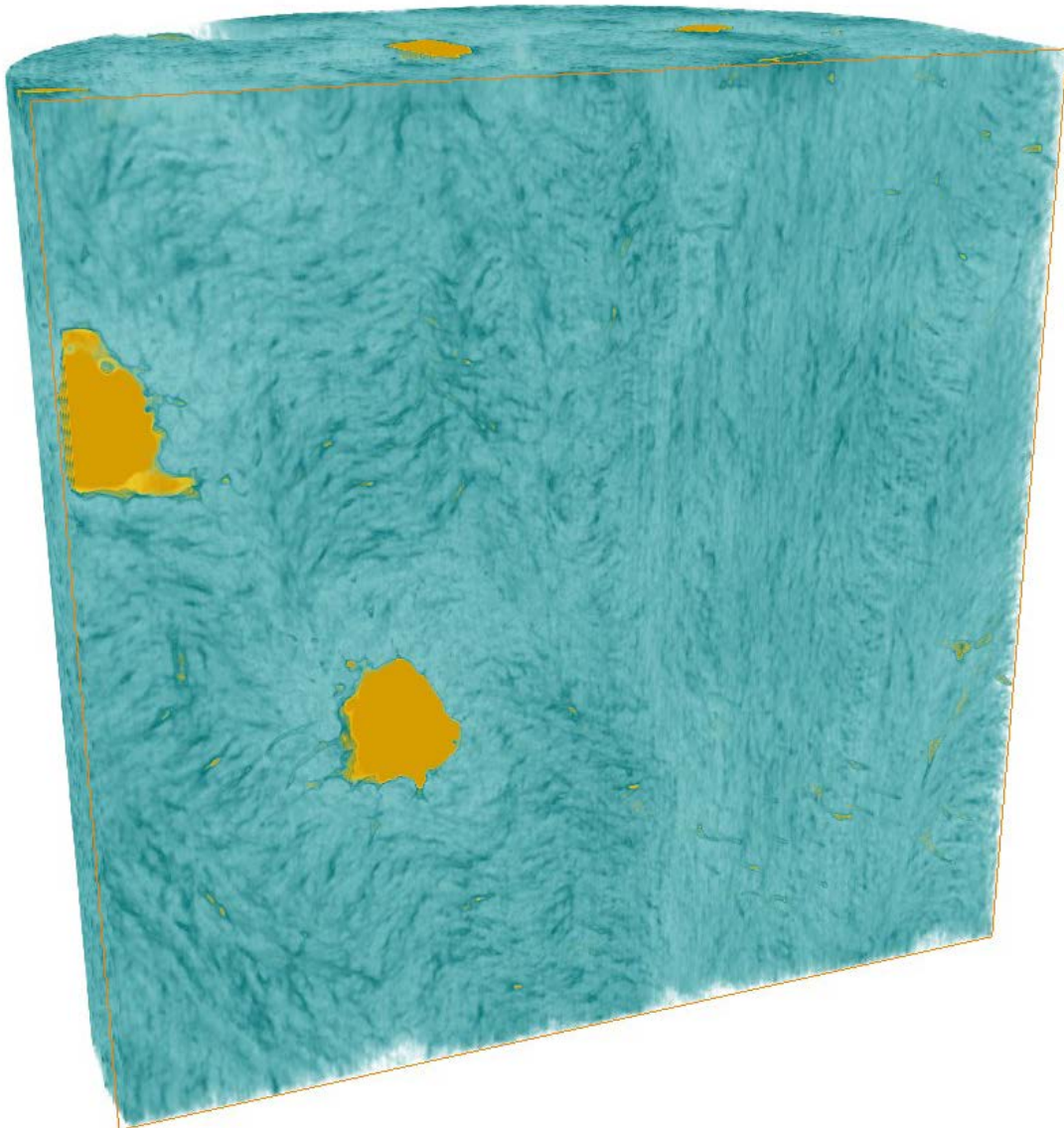
Figure 69 Frontal section through the volume rendering. One can observe that around the cell lacunae the bone matrix appears denser, hence higher degree of mineralization. Pixel size was 60 nm.
