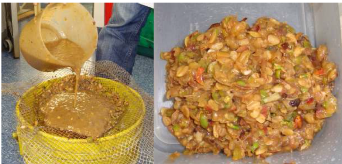
Figure AIII2. Coffee mucilage processing: removal of thick solids composed by coffee grains, pulp and some coffee beans.
