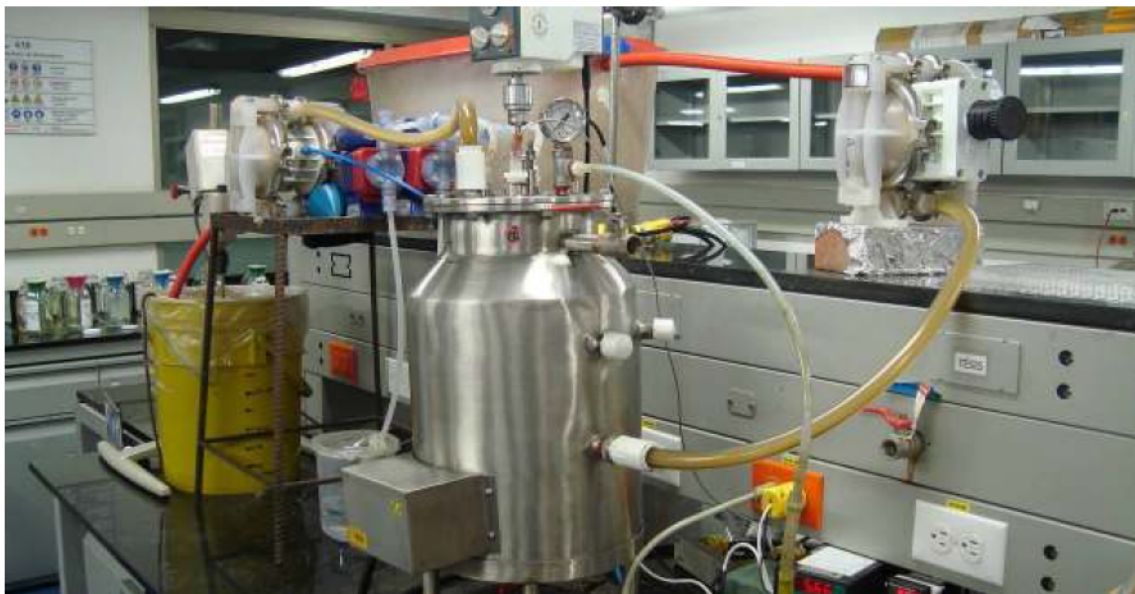
Figure AIII1. Reactor system for hydrogen experiments
