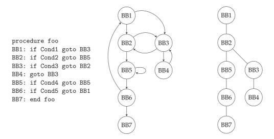
Figure 2.2: Example procedure, its control-flow graph and a dominator tree.
