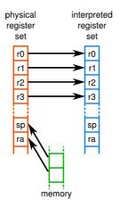
Figure 7.6: Copying the result to the interpreted registers after the call and restoring stack pointer and return address
