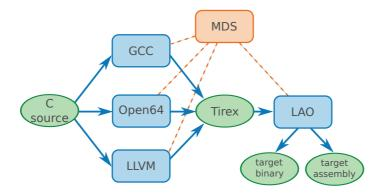
Figure 6.1: Tirex in our toolchain. The MDS supplies target-specific files to build the upstream compilers and LAO code generator. The path from GCC is not yet functional.
