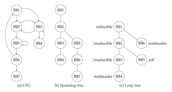
Figure 2.7: An example of a loop tree for given CFG and its spanning tree.
