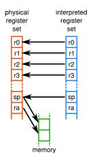
Figure 7.5: Passing arguments before the call, saving stack pointer and return address and switching stack pointers
