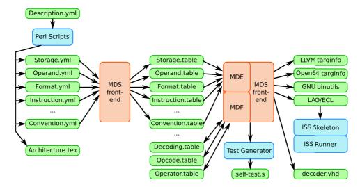
Figure 5.2: MDS (Machine Description System) work-flow.
