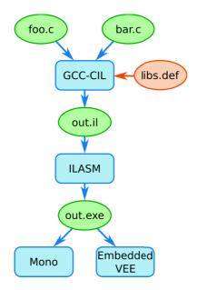
Figure 4.1: GCC-CIL compilation and execution flow
