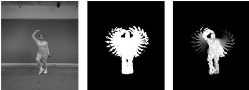
Figure 1.5: The motion energy images (MEI) and motion history images (MHI) of Bobick and Davis [2001].
