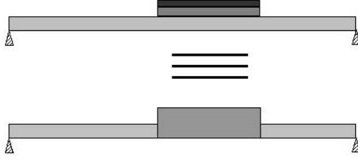
FIG. 2. Single-layer equivalence process applied to a plate with damping patch
