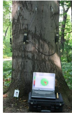
Figure 63 : Tomographe ArborSonic 3D ( http://www.fakopp.com/ ).
