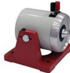
Figure 22 : Pot vibrant (Source Bruel & Kjaer, type LDS V201).
