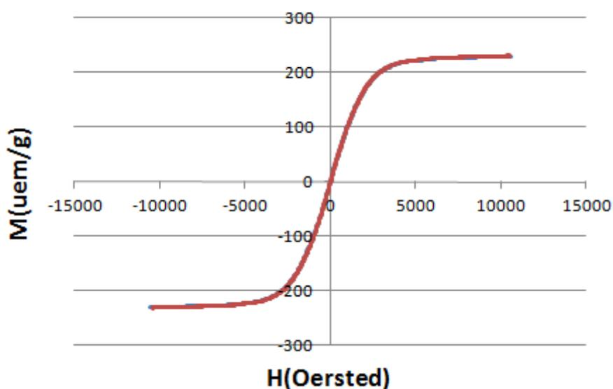
*Fig. 5-12 Magnetization curve of BASF particles (HQ grade)*
