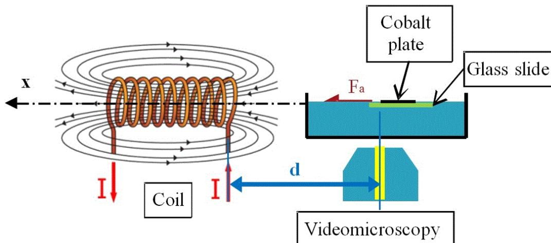
*Fig. 3-12: Simplified experimental setup, experience with the cobalt plate bonded to glass slide, on carbopol*
