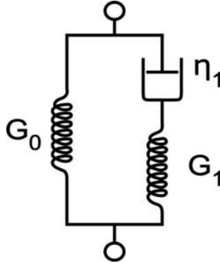
**Fig. 6-7: A schematic of the Zener Model**
