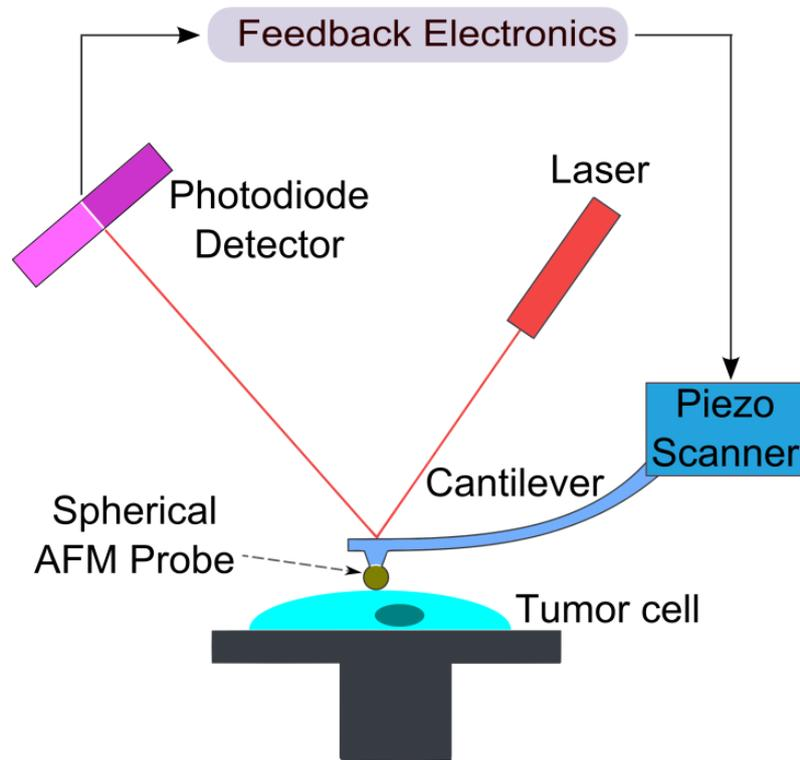
*Fig. 2-13: Block diagram of atomic force microscope*
