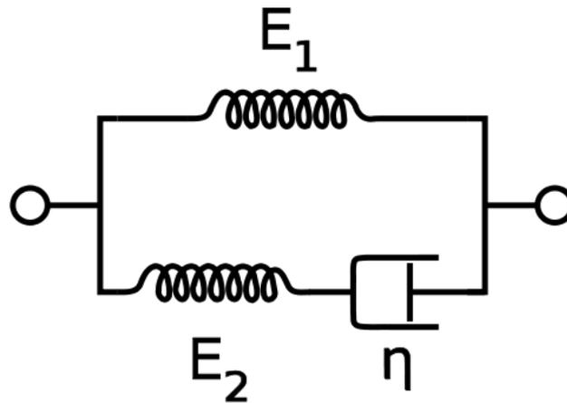
*Fig. 2-11 : Schematic representation of the Zener model*
