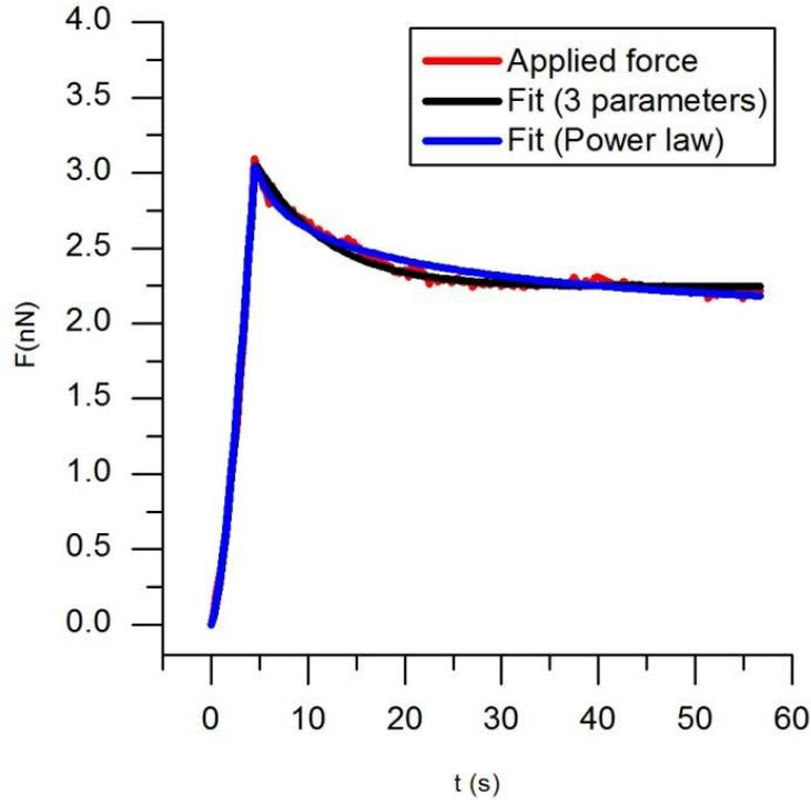
**Fig. 4-15: Applied force (in red) versus time during an indentation with a velocity:  $v=0.25\mu\text{m/s}$  and a maximum indentation depth:  $h_s=1.08\mu\text{m}$ . The blue triangles represent a fit with a power law for  $G(t)$  and the black circles a fit with a one branch Maxwell model**
