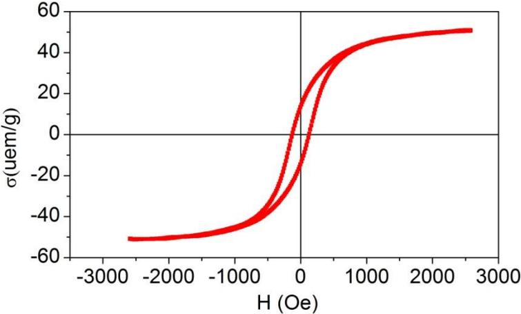
*Fig. 5-14: Magnetization curve of iron oxide particles*
