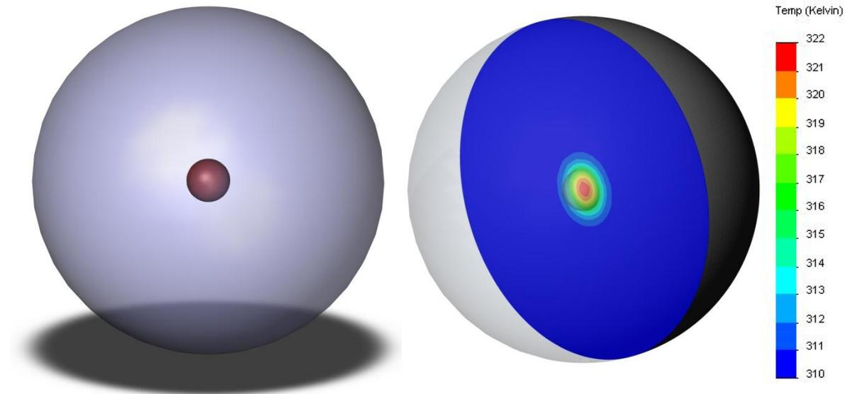
*Fig. 7-12: Simulation of hyperthermia in cancer treatment, the left figure represents a tumor of  $1\text{cm}^3$  in a spherical environment (diameter of 10cm) of water, the right figure is the result of simulation (Cross-sectional view) after 2mn*
