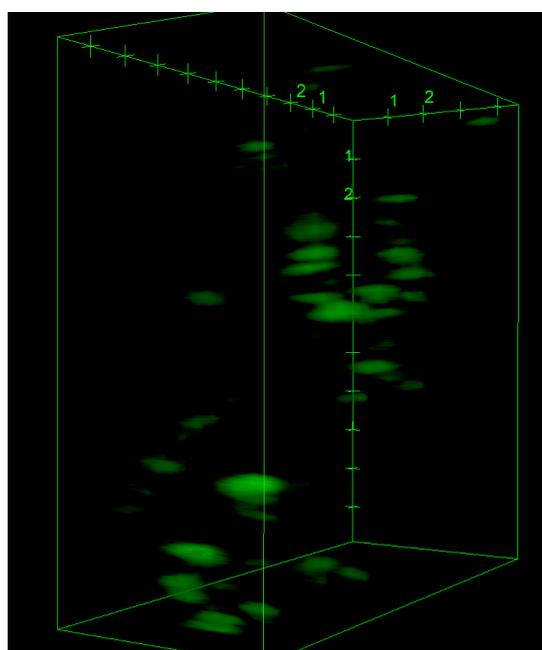
*Fig. 5-6: Confocal microscopy 3D-picture of Fe@Au-S-PEG<sub>5000</sub>-Fluorescein NPs in emission mode (green channel). The bounding box displays xyz coordinate system as well as units (scale in  $\mu m$ ).*
