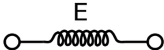
*Fig. 2-6 : Model of an elastic solid, a spring*
