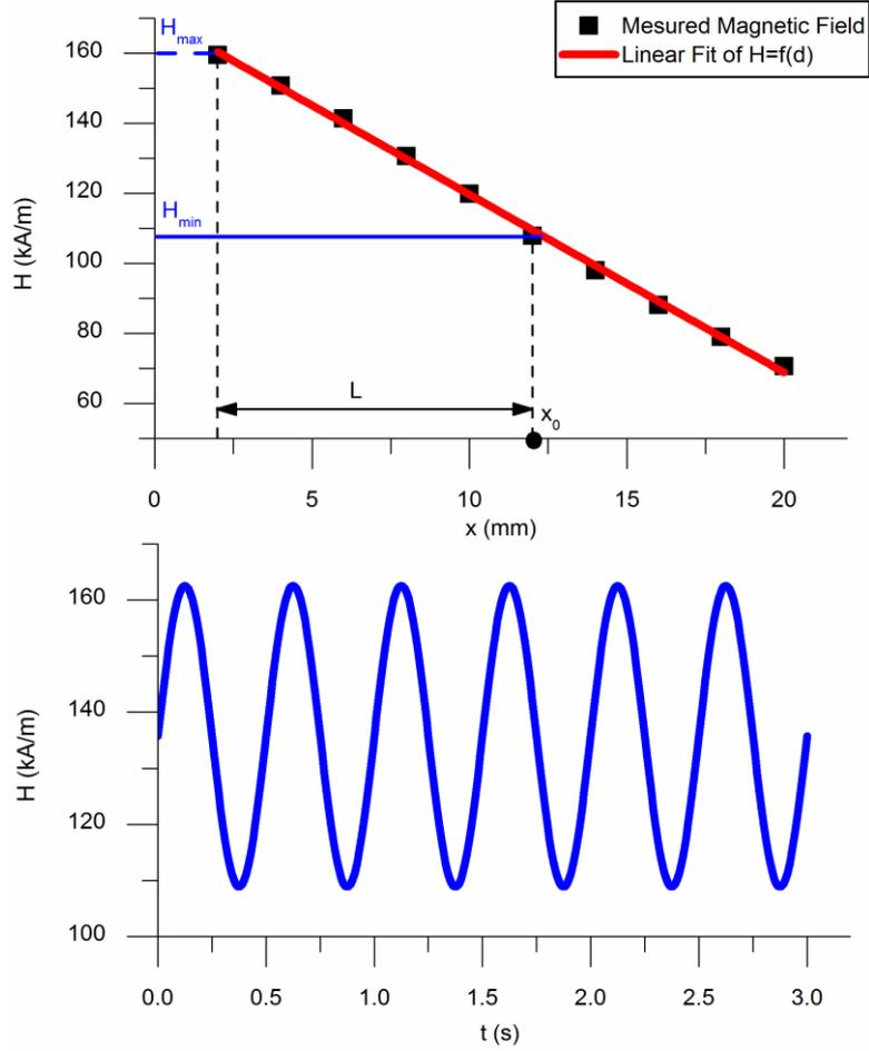
**Fig. 6-2: Upper graph: Measurement of magnetic field vs. distance between magnet and cells.
