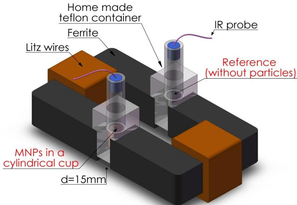
*Fig. 7-1 : Experimental setup for hyperthermia*
