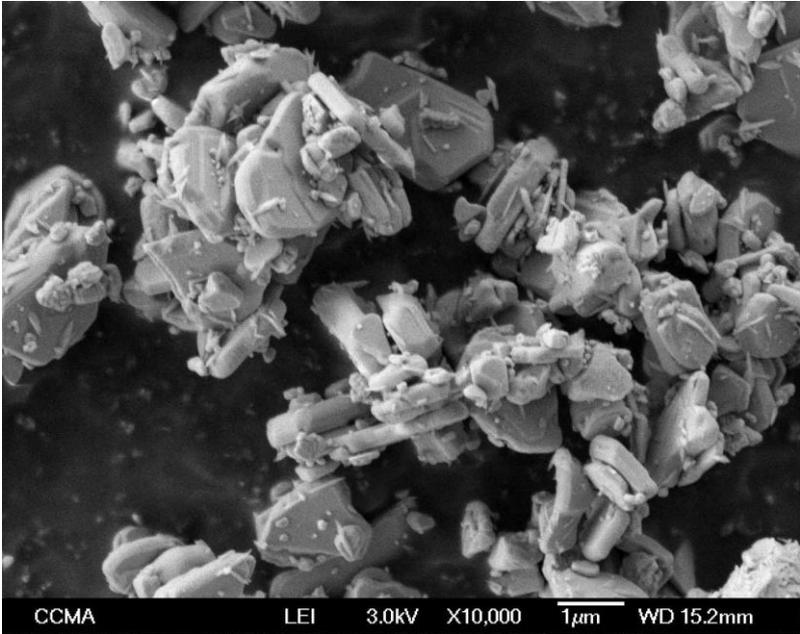
*Fig. 5-13: SEM view of iron oxide particles*
