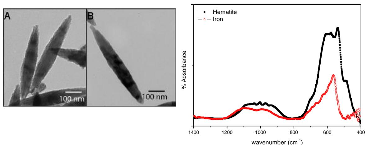
**Fig. 5-3: TEM pictures of (A)  $\alpha\text{-Fe}_2\text{O}_3$  and (B)  $\alpha\text{-Fe}(0)$  NPs. (C) IR spectrum of  $\alpha\text{-Fe}_2\text{O}_3$  (black line) and  $\alpha\text{-Fe}(0)$  NPs (red line)**
