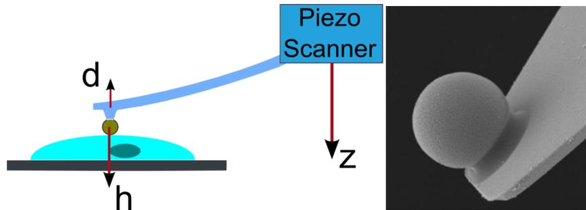
*Fig. 4-4: AFM spherical probe for rheological study*
