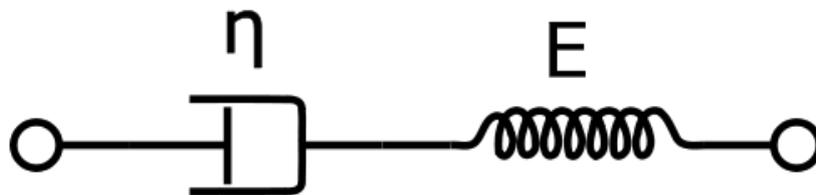
*Fig. 2-8 : Maxwell model, a dashpot and a spring in series*
