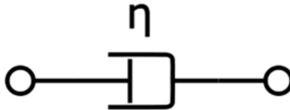
*Fig. 2-5 : Model of a Newtonian fluid, a dashpot*
