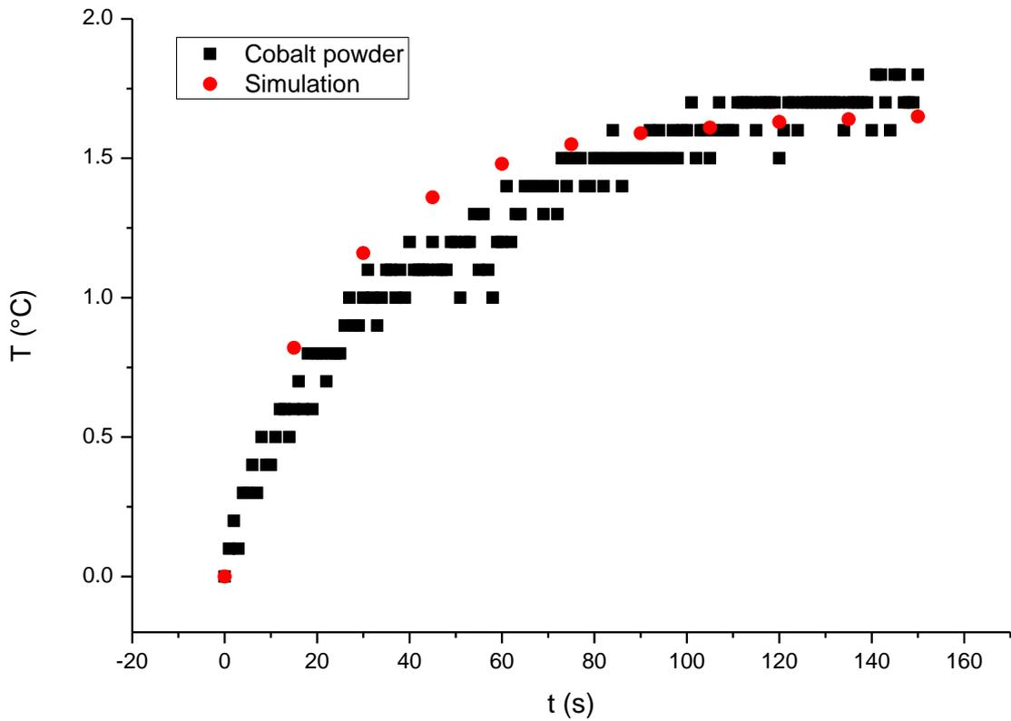
**Fig. 7-9: Increase of temperature versus time, the comparison of experimental and simulation result of cobalt powder, same condition as in Fig. 7-8**
