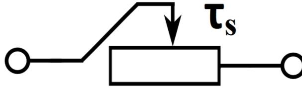
*Fig. 2-7 : Model of a yield stress, a switch*
