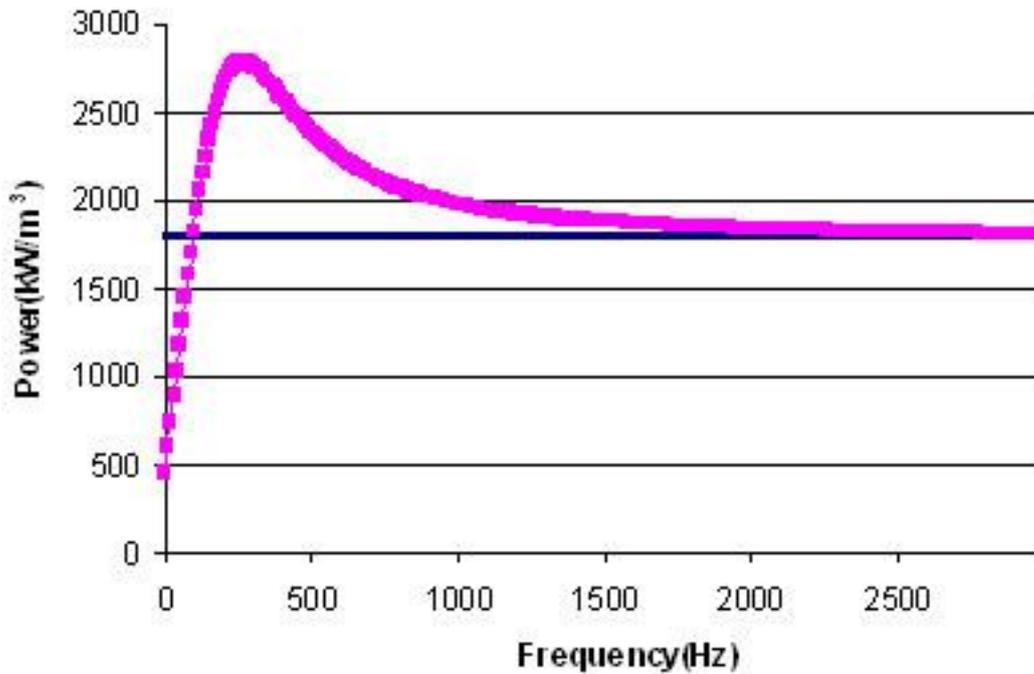
*Fig. 7-11. Power dissipated by rotation for  $\theta_0=30^\circ$   $H=12\text{kA/m}$   $M_r=250\text{kA/m}$   $\eta=10\text{Pa}\cdot\text{s}$  The blue line is the limit predicted by Eq.(7.15)*
