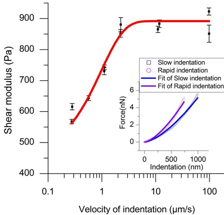
**Fig. 4-14: Young's modulus versus indentation velocity. In the insert: force versus indentation for two different velocities ( $v=100\mu\text{m/s}$  and  $100\text{nm/s}$ ) and their fit by Eq. (4.22)**
