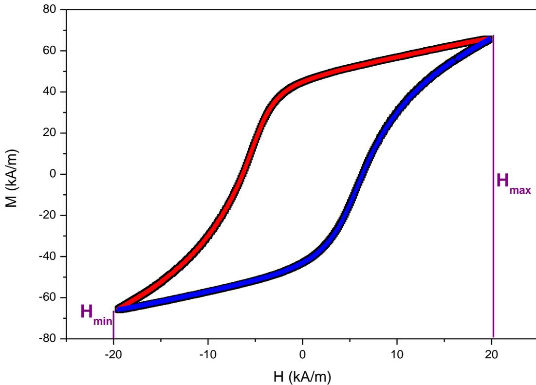
*Fig. 7-3: Hysteresis loop, the dissipated energy is the area under red line minus the area under blue line. Here for cobalt nanowires*
