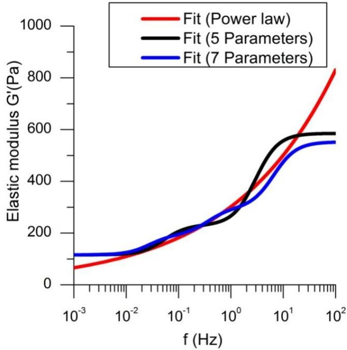
**Fig. 4-18 : Frequency dependence of the real part of the shear modulus:  $G'(\omega)$  deduced from the fit of  $G(t)$  by different models. Black line: power law model (Eq.(4.44)), redline: Maxwell model with two branches (Eq.(4.42)), Blue line: Maxwell Model with three branches**
