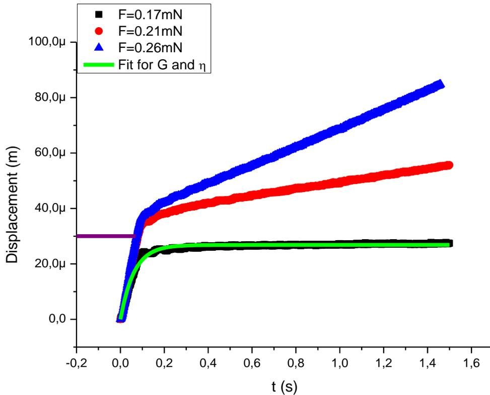
*Fig. 3-19: The displacement of the nickel fiber versus time*
