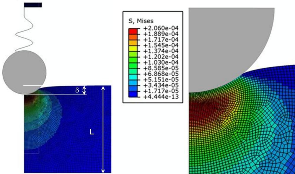
**Fig. 4-9: Calculation of the force with respect to the indentation in a viscoelastic medium with a spherical probe mounted on a spring using the software Abaqus**
