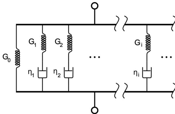
**Fig. 4-7: Schematic representation of the Generalized Maxwell model**
