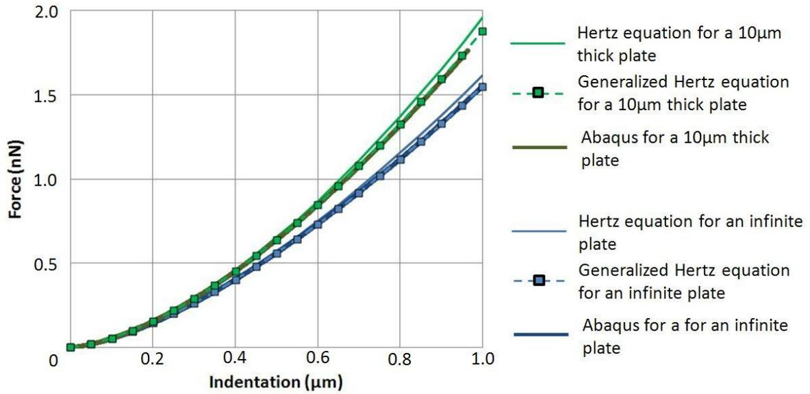
**Fig. 4-8: Calculation of the force with respect to the indentation using Abaqus, the Hertz model and the generalized Hertz model in the case of an infinite elastic plate and of a 10μm thickness plate**
