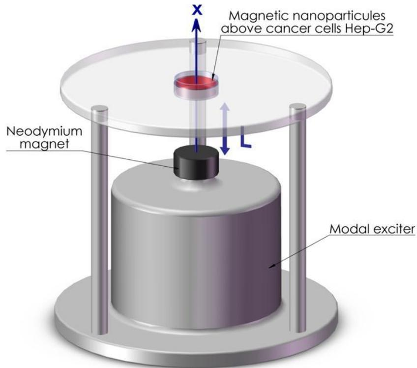
**Fig. 6-1: Experimental setup**
