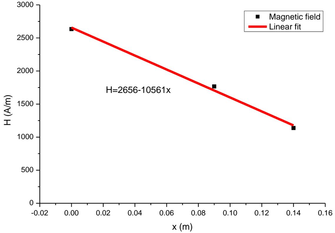
*Fig. 3-10 : Measurement of magnetic field gradient*
