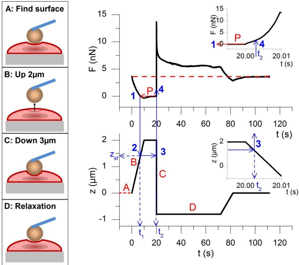
*Fig. 4-5: Left is an indentation cycle; right is the method for the determination of the contact point and of the force/indentation curve. Upper graph: experimental force versus time. Lower graph: motion of the cantilever head versus time*
