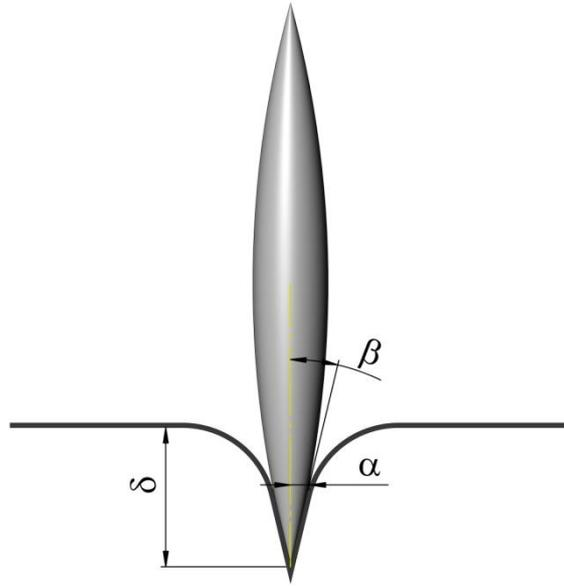
**Fig. 6-6: Conical particles**
