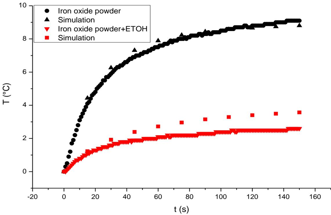
*Fig. 7-8: Temperature rise versus time, comparison of experimental and simulation results for iron oxide powder with and without ethanol, the conditions of experiment:  $f=5$  kHz,  $H=12$  kA/m*
