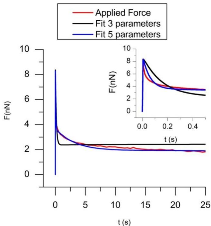
**Fig. 4-16 : Rapid indentation: applied force versus time during an indentation with a velocity:  $v=250\mu\text{m/s}$ . Red dots represent a fit with 3 parameters (the Zener model) for  $G(t)$  and the blue triangles a fit with 5 parameters (two Maxwell branches)**
