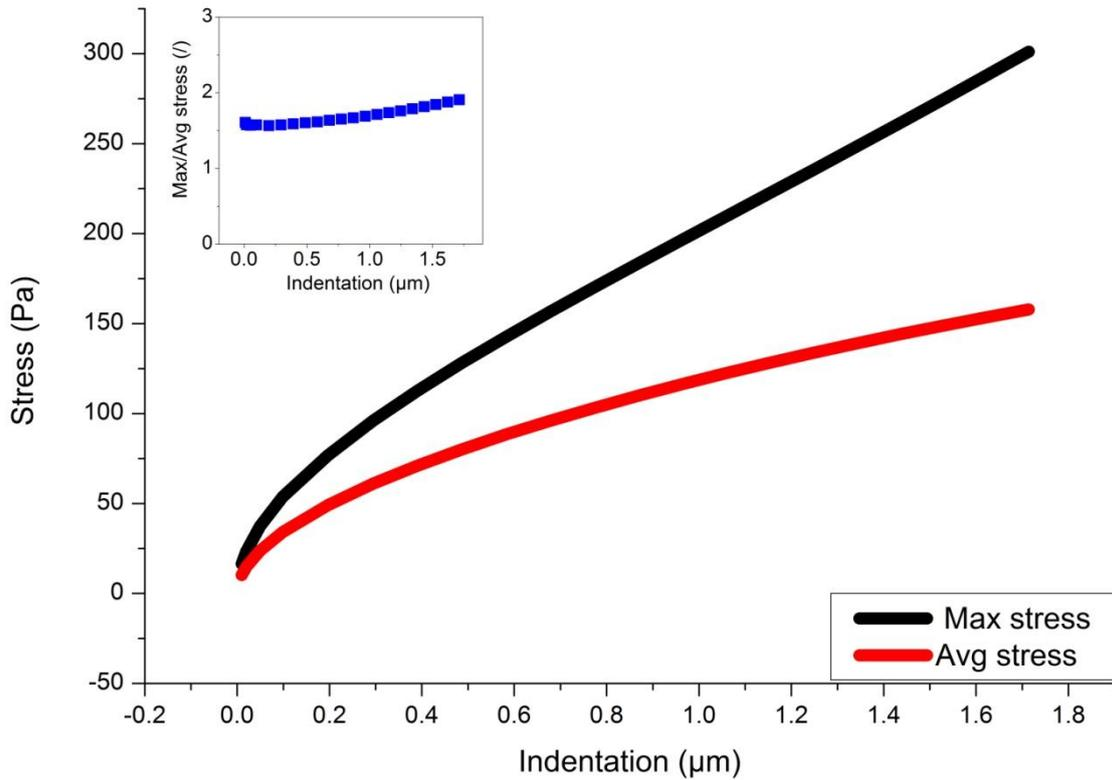
**Fig. 4-11: Maximum and average stress with respect to the indentation depth for a purely elastic medium; the diameter of the bead is  $5\mu\text{m}$  and the thickness of the layer is  $10\mu\text{m}$ ; the insert is the ratio of maximum stress to average stress**
