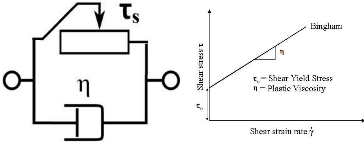
*Fig. 2-10 : Model of Bingham, a dashpot and a switch in parallel*
