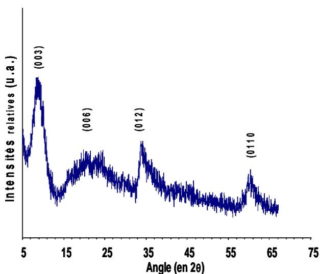
Figure IV-2 : Diffractogramme X de [Zn-Ni-Cr-SO<sub>4</sub>]
