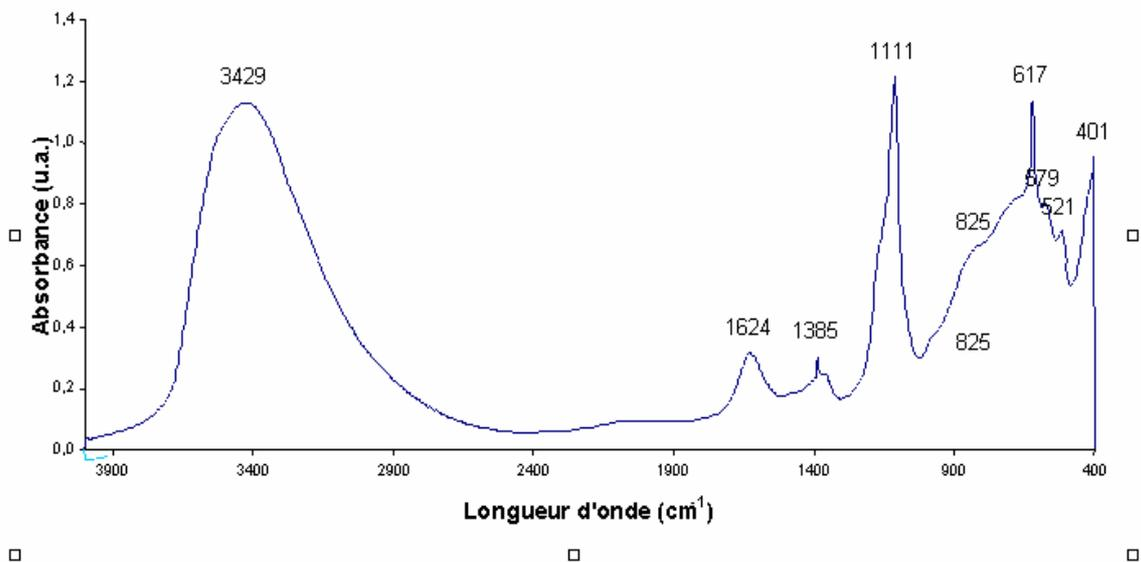
Figure IV-5 : Spectre infrarouge de [Zn-Ni-Al]
