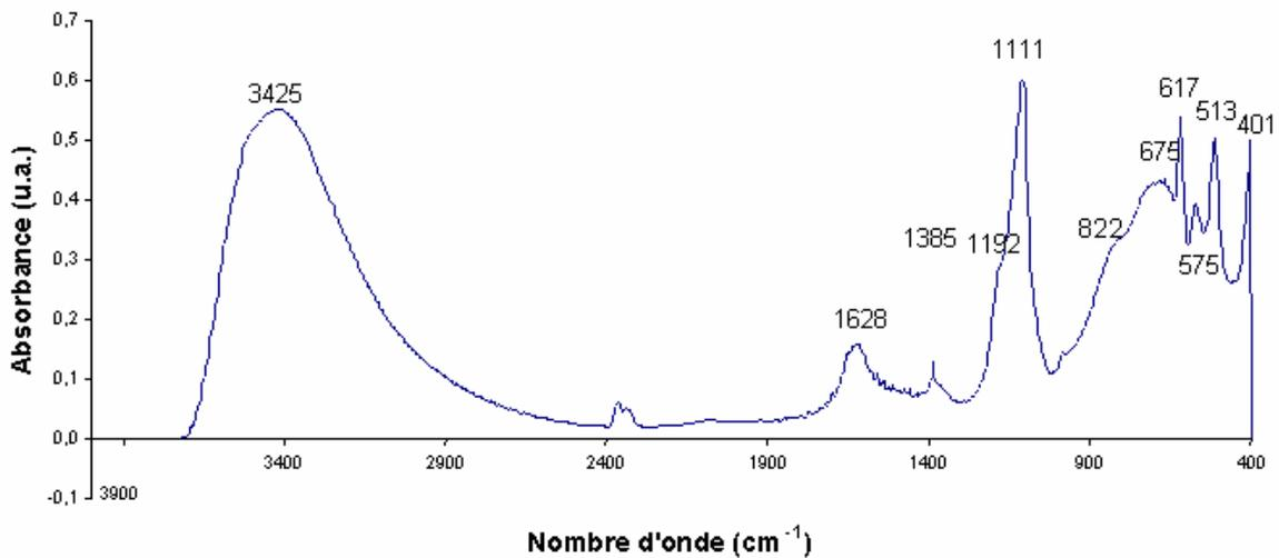
Figure IV-4 : Spectre infrarouge de [Zn-Ni-Cr]
