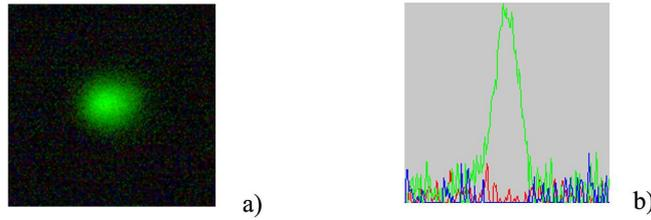
Figure 2.6: *Pump beam profile at the sample level, obtained with uEye CCD camera: a) beam shape; b) intensity profile.*
