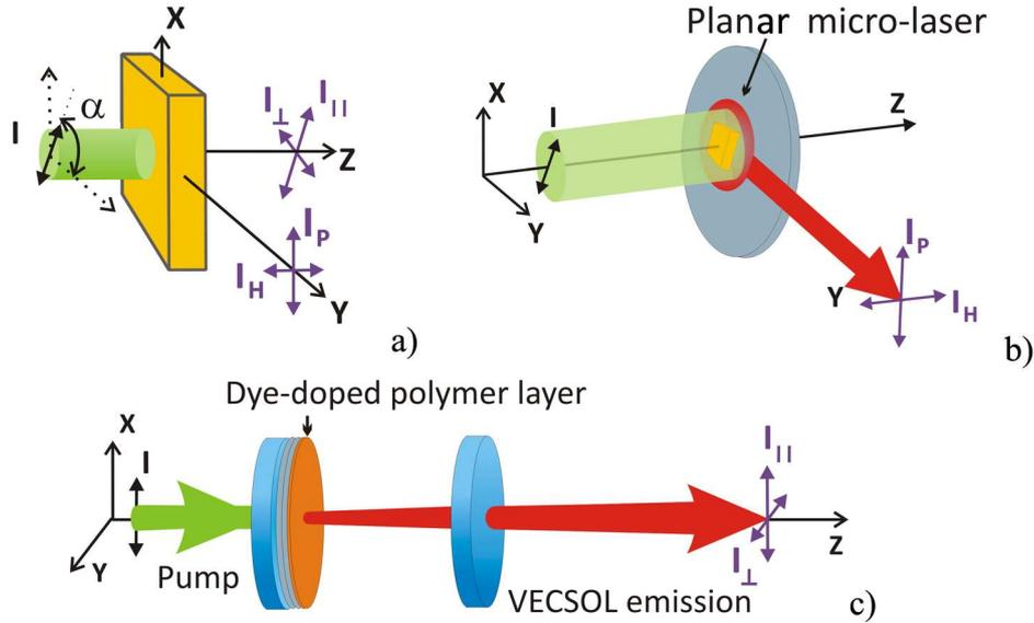
Figure 3.2: Description of different lasers emission configurations with respect to the pump beam polarization: a) general scheme for an arbitrary orientation (angle  $\alpha$ , defined with respect to the  $y$ -direction) of the linear polarization of the pump beam; b) planar micro-laser; c) VECSOL.
