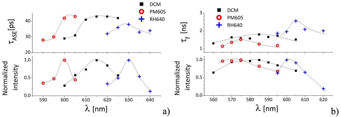
Figure 3.14: *Dynamics of stimulated (a) and spontaneous (b) emission in a layer of PMMA polymer doped with 5 wt% of DCM, RH640 or PM605. The upper frames show the process duration (error  $\pm 1.3$  ps for the ASE and  $\pm 60$  ps for the fluorescence), and the lower ones - the emission intensity for a series of wavelengths, normalized by the maximum intensity in the spectrum.*
