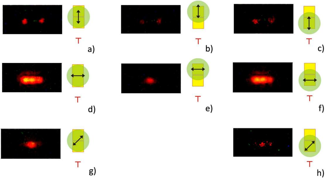
Figure I.4: *Slightly oblique observation of light emission from a system of closely-placed square-shaped micro-lasers (1  $\mu\text{m}$  gap) for various orientations of pumping beam polarization (with no sample illumination): a), b), c)  $\alpha = 0^\circ$ ; d), e), f)  $\alpha = 90^\circ$ ; g), h)  $\alpha = 45^\circ$ . Both symmetric (a, d, g) and non-symmetric pumping geometries applied (b, c, e, f, h). Pumping beam intensity was  $50 \text{ MWcm}^{-2}$ .*
