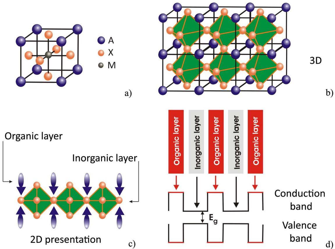
Figure J.1: *Perovskite materials: a) unit perovskite cell; b) 3D presentation of periodic repetition of the unit cells; c) 2D presentation of organic and inorganic layers; d) schematic organic-inorganic perovskite structure and a possible energy-level scheme.*
