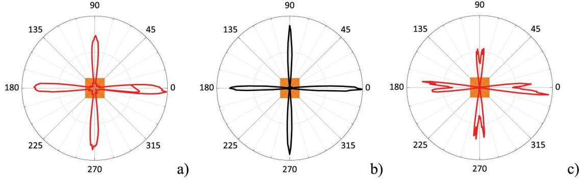
Figure 6.2: *Emission diagrams of a square micro-laser pumped with a  $20 \text{ MWcm}^{-2}$  circularly polarized light, corresponding to: a) total intensity of all peaks in the spectrum, b),c) maximum peak for each comb. The diagrams in (b) and (c) are plotted in different colors to depict different combs in emission spectra, consistently with the two combs spectrum on Fig.6.3.b.*
