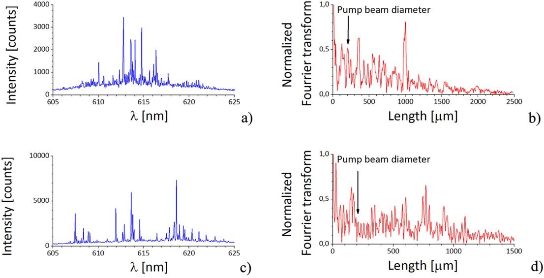
Figure H.1: *Random lasing in PMMA thin film doped with 5 wt% of DCM: a),c) emission spectra; b,d) their Fourier transform. Measurements were taken at two different pumping points (a,b) and (c,d), where the second point (c,d) was found in close vicinity of previously pumped region.*
