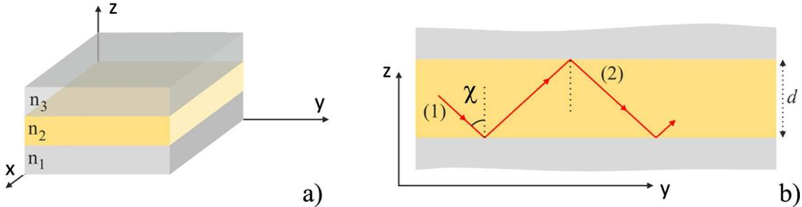
Figure 1.12: *Polymer layer viewed as a slab waveguide: a) schematic representation of our standard geometry as a 3-layer system (1 - substrate, 2 - guiding layer and 3 - surrounding) b) ray propagation inside the guiding layer.*
