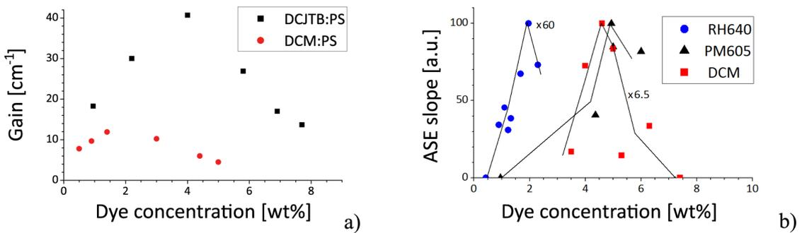
Figure 5.3: Amplification in PMMA-doped layer for the varied dye concentration: a) gain values from Ref. [129]; b) slope of ASE curves measured by the 2-D set-up for PMMA doped with RH640, PM605 or DCM.
