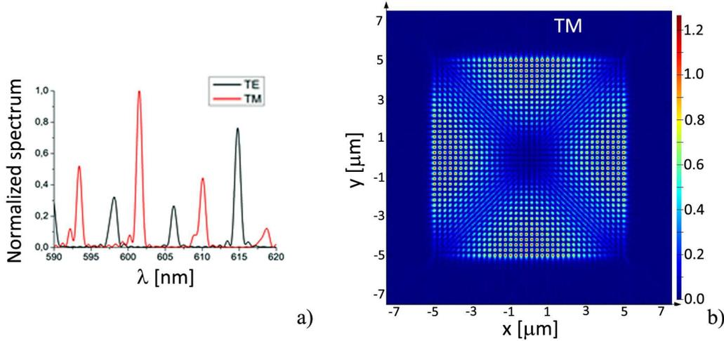
Figure 6.6: *FDTD simulations on a  $10 \mu\text{m}$  side square micro-laser: a) calculated spectrum in the spectral region used for experimental observation; b) mode pattern of a TM-polarized wave at  $593.5 \text{ nm}$ .*
