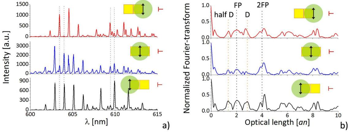
Figure I.6: *Emission of the system of two closely placed micro-lasers (1  $\mu\text{m}$  gap) with excitation geometry varied (indicated by the scheme next to each plot): a) emission spectra; b) normalized Fourier-transform (lengths of periodic orbits are indicated with FP and D: Fabry-Perot  $FP = 2an$ ; diamond  $D = 2\sqrt{2}an$ ). Excitation was made with the intensity of  $38.5 \text{ MWcm}^{-2}$  with polarization orthogonal to the emission direction ( $\alpha = 90^\circ$ ).*
