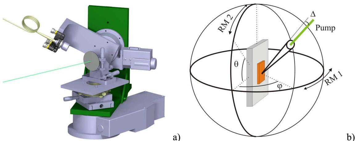
Figure 2.7: 3-D detection set-up a) overall scheme; b) detection geometry (the rotating mounts motion directions are shown by arrows RM 1, 2, the angle  $\Delta$  shows a dark region due to the finite physical dimensions of the system).
