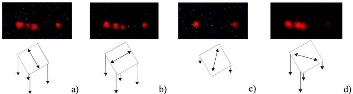
Figure 6.11: Slightly tilted observation off symmetry of light emission from square-shaped micro-laser for various orientations of the pump beam polarizations: a)  $\alpha = 0^\circ$ , b)  $\alpha = 90^\circ$ , c)  $\alpha = 45^\circ$ , d)  $\alpha = 135^\circ$ .
