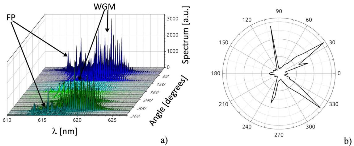
Figure G.2: *Emission properties of 70  $\mu\text{m}$  radius MD7-based concave kite ( $\delta = 0.5$ ): a) emission spectra; b) emission diagram from the full spectrum.*
