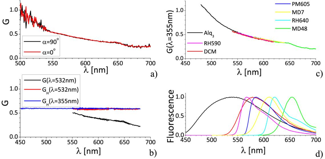
Figure D.2: Set-up-induced depolarization factors  $G$  and  $G_H$ : a)  $G$  value for RH590 solution under pumping with different  $\alpha$ , b)  $G_H$  values under 532 and 355 nm pumping and  $G$  (532 nm); c) illustration of the  $G$  parameter on the example of  $G$  (355 nm) as from the peak emission of the corresponding fluorescence spectra (d).
