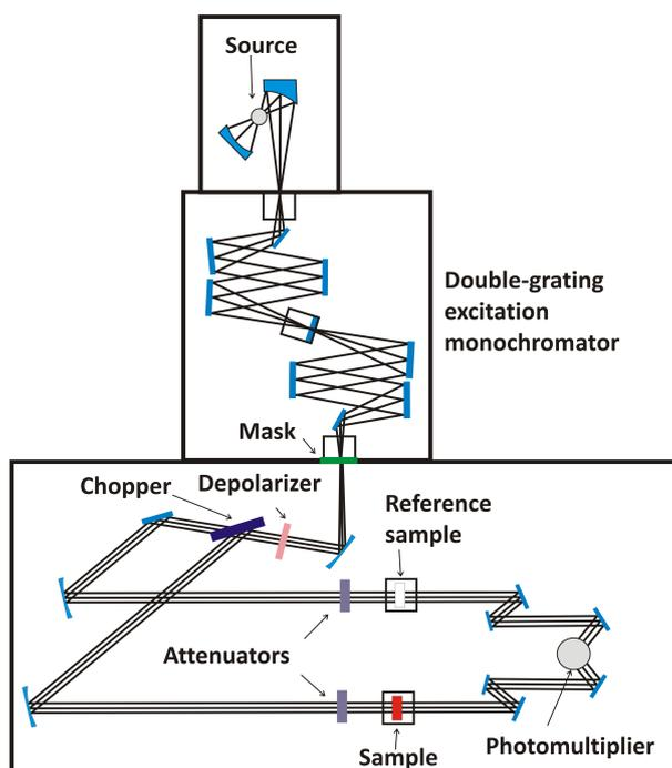
Figure 2.9: *Scheme of the Lambda 950 spectrometer.*
