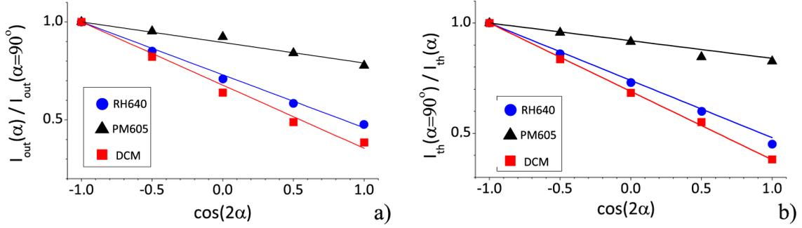
Figure 5.11: Influence of the polarization on relative values of: a) ASE, b) threshold for a 165  $\mu\text{m}$  ribbon micro-laser. Experimental data on all three dyes is plotted by points while solid lines follow Eq.(5.25) with  $\rho$  taken from experimental data (averaged over  $\alpha$  to reduce the error)
