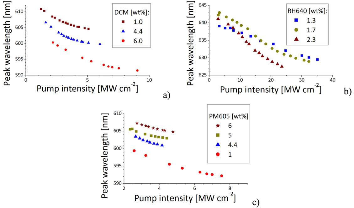
Figure 5.4: Spectral shift of the ASE peak with the increase of pump power at various concentrations of: a) DCM, b) RH640, c) PM605.
