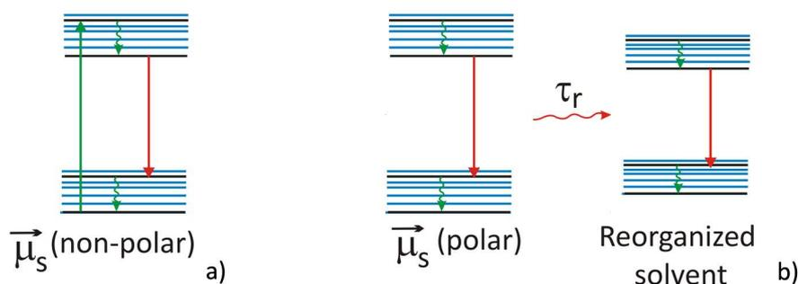
Figure 1.9: Mechanism of the solvatochromic influence on the fluorescence properties of dyes: a) Perrin-Jablonski diagram for a dye in a solvent with low polarity, b) Perrin-Jablonski diagram for a dye in a polar solvent.
