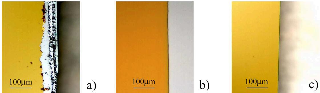
Figure A.3: *Optical microscope photographs of edge cleaving methods: a) polymer side cut b) plasma etching (layer covered by a glass plate), c) wafer side cut.*
