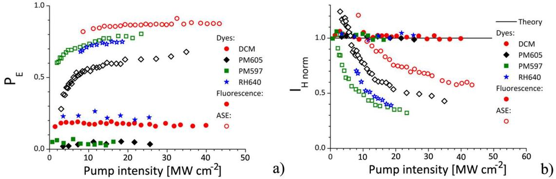
Figure 3.15: Change of the anisotropy when going from guided fluorescence to ASE (fluorescence generated by CW pumping on a PMMA-doped layer deposited on a Si/SiO<sub>2</sub> wafer): a)  $P_E$ , b)  $I_H$ .
