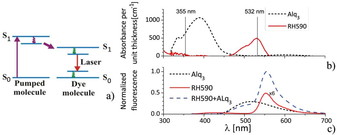
Figure 4.1: *Excitation of a dye via energy transfer: a) excitation scheme; b) absorbance of RH590, Alq<sub>3</sub> (measured with spectrophotometer, Sub-section 2.3.1), c) fluorescence of RH590, Alq<sub>3</sub> and RH590-Alq<sub>3</sub> mixture taken at equal molar quantities (measured with spectrofluorimeter, Sub-section 2.3.3). The absorption and fluorescence measurements were performed with dye-doped thin polymer films deposited on glass slide.*
