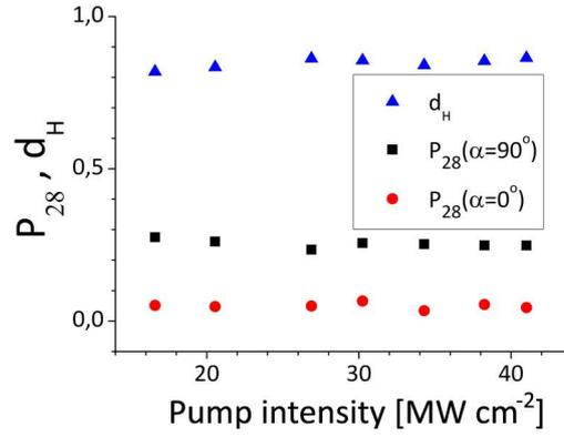
Figure 3.11: *Experimental plots for the polarization degree ( $P$ ) and  $d_H$  parameter, obtained with 3-D detection set-up for the emission at  $\gamma = 28.1^\circ$  ( $\gamma_0 = 45^\circ$ , Fig.3.10.a) with 5 wt% DCM in PMMA (spin-coated layer) under pulsed pumping. Deduced averaged values are provided in Tab.3.3.*
