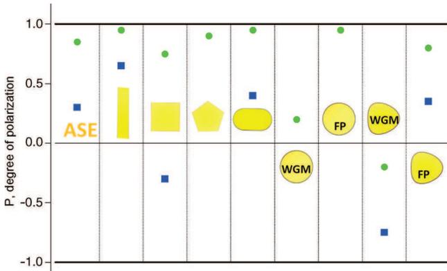
FIG. 8. (Color online) Degree of polarization  $P$  in connection with the resonator shape for a DCM-PMMA layer pumped at 532 nm (green disks) and a MD7-PMMA layer pumped at 355 nm (blue squares). (From left to right) ASE, Fabry-Perot, square (diamond modes), pentagon (inscribed pentagon), stadium (WGM), disk (WGM), disk (Fabry-Perot modes), kite (WGM), and kite (Fabry-Perot modes).
