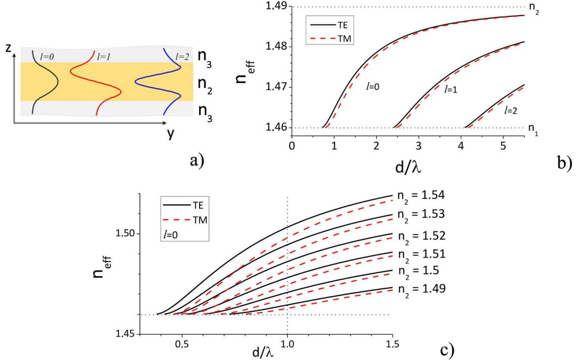
Figure 1.13: Mode structure in traversal direction of a planar waveguide with symmetric environment (a), effective refractive index of a guiding layer as a function of  $d/\lambda$  for the non-doped PMMA (b) and for several values of refractive index slightly modified as result of doping the PMMA with a dye (c).
