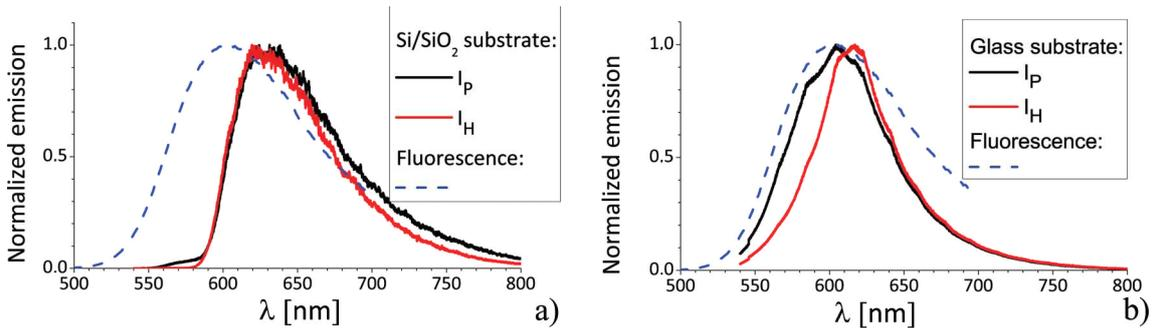
Figure 3.9: Guided wave fluorescence spectra, measured in the edge emission configuration in a thin PMMA film doped by 5% of the PM605 dye deposited on: a) a Si wafer covered by  $2 \mu\text{m}$  of silica, b) a glass slide. Comparison is made with the fluorescence spectrum measured in an oblique (e. g. “non-edge”) emission direction in a film deposited on a Si wafer, whereby guiding is not possible. The excitation wavelength is 532 nm.
