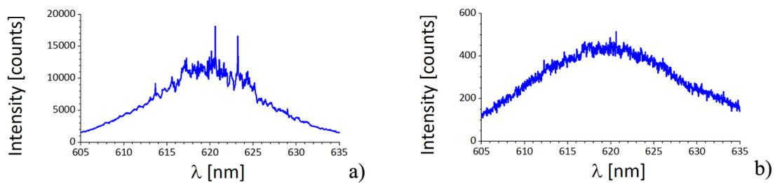
Figure H.7: *Polarized emission spectrum (integrated over 3 s): a) TE polarization (in the sample plane); b) TM polarization - ASE only (orthogonal to the sample plane). Measurement performed in the PMMA thin film doped with 5 wt% of DCM.*
