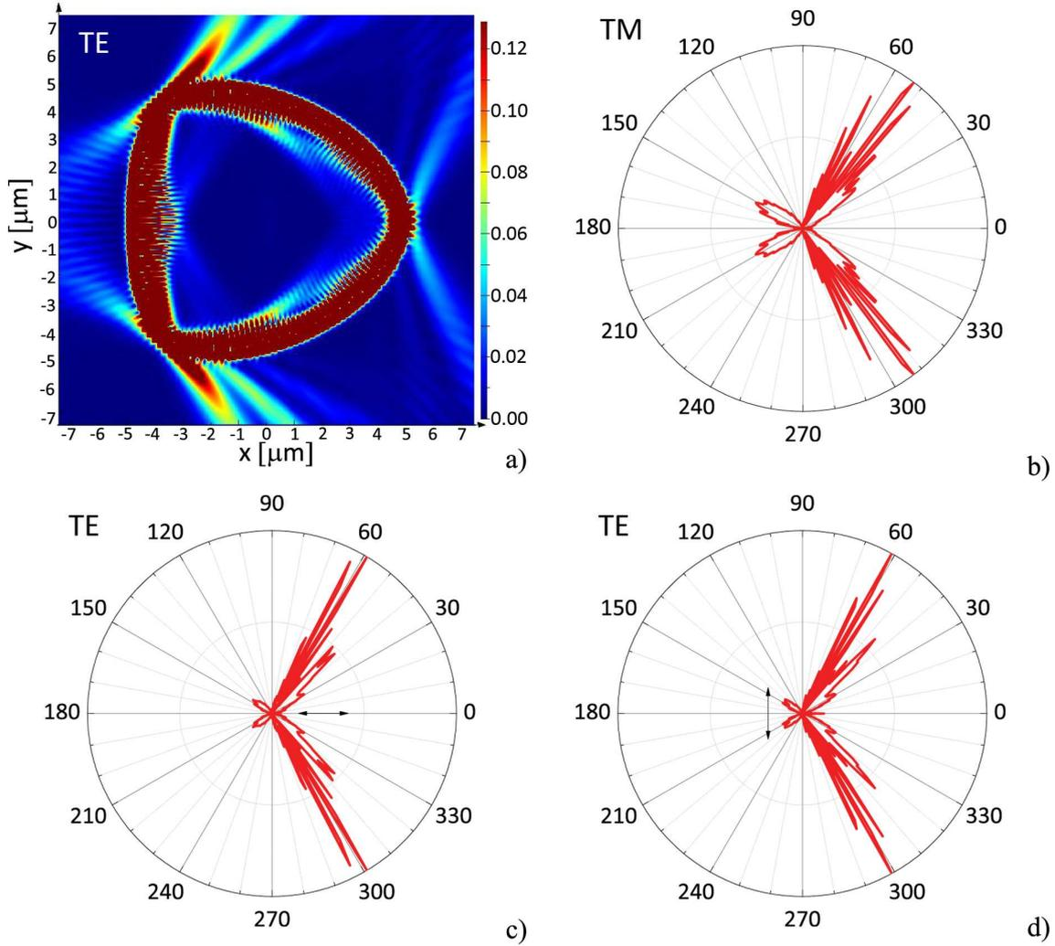
Figure 6.25: FDTD simulations for a  $r = 5 \mu\text{m}$  kite with  $\delta = 0.165$  : a) zoom of a TE mode map (606.5 nm); angular emission diagrams for b) TM (604.3 nm); c) TE (606.5 nm,  $\alpha = 0^\circ$ ) d) TE (606.5 nm,  $\alpha = 90^\circ$ ).
