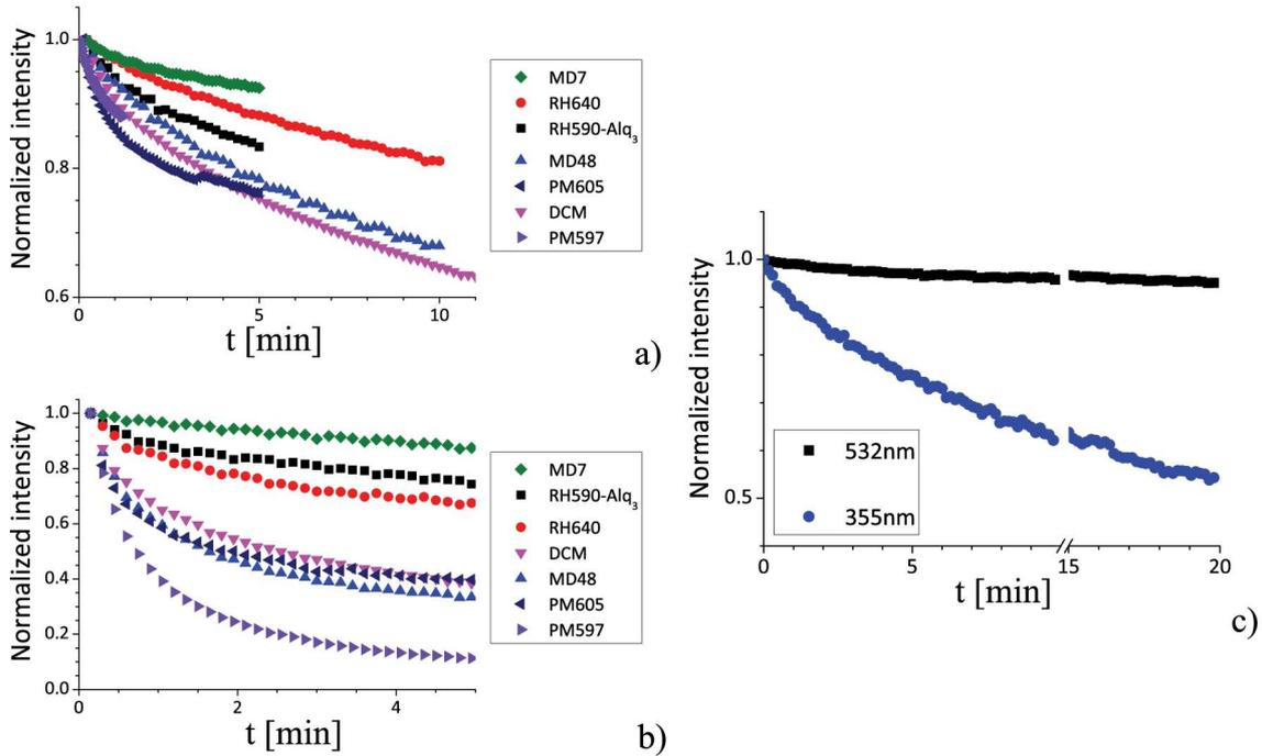
Figure 4.10: *Intensity decay of ASE emission of dye-doped polymer layers under pulsed pumping (500 ps, 10 Hz) at wavelength of: a) 532 nm (17  $\text{MW cm}^{-2}$  for RH640 and MD48); b) 355 nm (pump intensity about 50  $\text{MW cm}^{-2}$ ); c) comparison of MD7 dye degradation under pumping at 532 (50  $\text{MW cm}^{-2}$ ) and 355 nm (about 50  $\text{MW cm}^{-2}$ ).*
