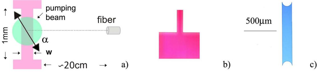
Figure 5.5: *Experimental study of Fabry-Perot resonators: (a) pumping configuration ( $\alpha$  stands for the angular orientation of the linear pumping beam polarization with respect to the observation direction); optical microscope photos of  $165\mu\text{m}$  PMMA-PM605 ribbon micro-laser made by e-beam (part of it only, as the overall cavity size is too big to enter the frame), another Fabry-Perot type cavity made from PMMA-MD48 by photo-lithography (c).*
