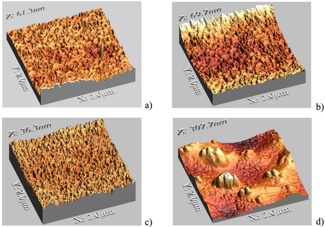
Figure J.5: Atomic force microscope images on PEPI film roughness. The left column corresponds to surface treatment with  $O_2$  prior to PEPI deposition, while the right - with KOH. Following substrates were used for PEPI deposition: glass (a, b) and PMMA deposited on the glass (c, d).
