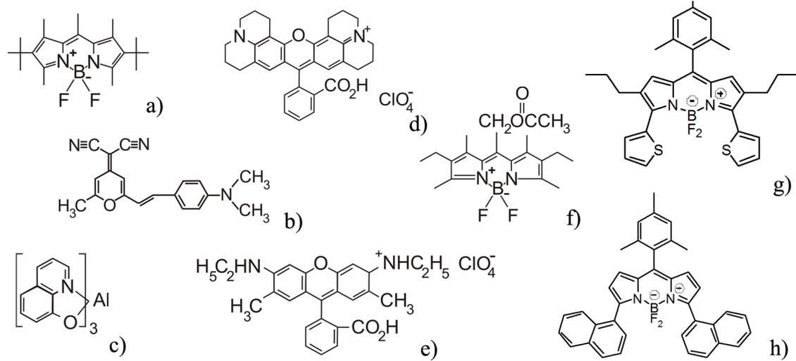
Figure C.1: The molecular structure of the dyes and fluorophores used in this work: a) PM597; b) DCM; c) Alq<sub>3</sub>; d) RH640; e) RH590; f) PM605; g) MD48; h) MD7.
