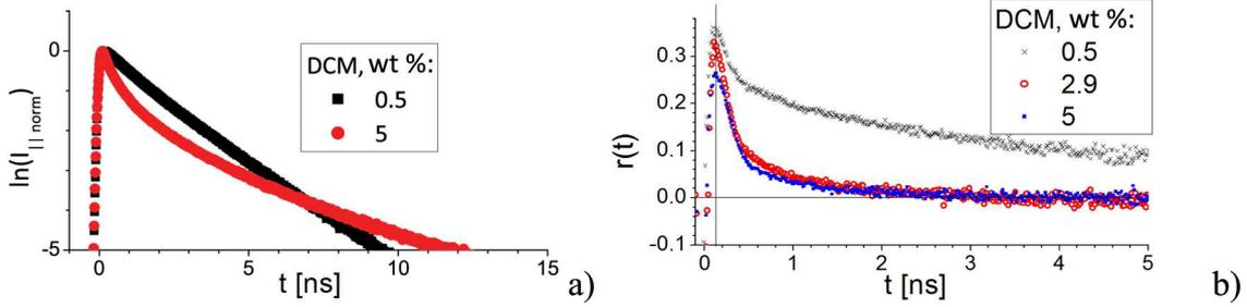
Figure 3.8: Influence of FRETs on the fluorescence emission on the example of DCM in PMMA: a) mono- and bi-exponential decays of the  $I_{\parallel}$  intensity component respectively for 0.5 and 5 wt% concentration, b) reduction of anisotropy with the concentration increase.
