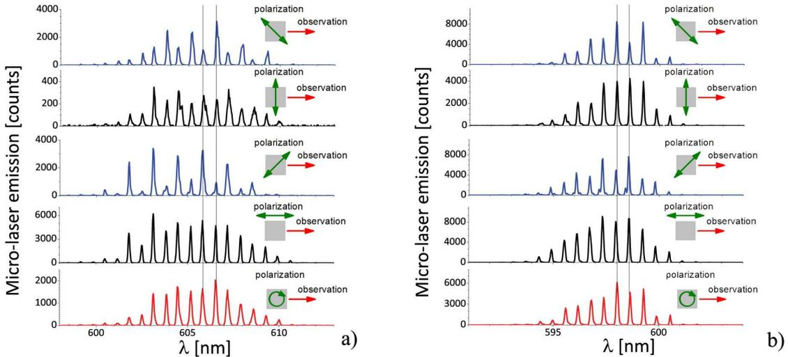
Figure 6.4: *Effect of pump polarization on the spectra of a square micro-laser (120  $\mu\text{m}$  side): a) DCM-based square under  $54 \text{ MWcm}^{-2}$  pumping, b) PM605-based square under  $7 \text{ MWcm}^{-2}$ .*
