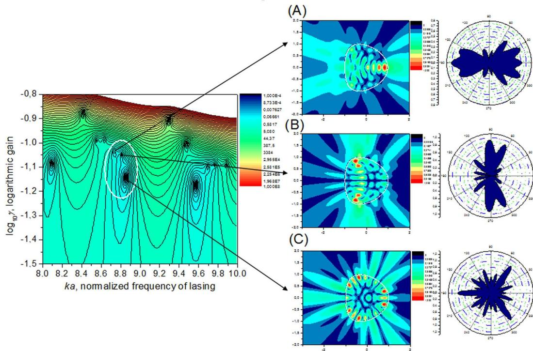
Figure 6.21: *LEP simulations: (left) map of the eigenvalues (dark colored regions) in gain ( $\gamma$  - imaginary part of refractive index) and  $ka$  (cavity size) coordinates, (right) - field maps and emission diagrams for three adjacent eigenvalues from the map on the left. Simulation parameters:  $\delta = 0.165$ , refractive index  $n=1.5$ , discretization by  $N=50$  quadratures.*
