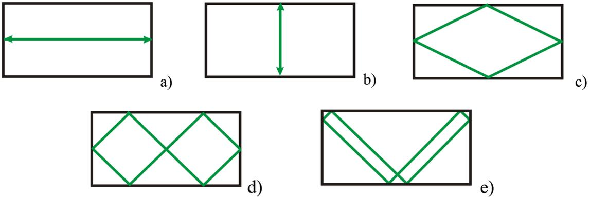
Figure 6.14: *Scheme of periodic orbits in a 2:1 rectangle resonator: Fabry-Perot (a,b), diamond (c), symmetric double diamond (d), general in-family double diamond (e) orbit. Only Fabry-Perot orbits depicted in (a) observed experimentally.*
