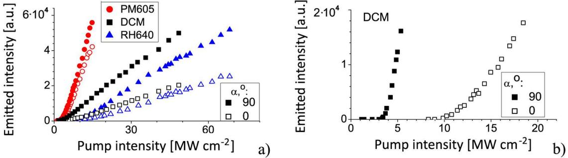
Figure 5.10: Influence of the pump beam polarization angle  $\alpha$  on the emitted versus pump intensity in the case of a) ASE, b) a  $165 \mu\text{m}$  DCM ribbon micro-laser.
