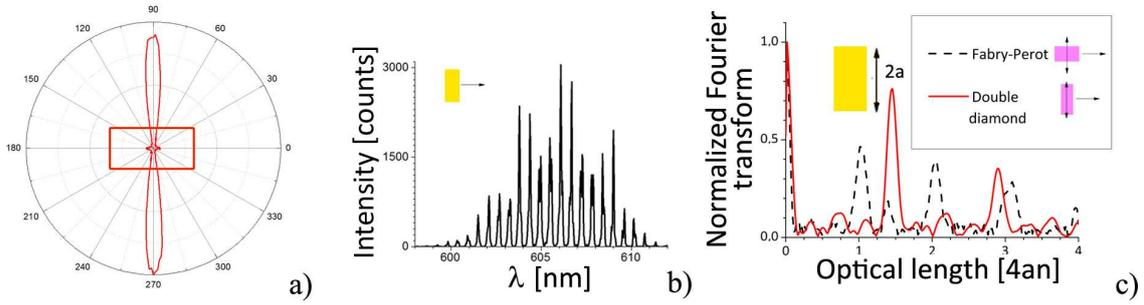
Figure 6.17: *Emission diagram (a) and spectrum (b) of the double diamond mode from a rectangle micro-laser (5 wt% DCM, pumped by a circularly polarized beam). Fourier transform (c) of the spectra, obtained under linear pumping beam polarization ( $\alpha = 90^\circ$ ) along long (Fabry-Perot orbit) and short (double diamond orbit) cavity sides.*
