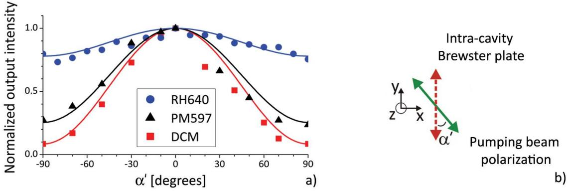
Figure 3.16: *Polarization properties of the VEC SOL: a) output intensity of VEC SOL lasers under a fixed pumping power at varying angles for pumping beam polarization with respect to the orientation of an intra-cavity Brewster plate; b) scheme on respective orientation of the pumping beam polarization and the orientation of an intra-cavity Brewster plate.*
