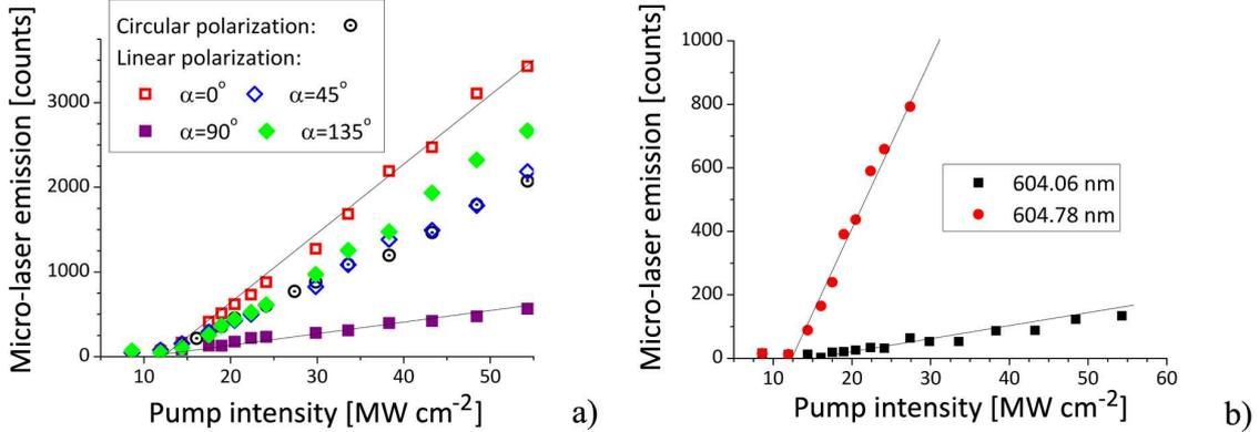
Figure 6.5: *Thresholds of square micro-laser emission in terms of pumping level: a) influence of pump beam polarization (threshold determined by the maximum peak), b) thresholds of two combs at  $\alpha = 45^\circ$  ( $11.2 \pm 0.3$  and  $12.6 \pm 0.3 \text{ MW cm}^{-2}$ ). Measurements performed with a  $120 \mu\text{m}$  side square made of PMMA-DCM (sample LPN7)*
