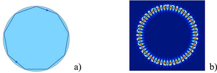
Figure 6.19: *Whispering gallery mode in a disk: a) schematic geometrical optics representation of the orbit propagation subject to periodic total internal reflections at the cavity border; b) simulated WGM field pattern.*
