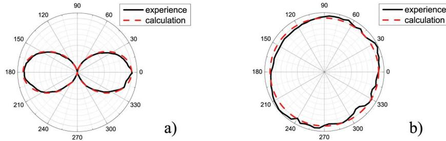
Figure 2.5: *Pump beam polarization state (a - linear, b - circular), presented as the normalized beam intensity just after W2 (a) or W3 (b) measured through a polariser (Polaroid film) by the photodiode (532nm pump wavelength). The angle plot on the diagrams corresponds to the angle between the polarizer and wave plate axes. The theoretical curves expected for polarizer transmission are shown by a red dashed line.*
