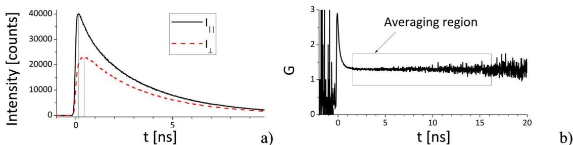
Figure D.1: *set-up-induced depolarization factor  $G$  and delay between polarized components, measured in a reference experiment with RH640 in anisole solvent: a) registered polarized components  $I_{\parallel}$  and  $I_{\perp}$  (as it is seen, the maximum of  $I_{\perp}$  is delayed with respect to  $I_{\parallel}$ ); b) the definition of  $G$  factor (delay between polarized components is taken into account).*
