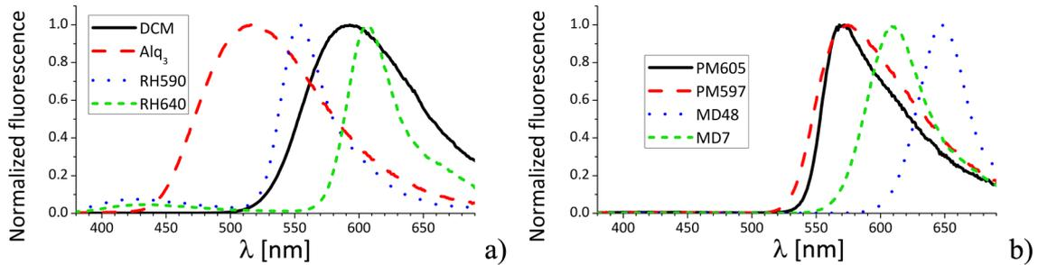
Figure 1.4: *Fluorescence spectra of thin PMMA layers (about 600nm), doped by various dyes: a) DCM, Alq<sub>3</sub>, RH590, RH640; b) Bodipy-family dyes: PM597, PM605, MD7, MD48.*
