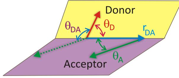
Figure 1.7: On  $\kappa^2$  calculations:  $\theta_{DA}$  is the angle between the emission dipole of the donor and the absorption dipole of the acceptor,  $\theta_D$  and  $\theta_A$  are the angles between these moments and the vector  $r_{DA}$  joining the donor and the acceptor.
