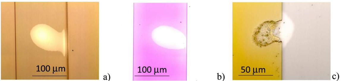
Figure 4.9: *Degradation of dye and polymer in ASE and lasing regimes on the example of a ribbon Fabry-Perot micro-laser made of 5 wt% of: a) RH590-Alq<sub>3</sub>, b) PM605, c) DCM. Pump intensity about  $70 \text{ MW cm}^{-2}$*
