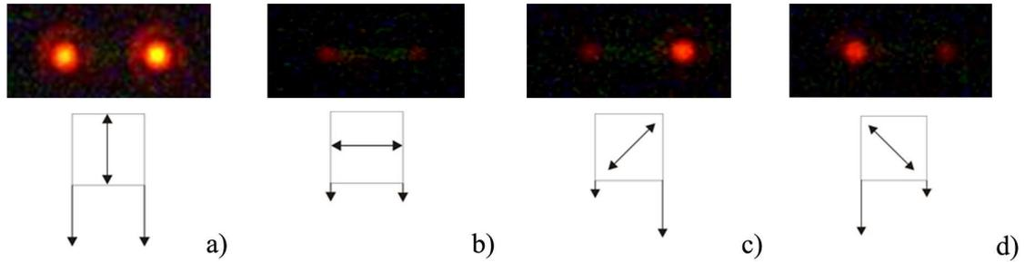
Figure 6.10: Slightly oblique observation of light emission from square-shaped micro-laser for various orientations of pumping beam polarizations (with no sample illumination): a)  $\alpha = 0^\circ$ , b)  $\alpha = 90^\circ$ , c)  $\alpha = 45^\circ$ , d)  $\alpha = 135^\circ$ .
