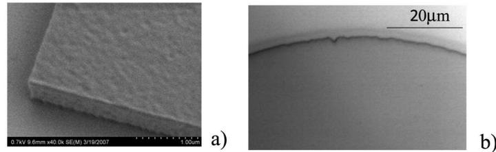
Figure 2.3: *E-beam lithography (a) versus photo-lithography (b).*
