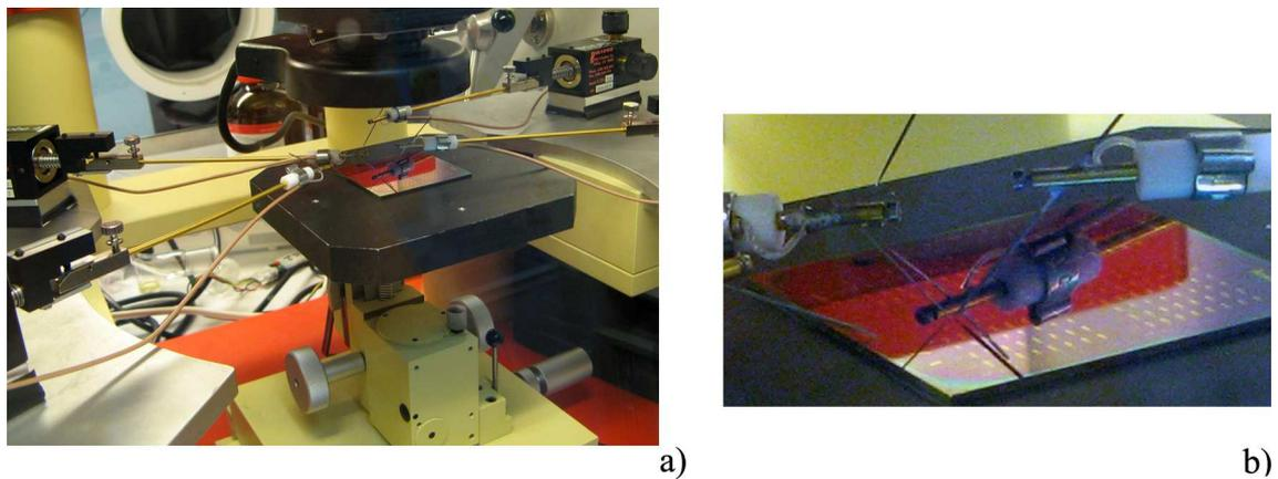
Figure J.7: *Photographs on the set-up utilized for the measurement of current-voltage characteristics of transistor: a) needle-contact micro-positioning system; b) zoom to the sample area.*
