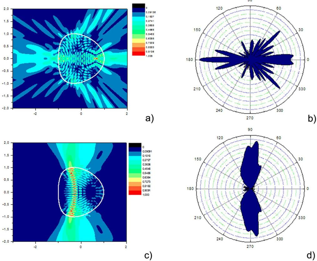
Figure 6.22: LEP map fields (a,c) and emission diagrams (b,d) for a kite with  $\delta = 0.165$ , and with  $(ka; \gamma) = (23.37; 3.54 \cdot 10^{-2})$  (a,b) and  $(23.49; 3.46 \cdot 10^{-2})$  (c,d). Refractive index  $n=1.5$ , discretization over a set of  $N=100$  points.
