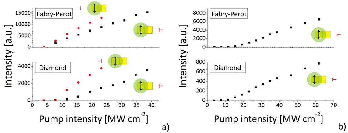
Figure I.8: *Lasing thresholds curves of Fabry-Perot and diamond modes in a system of two closely placed square micro-lasers for various gap sizes: a) 0.2  $\mu\text{m}$ ; b) 1  $\mu\text{m}$ . Excitation geometry is indicated by the scheme next to each plot.*
