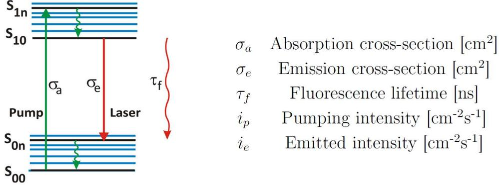
Figure 1.11: *Dye molecule as a 4-level lasing system.*
