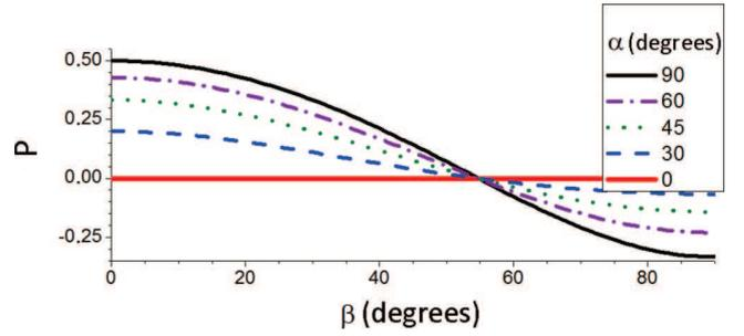
FIG. 4. (Color online) Degree of polarization  $P_{\text{in plane}}$  versus the angle  $\beta$  between the absorption and emission dipoles, following expression (2). For  $\alpha = \pi/2$ ,  $P_{\text{in plane}} = P_{\text{VECSOL}}$ .
