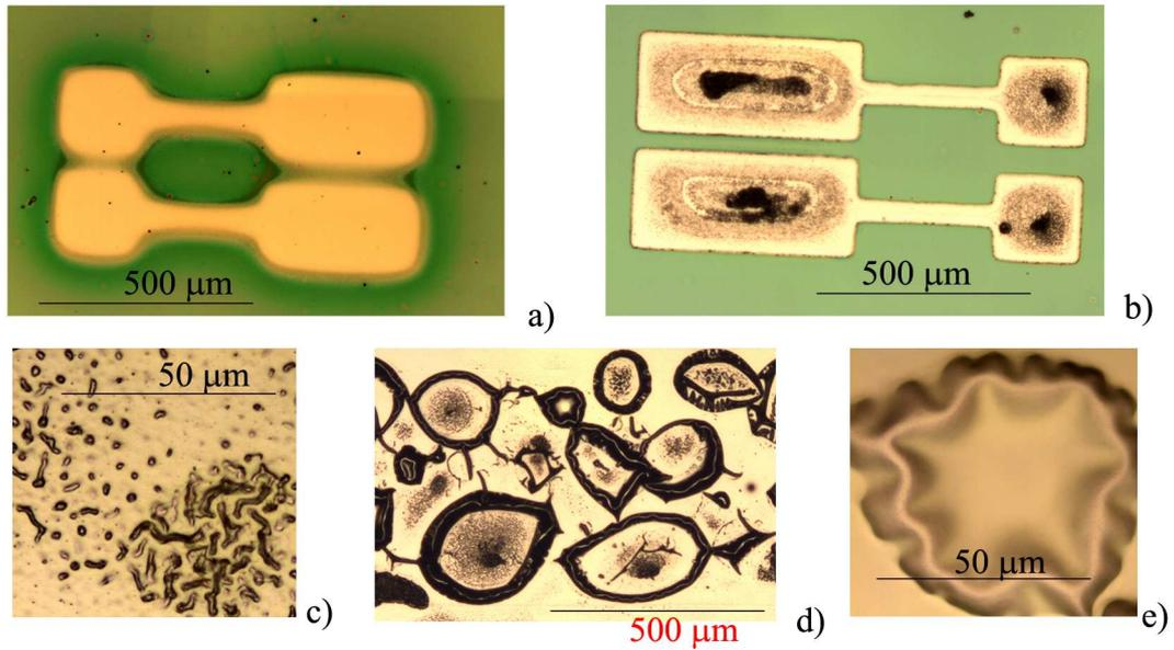
Figure J.8: *Optical microscope photographs on the top contacts: a) Au deposited on the PEPI film fabricated at LPQM; b)-d) Al deposited on PEPI fabricated i glove-box. c) and e) are represent a zoom of respectively b) and d). A separation between contacts is absent on (a) due to fabrication problems with this sample, still the photograph evidences the absence of degradation on the surface of the contacts.*
