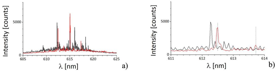
Figure H.6: *Fluctuations in the emission spectrum with variation of the pumping point location: a) whole spectrum; b) spectrum in the narrow wavelength range for better visualization. These are emission spectra accumulated during 0.1 s (a single pump pulse used for excitation) taken in two different pumping points at the pump intensity of  $73 \text{ MWcm}^{-2}$ .*
