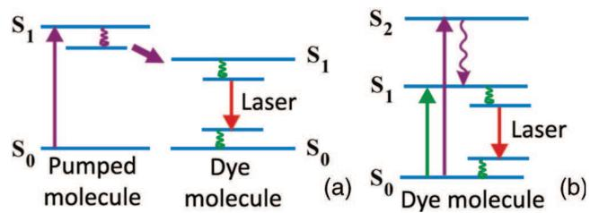
FIG. 9. (Color online) Pumping schemes are (a) via energy transfer from an excited molecule to the laser dye, (b) direct pumping to the  $S_2$  state of the dye laser.
