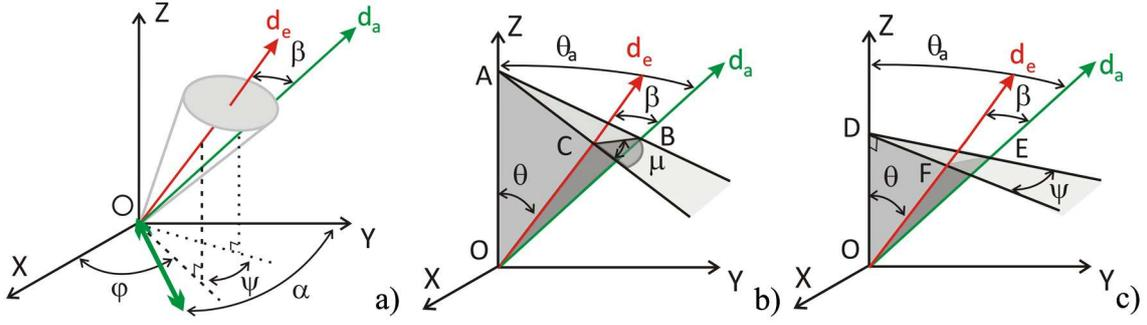
Figure B.1: *Illustration of the trihedral formula applied to the issue of relating the angles between absorption and emission dipoles: a) depiction of the orientation of the moments; trihedrons b) ABCO and c) DEFO in this system.*
