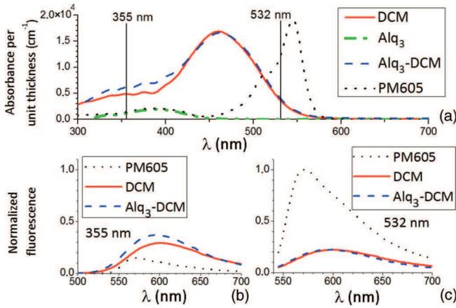
FIG. 11. (Color online) (a) Absorption spectra of PM605, DCM, Alq<sub>3</sub>, and Alq<sub>3</sub>-DCM. (b) and (c) Fluorescence spectra of PM605, DCM, and Alq<sub>3</sub>-DCM under pumping at wavelengths of 355 nm (b) and 532 nm (c), normalized by the maximum of PM605 fluorescence spectrum under 532-nm pumping wavelength.
