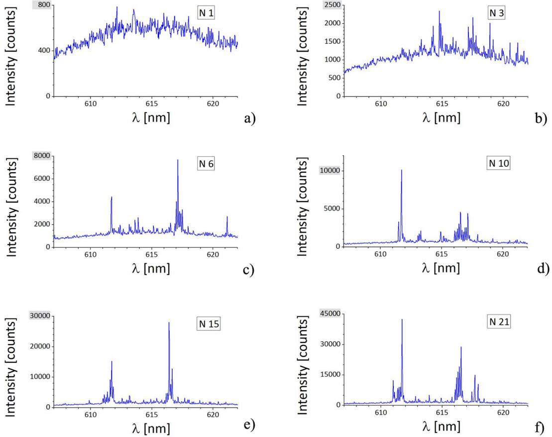
Figure H.3: *Emission spectra from the same measurement serie. Each spectrum was accumulated during 0.1 s (a single pump pulse used for excitation) under the fixed pump intensity of  $68 \text{ MWcm}^{-2}$ . Spectrum number: a) 1; b) 3; c) 6; d) 10; e) 15; f) 21. Measurement performed in the PMMA thin film doped with 5 wt% of DCM.*
