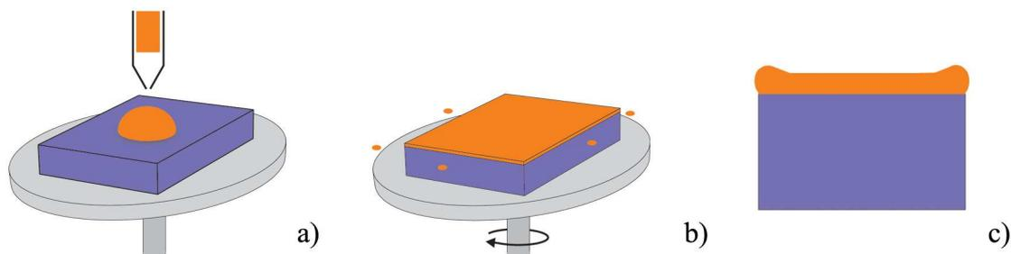
Figure 2.1: *Schematic depiction of the spin-coating process: a) deposition of a few droplets of the dye-polymer solution on a substrate; b) redistribution of the liquid during spinning; c) side view of the spin-coated layer (rounded parts show the accumulation of spun-coated material along the substrate border).*
