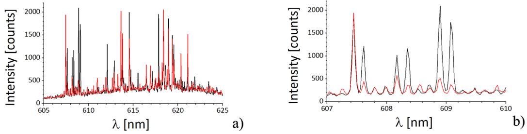
Figure H.4: *Fluctuations in the emission spectrum under fixed pump intensity level ( $95 \text{ MWcm}^{-2}$ ): a) whole spectrum; b) spectrum in the narrow wavelength range for better visualization. These are emission spectra accumulated during 0.1 s (a single pump pulse used for excitation) taken at the same pumping point.*
