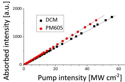
Figure 5.2: *Absorbed intensity under pulsed pumping (532 nm, 500 ps, 10 Hz) in a 600 nm thick PMMA layer doped with 5 wt% DCM (squares) or PM605 (circles) on a Si substrate, measured on the 3-D detection set-up (at 7° pump incidence) as a difference between signal reflected respectively from the reference substrate without polymer and from the sample. Present graph confirms the absence of absorption saturation effect in our system in the range < 50 MW cm<sup>-2</sup>.*
