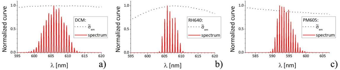
Figure 5.7: Normalized spectra of  $150\mu m$  width ribbon micro-lasers and normalized emission cross-section (deduced from Eq.(1.20) in Sub-section 1.1.4) for the given spectral region of the emission of dyes: a) DCM, b) RH640, c) PM605.
