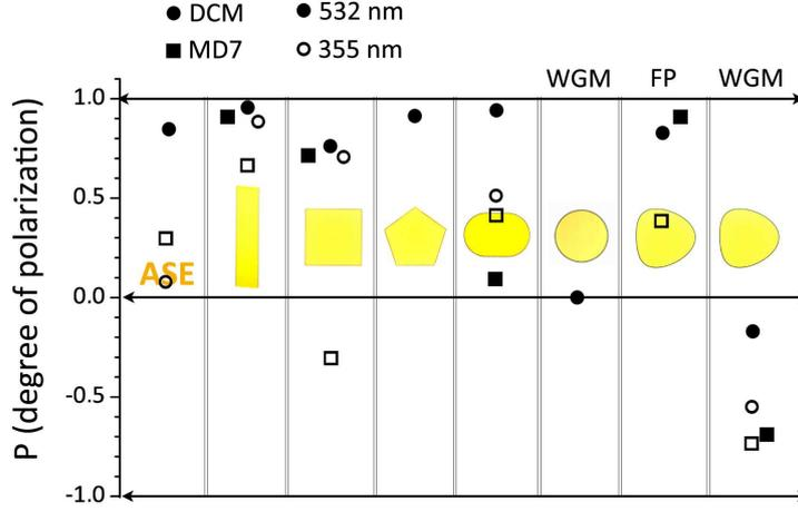
Figure 4.7: Comparison of the emission anisotropy in micro-lasers of various shapes, based on DCM (circles) or MD7 (squares) pumped to the  $S_1$  (solid icon) and  $S_2$  (empty icon) energy levels of the dyes.
