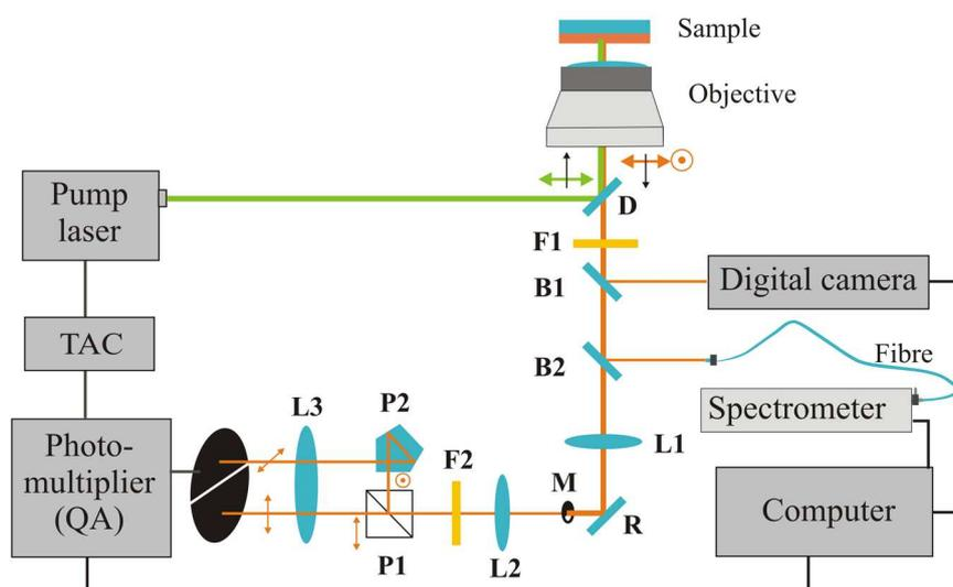
Figure 2.10: Scheme of the set-up used to study the fluorescence lifetime and polarization properties. Here  $F_{1,2}$  - filters for pumping wavelength,  $D$  - dichroic mirror,  $B_{1,2}$  - beam-splitters,  $R$  - mirror,  $L_{1,2,3}$  - lenses,  $P_1$  - Glan prism,  $P_2$  - pentaprism,  $M$  - mask, TAC - time-to-amplitude converter. The acousto-optical element and nonlinear optical crystal are included into the block of the pump laser.
