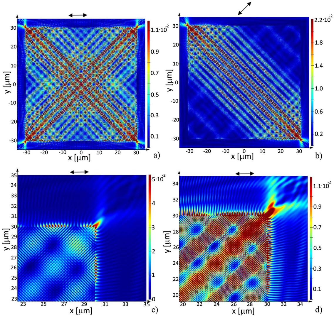
Figure 6.8: FDTD simulations of a  $60\ \mu\text{m}$  side square micro-laser for an in-plane polarization (at  $610.5\ \text{nm}$  peak). Mode patterns for a cavity pumped with a pump polarization at: a)  $\alpha = 0^\circ$ , b)  $\alpha = 135^\circ$ ; c-d) zoom at the corner of the cavity pumped with polarization at  $\alpha = 0^\circ$  with different intensity scales for the mode pattern in a.
