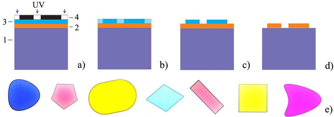
Figure 2.2: *Photo-lithographic fabrication scheme: 1 – wafer, 2 – dye-doped polymer layer, 3 – photo-resist layer, 4 – optical mask: a) irradiation by UV light; b) local changes in the chemical structure of the photo-resist; c) patterned photo-resist layer after developing; d) after plasma etching; e) optical microscope photos of the micro-lasers obtained by both methods (different dyes, top view).*
