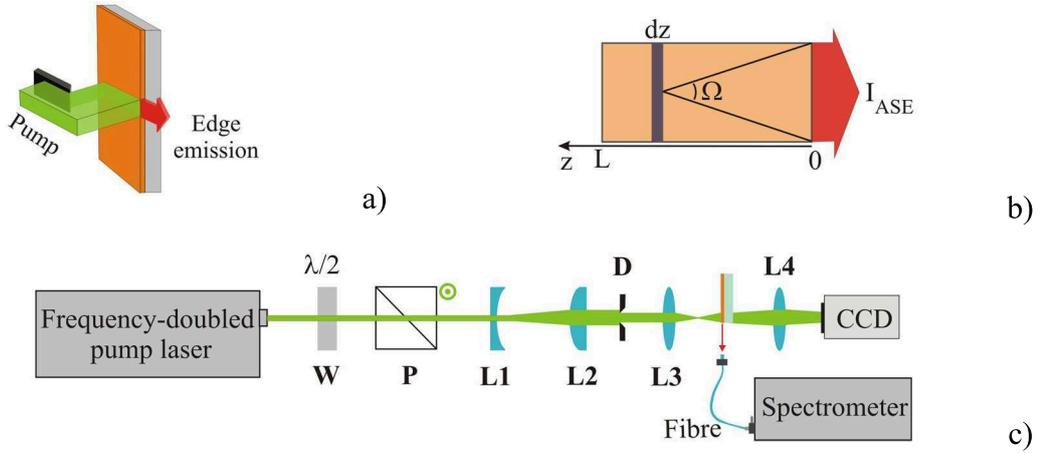
Figure 2.12: Variable Stripe Length (VSL) technique: a) pumping and emission configuration, the length of the pumping region is controlled with a blade; b) scheme for ASE calculation; c) experimental set-up. Here  $W$  is a half-wave plate,  $P$  - polarizer,  $L1-4$  stand for optical lenses and  $D$  for adjustable blades.
