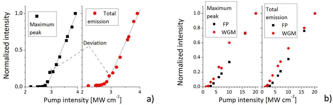
Figure E.2: *Illustration on the threshold analysis of a micro-laser emission: a) influence of the small peak intensity deviation on the threshold curve, built by maximum (left) or total (right) intensity in the spectrum of a 200  $\mu\text{m}$  ribbon Fabry-Perot micro-laser; b) influence of a co-existence of different modes on the threshold curve, built by maximum (left) or total (right) intensity in the spectral region occupied by a mode.*
