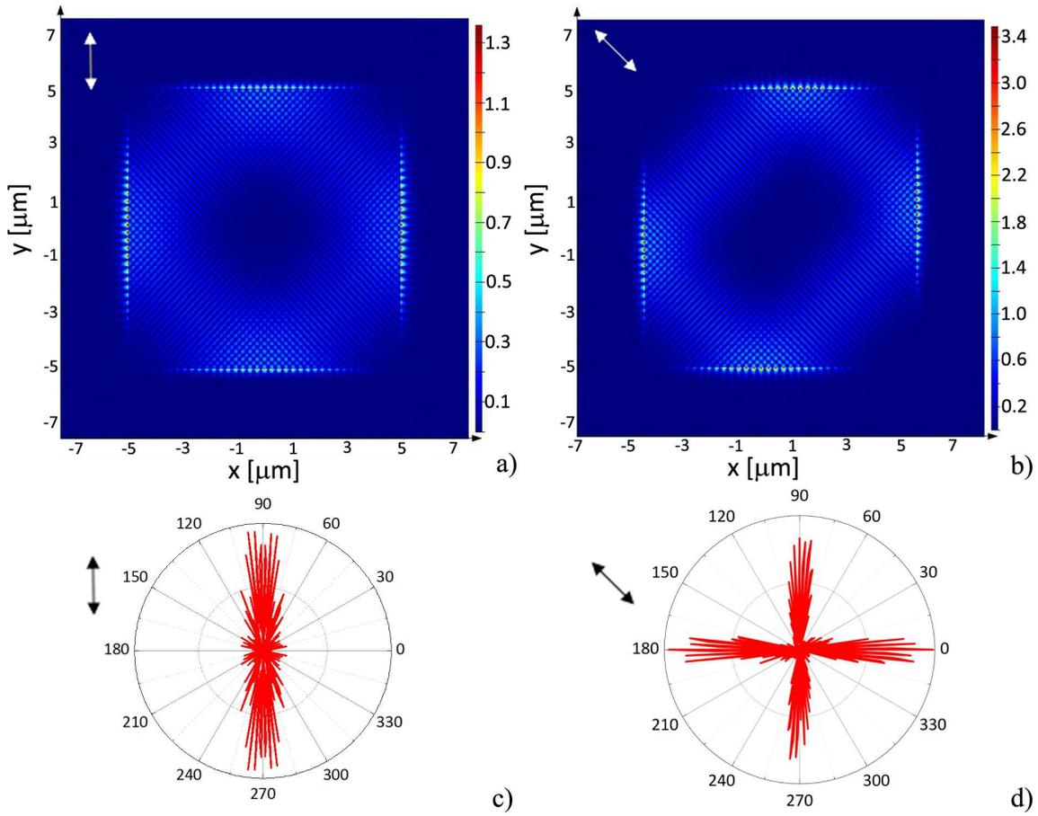
Figure 6.7: *FDTD simulations on a 10  $\mu\text{m}$  side square micro-laser for an in-plane polarization (TE, at 598 nm peak). Mode patterns (a,b) and emission diagrams (c,d) for pump polarization at: a,c)  $\alpha = 90^\circ$  (along the cavity side, represented by the arrow on (c)), b,d)  $\alpha = 45^\circ$  (along the cavity diagonal, represented by the arrow on (d)).*
