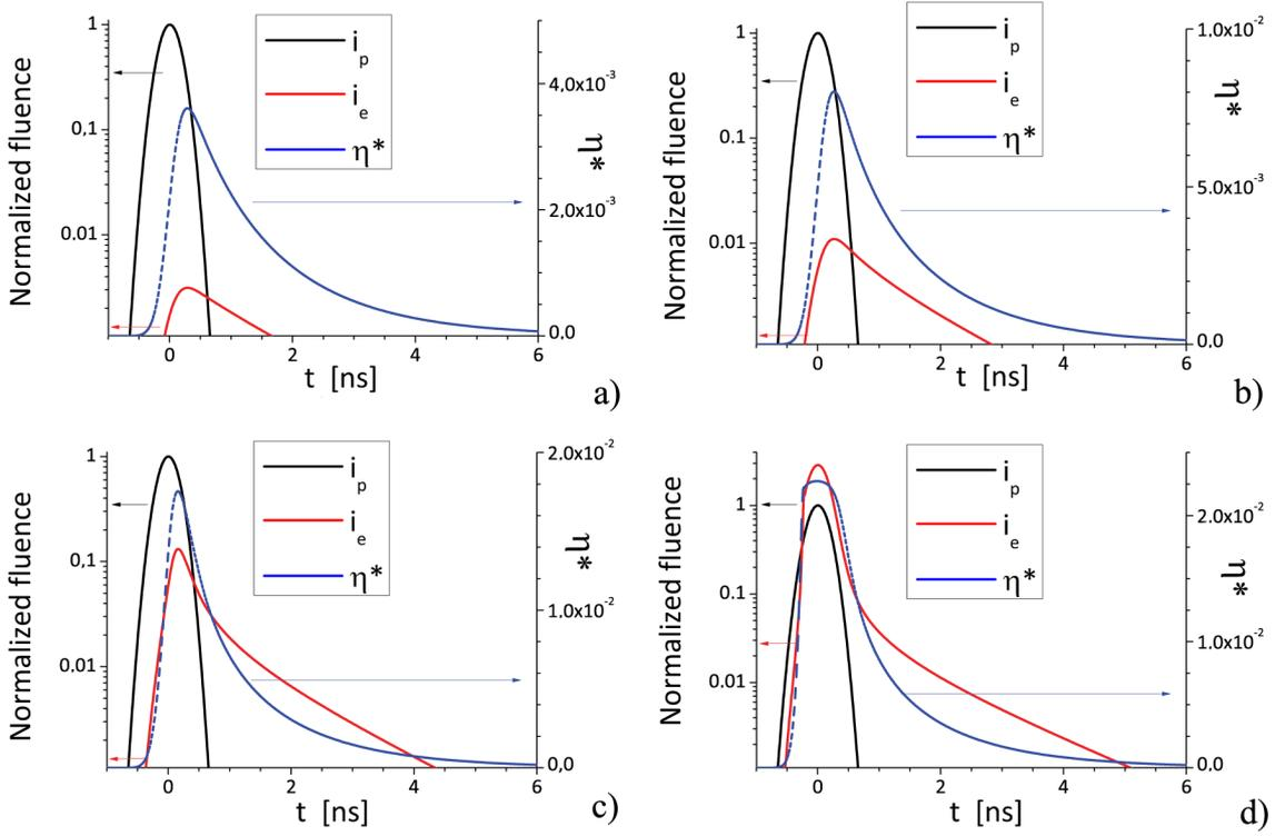
Figure 5.12: Results of numerical simulations on a laser emission dynamics, performed by equations (5.26) depending on  $I_{p0}$  : a) fluorescence emission ( $6 \text{ kW/cm}^2$ ); b) just below threshold ( $12 \text{ kW/cm}^2$ ); c) just above threshold ( $40 \text{ kW/cm}^2$ ); d) further above the threshold ( $0.4 \text{ MW/cm}^2$ ). The left scale shows the normalized intensity (scaled by the ratio of emitted over pump energy), and the right one the relative number of excited molecules.
