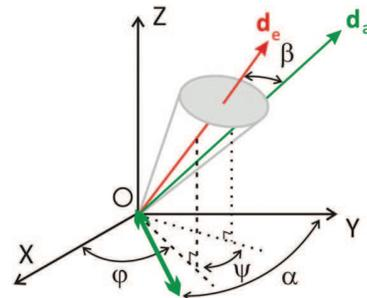
FIG. 12. (Color online) Notations are as follows: absorption ( $\vec{d}_a$ ) and emission ( $\vec{d}_e$ ) transition dipoles are oriented at the angles  $\theta_a$  and  $\theta_e$  with respect to the  $z$  axis,  $\beta$ , angle between the moments,  $\psi$ , between their projections on the  $xy$  plane,  $\varphi$ , angle between the  $x$  axis and projection of  $\vec{d}_e$  on the  $xy$  plane,  $\alpha$ , angle between the  $y$  axis and the pump beam polarization (thick green arrow).
