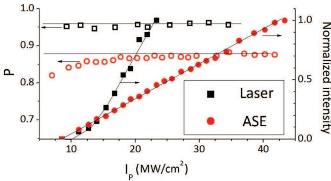
FIG. 5. (Color online) Degree of polarization  $P$  versus the pump intensity  $I_p$  (per pulse) for ASE and Fabry-Perot in planar microresonator configuration for a DCM-PMMA layer. The intensity of emission versus  $I_p$  is presented for comparison. Thin lines are drawn for guiding eyes.
