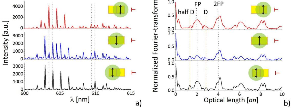
Figure I.5: *Emission of the system of two closely placed micro-lasers (1  $\mu\text{m}$  gap) with excitation geometry varied (indicated by the scheme next to each plot): a) emission spectra; b) normalized Fourier-transform (lengths of periodic orbits are indicated with FP and D: Fabry-Perot  $FP = 2an$ ; diamond  $D = 2\sqrt{2}an$ ). Excitation was made with the intensity of  $38.5 \text{ MWcm}^{-2}$  with polarization orthogonal to the emission direction ( $\alpha = 90^\circ$ ).*
