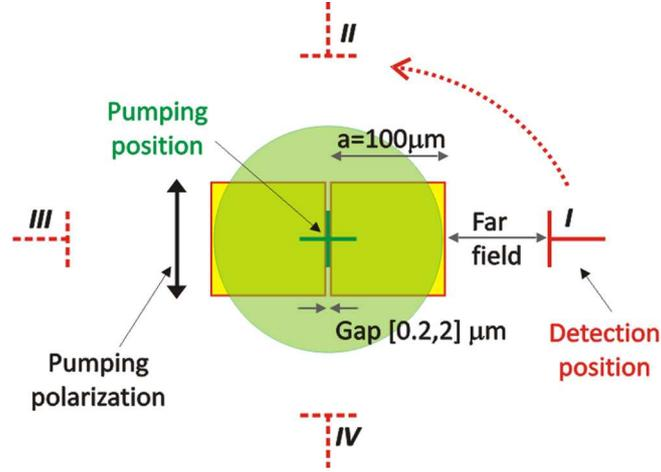
Figure I.2: *Scheme on the symmetric pumping configuration. Pumping beam is centered with the symmetry center of the system, while the detection in the far field is performed in the sample plane at several angular positions depicted by I, II, III and IV. Pumping beam dimensions are realistic.*
