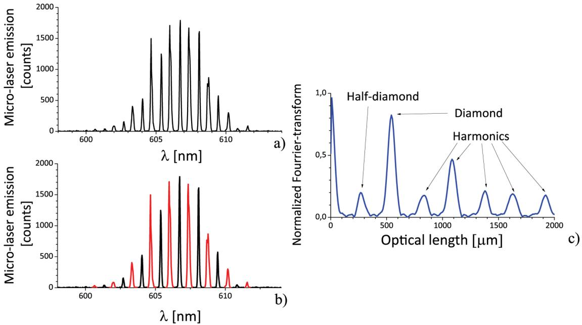
Figure 6.3: *Square micro-laser: a) spectrum in the direction of maximum emission, b) spectrum in (a) presented as superposition of two combs, c) Fourier-transform of the spectrum in (a).*
