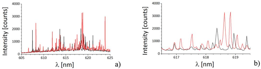
Figure H.5: *Fluctuations in the emission spectrum with the pump intensity variation: a) whole spectrum; b) spectrum in the narrow wavelength range for better visualization. These are emission spectra accumulated during 0.1 s (a single pump pulse used for excitation) taken at the same pumping point. Pump intensities applied are  $95 \text{ MWcm}^{-2}$  for spectrum presented in black and  $110 \text{ MWcm}^{-2}$  for spectrum presented in red.*
