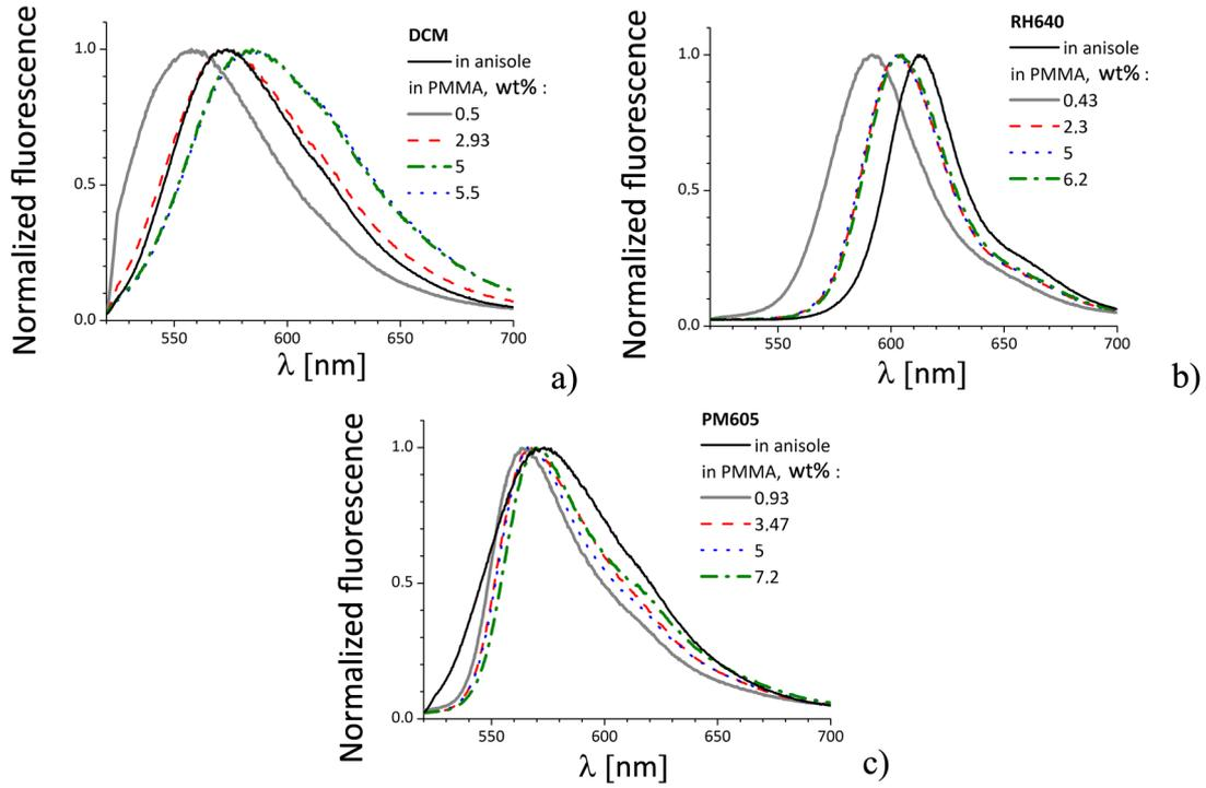
Figure 1.10: Illustration on the influence of the molecular environment on the emission properties of dyes. Fluorescence spectra of various concentrations of the dye respectively in a thin PMMA film and in an anisole solution (without PMMA): a) DCM, b) RH640 and c) PM605.
