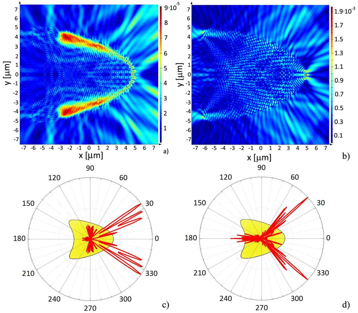
Figure G.1: *FDTD simulations on 5  $\mu\text{m}$  radius kite with  $\delta = 0.5$ : field patterns (a,b) and emission diagrams (c,d) for TE-polarized at 611 nm (a,c) and TM-polarized emission at 614 nm (b,d).*
