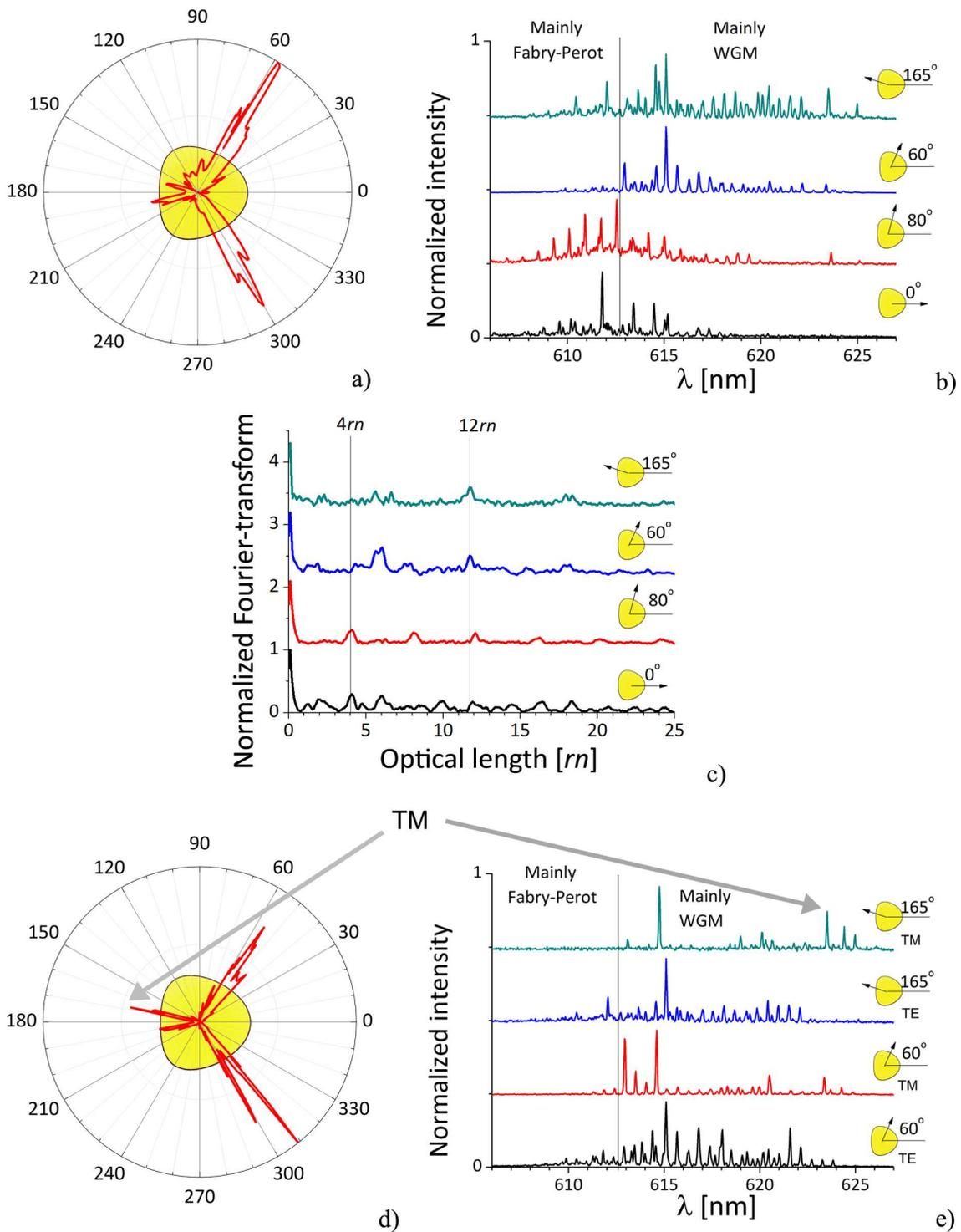
Figure 6.27: *Experimental emission properties of a  $r = 70\mu\text{m}$  kite made of DCM: a) emission diagram representing the total intensity in spectrum; b) spectra at some directions of emission maxima; c) Fourier-transform of the spectra given in (b); d) diagram of emission at 623 nm; e) polarization components of the emission spectra at 60° and 165° (TE - within the cavity plane, TM- orthogonal to the plane).*
