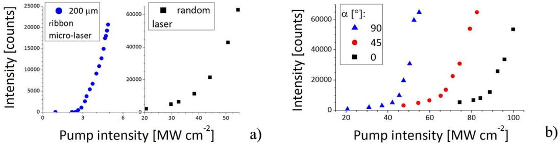
Figure H.2: *Threshold curves of the random laser in thin PMMA film doped with 5 wt% of dye: a) DCM; b) RH640. (a) random laser threshold versus 200 μm large ribbon micro-laser, both had pump beam polarization a orthogonal to the emission direction ( $\alpha = 90^\circ$ ). (b) influence of the pump beam polarization  $\alpha$  on the random laser threshold for RH640-based sample. These curves were built from 3 s integration spectra.*
