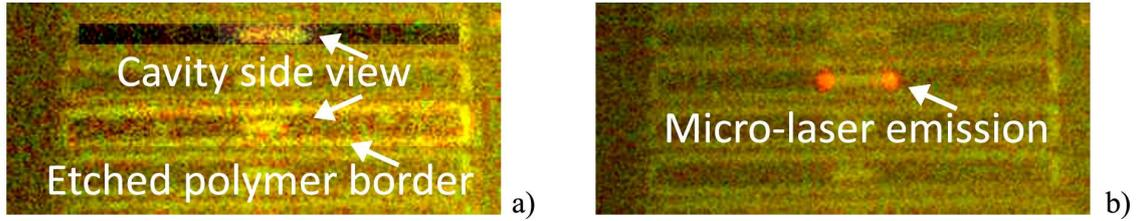
Figure 6.9: Image from the uEye CCD camera (sample lightened by a table lamp): a) alignment, b) lasing.
