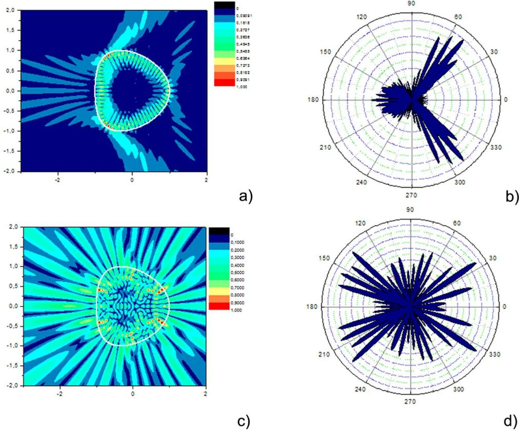
Figure 6.23: LEP map fields (a,c) and emission diagrams (b,d) for a kite with  $\delta = 0.165$ , and  $(ka; \gamma) = (23.74; 9.55 \cdot 10^{-3})$  (a,b) and  $(23.5; 4.56 \cdot 10^{-2})$  (a,b). Refractive index  $n=1.5$ , discretization over a set of  $N=100$  points.
