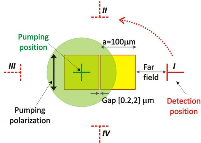
Figure I.3: *Scheme on the non-symmetric pumping configuration. Pumping beam is centered with the symmetry center of the system, while the detection in the far field is performed in the sample plane at several angular positions depicted by I, II, III and IV. Pumping beam dimensions are realistic.*
