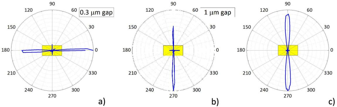
Figure I.9: Emission diagrams obtained under circular pumping beam polarization: a) couple of squares with  $0.3\mu\text{m}$  gap; b) couple of squares with  $1\mu\text{m}$  gap; c) rectangle 2:1. Diagrams represent integration of the whole emission spectrum.
