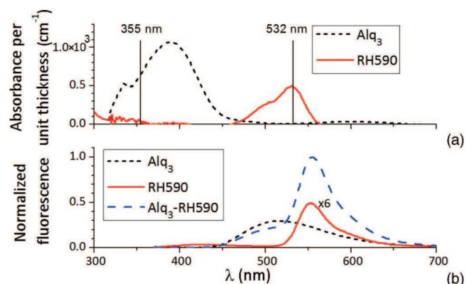
FIG. 10. (Color online) (a) Absorption spectra of Alq<sub>3</sub> and RH590. (b) Fluorescence spectra of Alq<sub>3</sub>, RH590 and Alq<sub>3</sub>-RH590 under the same pump intensity at 355 nm. They are normalized by the maximum of Alq<sub>3</sub>-RH590 fluorescence spectrum and the variation of layer thickness is taken into account.
