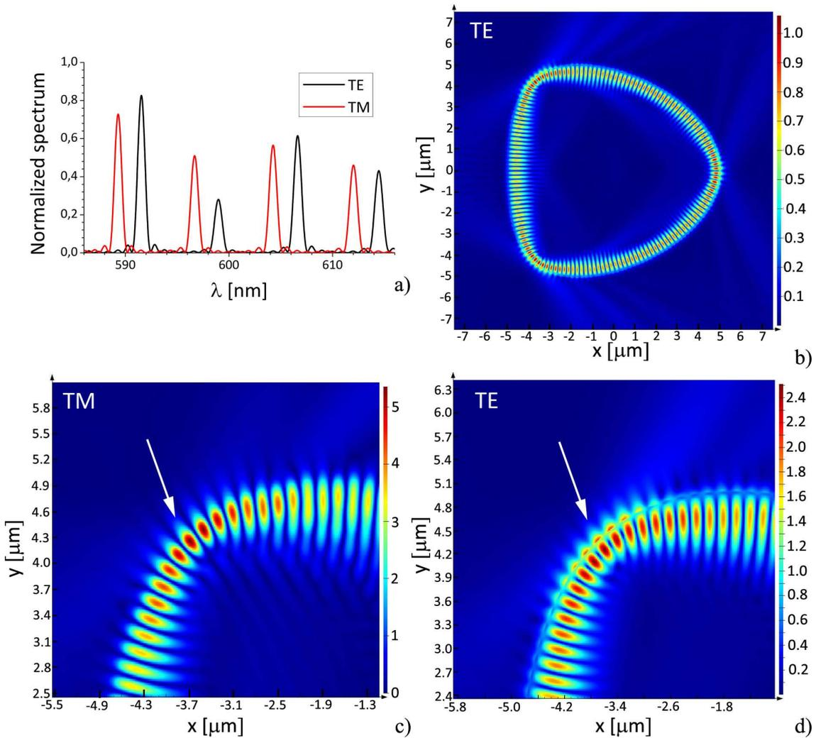
Figure 6.24: Mode patterns obtained with FDTD simulations for a  $r = 5 \mu\text{m}$  kite with  $\delta = 0.165$ : a) spectra of TE and TM-polarized mode; b) mode pattern at 606.5 nm resonance (TE-polarized). c),d) zoom of the mode map: c) 597nm resonance (TM), d) 606.5 nm resonance (TE).
