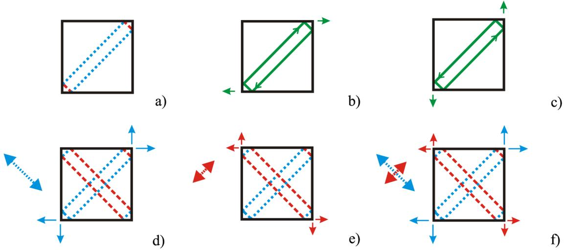
Figure 6.12: *Scheme of orbits inside the cavity and out-coupling: a) round trip of the diamond in-family periodic orbit, regions oriented along different diagonals are shown in dash and dot; b), c) out-coupling of same spatial mode with light propagating in opposite directions; d),e) cavity emission under linear pump beam polarization along the cavity diagonal; f) combination of d) and e), which accounts for the emission in the real system.*
