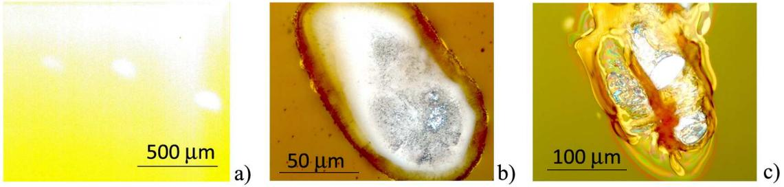
Figure 4.8: *Degradation process during ASE measurements on the PMMA layer doped with 5 wt% of DCM: a) bleaching, b) beginning of polymer melting, c) propagation of polymer melting. Pump intensity about  $150 \text{ MW cm}^{-2}$ .*
