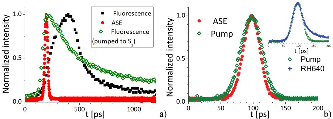
Figure 4.4: Dynamics of the spontaneous and the stimulated emission in a layer of PMMA polymer doped with 5 wt% of DCM dye: a) fluorescence and ASE (error  $\pm 60$  ps, solid squares and circles represent respectively fluorescence and ASE under  $S_2$  pumping), b) pump signal and ASE (error  $\pm 1.3$  ps, ASE of RH640 in the inset for comparison).
