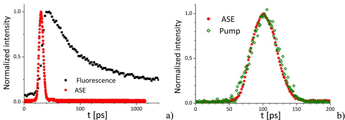
Figure 3.13: *Dynamics of the spontaneous and the stimulated emission in a layer of PMMA polymer doped with 5 wt% of DCM: a) fluorescence and ASE (error  $\pm 60$  ps), b) pump signal and ASE (error  $\pm 1.3$  ps).*
