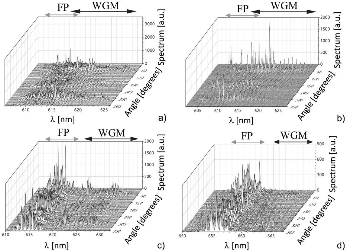
Figure 6.28: Emission spectra of kite micro-lasers at various angle observation: a)  $70 \mu\text{m}$  radius, DCM-based; b)  $40 \mu\text{m}$  radius, DCM-based; c)  $70 \mu\text{m}$  radius, MD7-based; d)  $70 \mu\text{m}$  radius, MD48-based.
