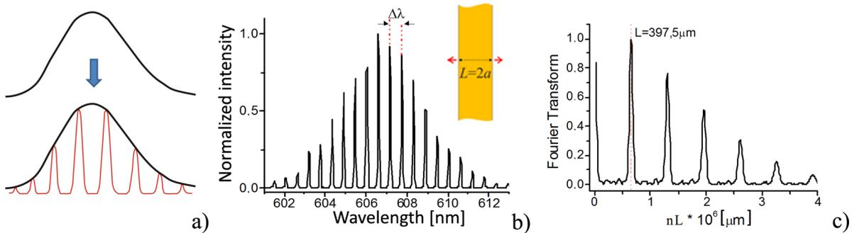
Figure E.1: *Illustration on the analysis of a micro-laser spectrum: a) resonator combs as result of constructive interferences; b) typical spectrum of planar ribbon Fabry-Perot micro-laser; c) Fourier transform of the spectrum depicted on (b).*
