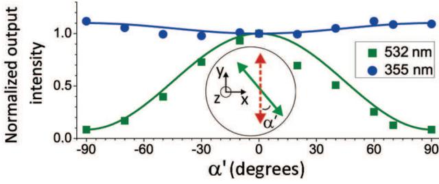
FIG. 7. (Color online) Normalized intensity emitted from a VECSEL with a PMMA-DCM gain material, versus the angle  $\alpha'$  of the pump polarization. Comparison between a 532-nm pump (green, squares) and a 355-nm pump (blue, circles), after corrections from bleaching. The curves are fitted according to Eq. (3). (Inset) Scheme of a VECSEL section. The polarization of emission is fixed and represented as a dotted red arrow, while the linear pump polarization is shown as a green continuous arrow.
