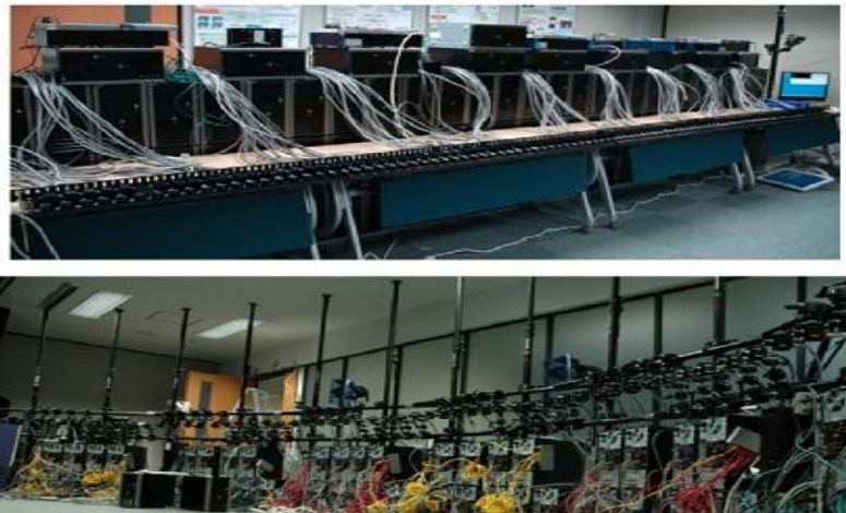
Figure 1-11 : A 100-camera multiview system (Fig 6. from (Jolly et al., 2009) )
