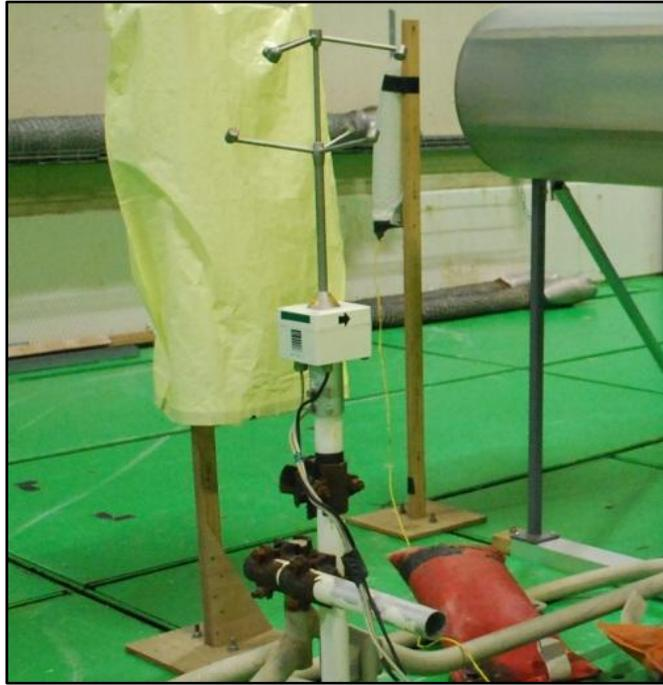
Figure 49. The ultrasonic anemometer on its support.
