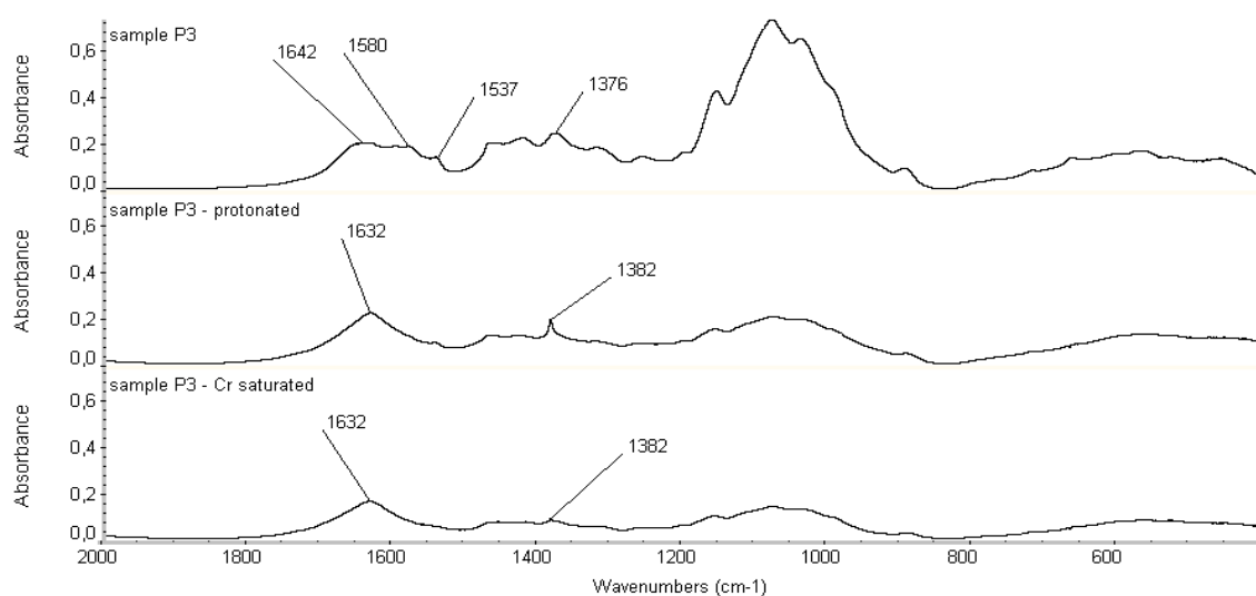
Figure 52 Detail of comparison of protonated, chromium saturated and original P3 spectra ( 2000 - 400\text{ cm}^{-1} )
