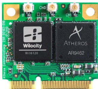
Figure 1.29: Wilocity's chip for IEEE 802.11ad communications at 60GHz paired with a Qualcomm Atheros' chip for IEEE 802.11n networking, from [14].
