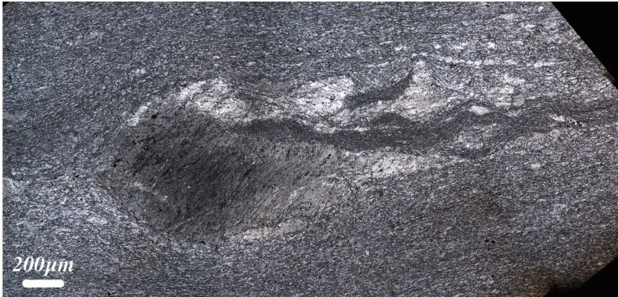
Figure 10: "Retort -shaped" calcite crystal embedded in a finely recrystallized calcite matrix (~80% have a grain size <math>15\mu\text{m}</math>, and ~50% <math>10\mu\text{m}</math>). The mylonitic foliation wraps around the porphyroclasts the upper part of which was more strongly sheared than the lower part and displays evidence of dynamic recrystallization. Polarized-analyzed reflected light. Sample # 10AG1B.
