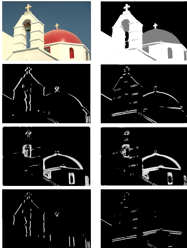
FIGURE A.6 – U -variable maps : the first row shows the original image and the segmentation for K = 3 clusters ; the rows below show U -variable maps (expected values of u_j^{nk} variables). Brighter values represent lower values of u . In each row, the U -variable maps for kernel indexed by j = 1 ( sky ), j = 2 ( roof and shadows ) and j = 3 ( building ), are shown respectively. The left column corresponds to u values computed for horizontal adjacencies, and the right column for vertical adjacencies.
