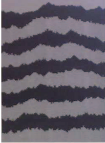
Figure 1.4: The interface after depositing 35000 particles on substrate with size L = 100 .
