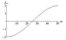
Figure A.1: Eigenvalues of 1D chain. The size is chosen N=5O sites and the parameters  $\epsilon = 0$  and t = 1. All the eigenvalues are non degenerate
