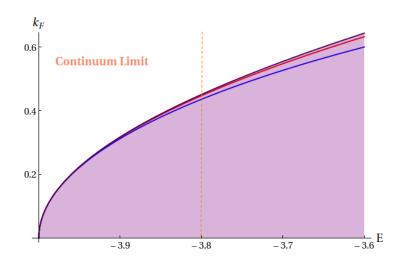
Figure E.1: different formulas of  $k_F$  near the bottom of the conduction band. Formula (b): Red curve, formula (c): Purple curve, formula (d): Blue curve. The continuum limit is the region of energies where the three curves are very close.
