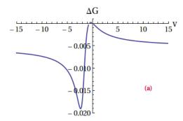
Figure 3.13: Numerical simulation for  $\Delta G$  vs the tip potential for Dirac delta model and completely open first mode. The tip is positioned at x=40a far from the QPC. The effect is always negative and show a resonance at some negative potential value. ( $\Delta G$  in units of  $\frac{2e^2}{h}$  and 'a' is the step of the lattice).
