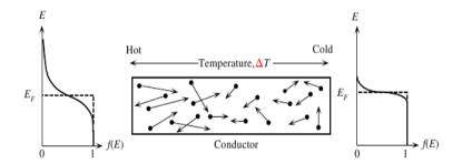
Figure 5.1: A conductor sketched between a hot and a cold electron reservoir. The Seebeck coefficient is given by the ratio between the difference of the two reservoirs temperatures and the voltage  $\Delta V$  induced by the difference  $\Delta \mathcal{T}$ . Taken from [63]
