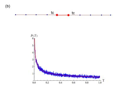
Figure 6.9: Transmission probability distribution: The transmission is distributed according to the law  $\frac{1}{2\sqrt{T}}$  (red color). The system considered in simulation is shown in top figure. The Hamiltonian is taken from Lorentzian orthogonal ensembles with mean  $(E - \Delta(E))$  and width  $\Gamma/2$ .
