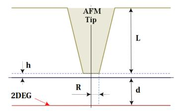
Figure 3.8: Geometry used in Poisson-3D simulation. adapted from [37]
