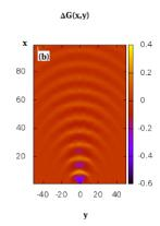
Figure 3.1: Spatial map of the zero temperature conductance change  $\Delta G(x,y)$  in units of the quantum conductance  $\frac{2e^2}{h}$  for two different models of the QPC. (a) a Wide-narrow-wide model shown in Fig. (1.7). (b) Potential V(x,y) defined with Eq. (3.1). The effect of the tip on the 2DEG is modeled with an on-site potential at position (x,y).
