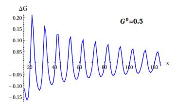
Figure 3.10: Change in the conductance (in units of  $\frac{2e^2}{h}$ ) as a function of the tip position. The tip is Lorentzian and the QPC realistic. The conductance of the systems without tip is  $G^{\circ} = 0.5$ . The position x is in units of the the lattice step a. The effect has both signs: negative and positive.
