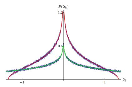
Figure 6.12: Verification of the Seebeck coefficient density function at arbitrary Fermi energy: E=1.7 (Green curve) and E=-1 (Red curve). The agreement between simulation and the analytical expression is excellent. The density function has a singularity at the origin. The density function is non-zero over a range  $\frac{8}{\Gamma^2}$ .
