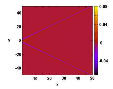
Figure 5.3: The change  $\Delta \Re \Sigma(x,y)$  in the real part of the self energy of a 2D lead as a function of the tip position. This result is given at the half filling limit. The effect of the tip is significant only in two directions  $\pm 45^{\circ}$ .
