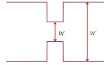
Figure 1.7: Wide-narrow-wide model: the attachment of the central region to the leads is abrupt.
