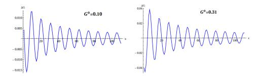
Figure 3.2:  $\Delta G$  as a function of the tip position for a pinched off QPC
