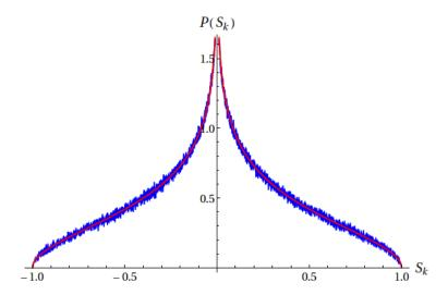
Figure 6.10: The distribution of the Seebeck coefficient  $S_k$  at half filling limit (E=0).  $S_k$  is bounded and the distribution is singular at the origin. The numerical simulation is well fitted with the function obtained analytically. This Seebeck is for a chaotic cavity connected to two 1D leads(one conducting mode in each one).
