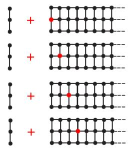
Figure 2.9: Each time we add a perfect slice to a semi-infinite lead from the left, the situation is equivalent to moving the charged tip (Red color) one step to the right
