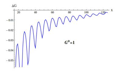
Figure 3.11: Change in the conductance (in units of  $\frac{2e^2}{h}$ ) as a function of the tip position. The tip is Lorentzian and the QPC realistic. The conductance of the systems without tip is  $G^{\circ} = 1$  (First plateau of conduction). We notice that the effect is always negative.
