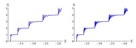
Figure 1.8: Transmission profile for a wide-narrow-wide model. In the right Fig, the length of the constriction is twice the length of the constriction which gave the left Fig. In both figures Fabry-Perot oscillations are visible. The bottom of the conduction band is taken at -4 (units of  $t_h$ ). The conductance is expressed in units of the quantum  $2e^2/h$
