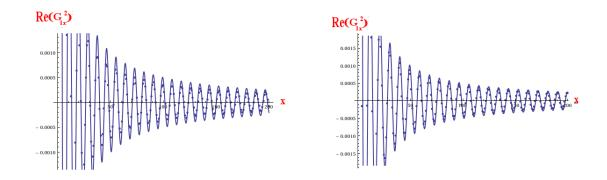
Figure 5.4: Comparison between numerical calculation(blue dots) obtained with the exact formula and the formula (5.32) (Blue curve) for the 2D change in the  $\Re(G_{1x(y)})^2$ . The figure in the right is obtained for an angle  $\alpha=18.43$  (i.e x=3y) and the figure in left is obtained for  $\alpha=26.56$  (i.e. x=2y)
