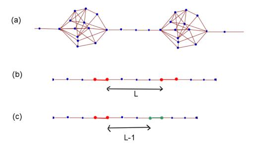
Figure 6.14: Decimation-renormalization procedure on a system composed of two chaotic cavities in series: First step, from (a) to (b), it replaces the two cavities with two minimal models distributed according to  $\mathcal{L}OE$ . The distance between the two scattering systems is noted L. The second step is to do again the decimation procedure on one of the two minimal systems, which shortens the length between the new scattering systems (L-1).
