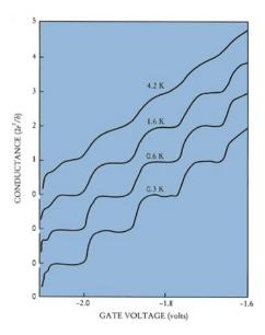
Figure 1.3: Conductance quantization in a quantum point contact in units of  $2\frac{e^2}{h}$  for different temperatures. Van Houten et al [2]
