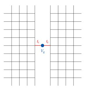
Figure 4.1: Toy Model to mimic transport through nanoconstrictions: One site biased to potential  $V_g$  and connected to two semi-infinite 2D leads via the coupling elements  $t_c$ .  $V_g$  and  $t_c$  both control the conductance of the system.
