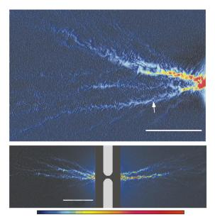
Figure 1.10: Experimental results on conductance changes with SGM technique. An interference pattern of  $\lambda_f/2$  fringes is obtained. We notice small angle scattering and branching strands for the electronic flow. the temperature in this experiments is 1.7 K . TopinKa et al [1].
