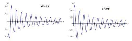
Figure 3.3: The effect of the tip along the central axis of the system for the first mode of conduction. The figures are given for different cases of the QPC opening. The conductance is expressed in units of  $\frac{2e^2}{h}$ . Lead width N = 2001a. The tip is a Dirac delta function (on-site potential)
