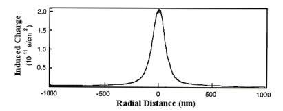
Figure 3.9: Profile of the charge induced by the tip on a 2DEG of density  $n=4.2\ 10^{11}e/cm^2$  obtained by numerical simulation. The tip is 10nm above the sample surface. Adapted from [37]
