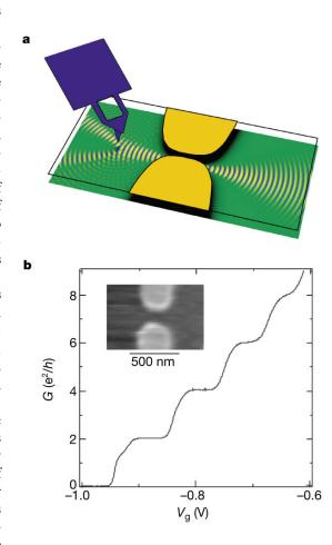
Figure 1: (a) Scanning Gate Microscopy on a Quantum point contact. (b) Conductance quantification. Topinka et al, Nature 2001
