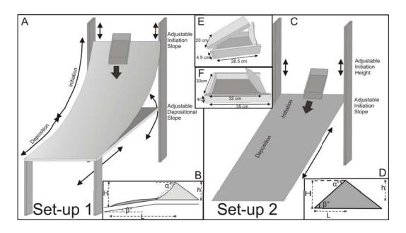
Figure 5.1: Analogue slides set-up. A, B Curved Ramp configuration for Set 1: the initiation and deposition slopes can be varied. C, D Inclined Straight Ramp configuration for Set 2: both the initiation, a and deposition slopes,  $\beta$  can be changed with height of initiation. E Source Box 1 with a simpler geometry. F Source Box 2 with inclined trapdoor and open lid.
