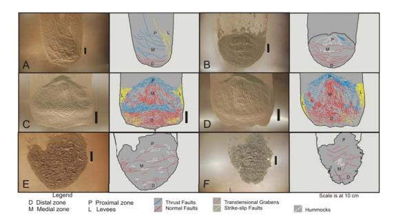
Figure 5.2: Set 1: Curved ramp analogue avalanches using the powder-size glass beads. Source slopes are at  $35^{\circ}$ ,  $45^{\circ}$ , and  $55^{\circ}$ ; deposition slopes are at  $0^{\circ}$ ,  $10^{\circ}$ , and  $18^{\circ}$ ; and volume of glass beads at 1000 and 2000 cm<sup>3</sup>
