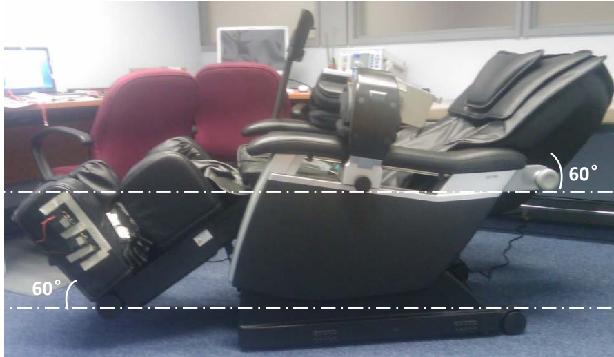
Figure 114 Inclination of OSIM massage chair during trial
