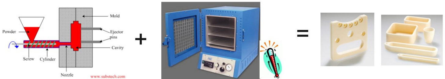
Figure 129 Molding process for ceramics. Samples taken from Friatek portfolio 17 .
