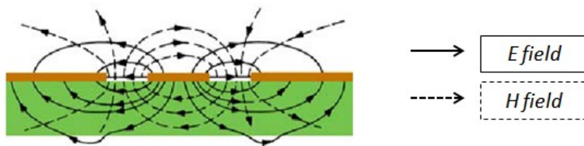
Figure 27 TEM Mode of a CPW line (transversal view) [21]
