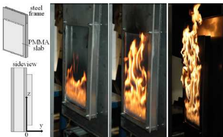
Fig. 2. PMMA slab configuration with steel frame to limit the combustion area ( 40 \times 20 cm) and location of y and z axes. On the right, pictures of flame spread at 60, 300 and 1500 s.
