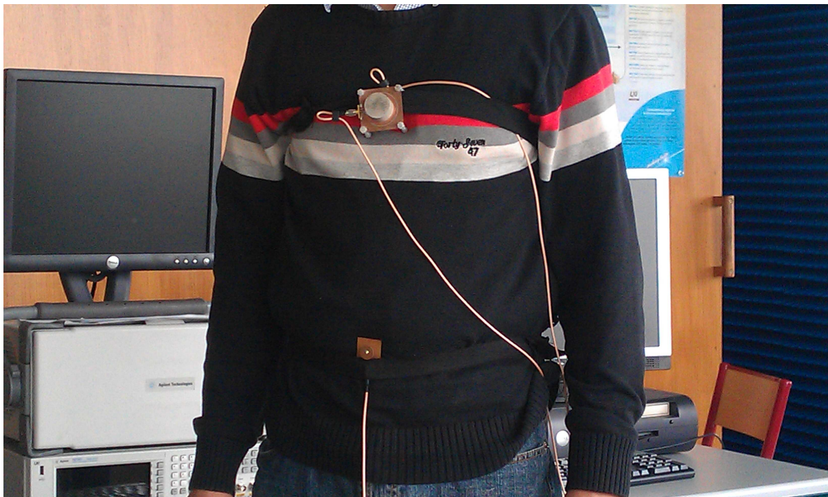
Figure 5.7: A person is walking in the laboratory by wearing diversity antenna in receiving mode at chest while top loaded monopole in transmitting mode at belly.
