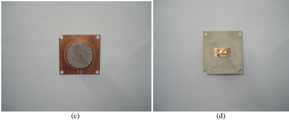
Fig3.36: DRAs fabricated designs at 2.4GHz; aperture slot fed: (a) top view (b) bottom view & monopole fed: (c) top view (d) bottom view
