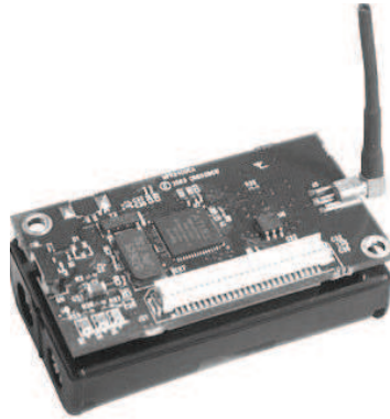
Figure 5.1: MICAz mote for which the idea is proposed. These motes lose their battery voltage with the passage of time.
