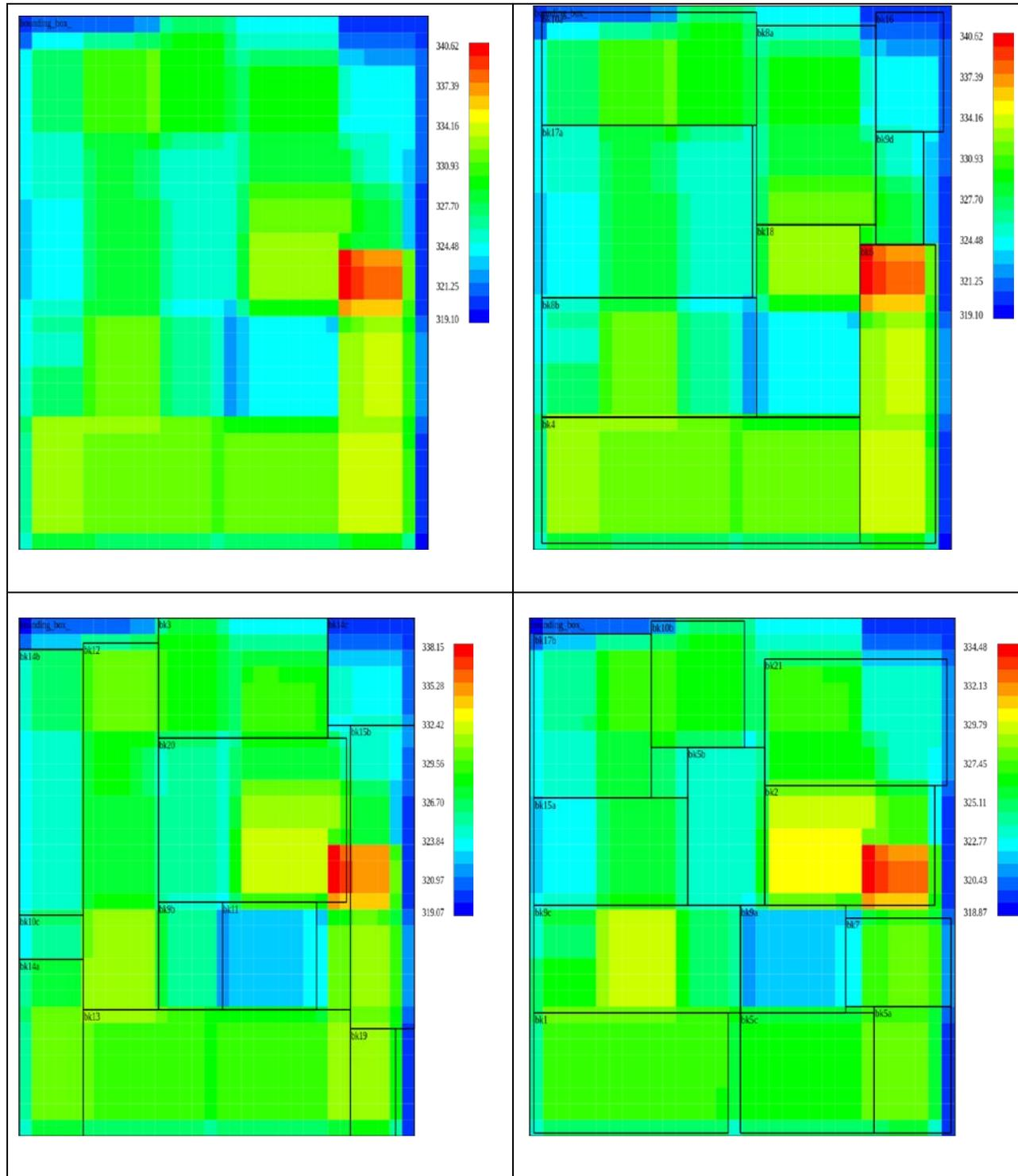
Figure 4.17 Test case 1 result – Thermal map
