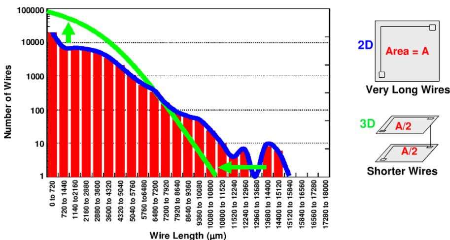
Figure 1.5 2D vs 3D wirelength distribution [18]
