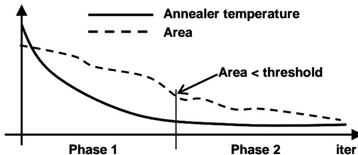
Figure 4.8 Two-phase algorithm and the switching criteria
