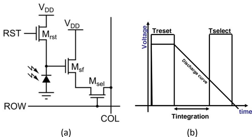
Figure 3.4 (a) 3T-APS structure (b) Timing graph
