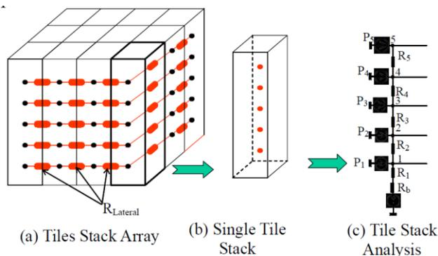
Figure 4.6 Simplified thermal model [10]
