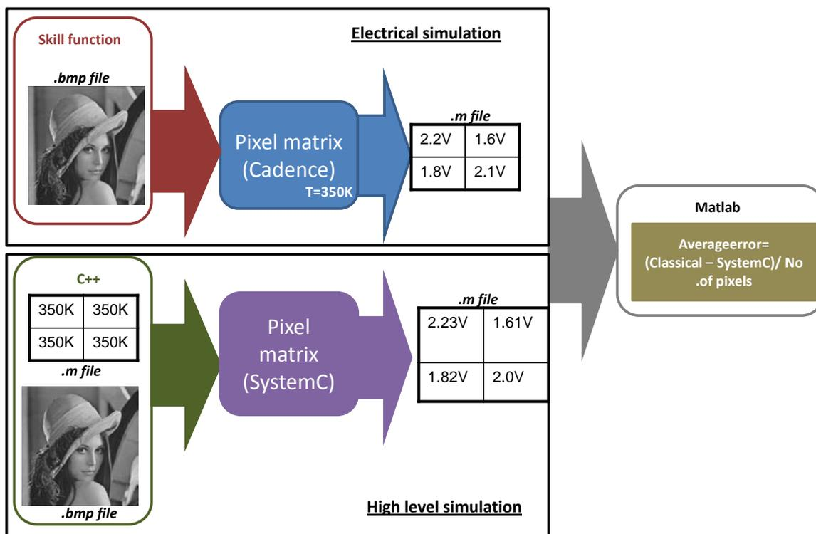
Figure 3.29 Post validation steps and used tools
