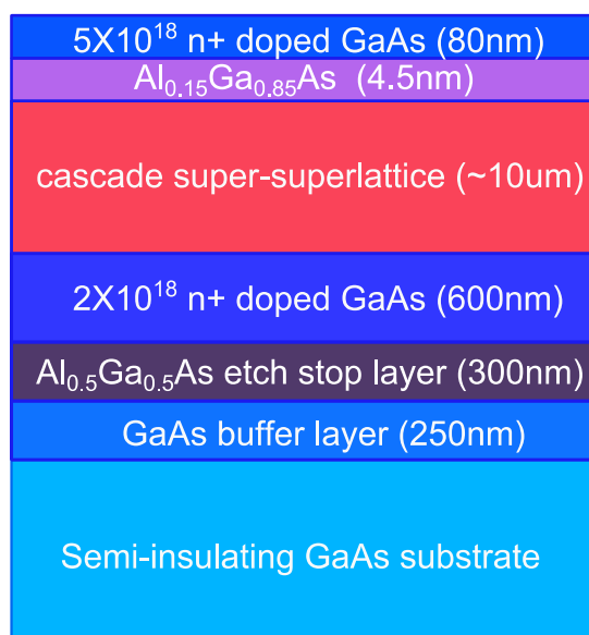
Figure 3.10: Structure of the MBE-grown doped Bloch samples, showing the thickness and the doping of the sacrificial layers, the active region and the contact layers.
