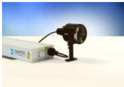
FIGURE II.1.5: Dantec ShadowStrobe (source : http://www.dantecdynamics.com )
