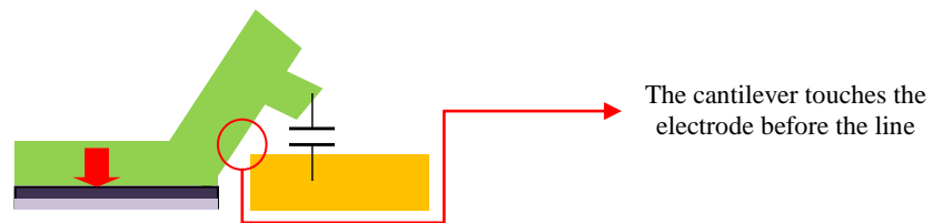
Fig. 2-19: Schema of the contact between the line and the cantilever in the actuated state. The red arrow show where the electrostatic force is applied
