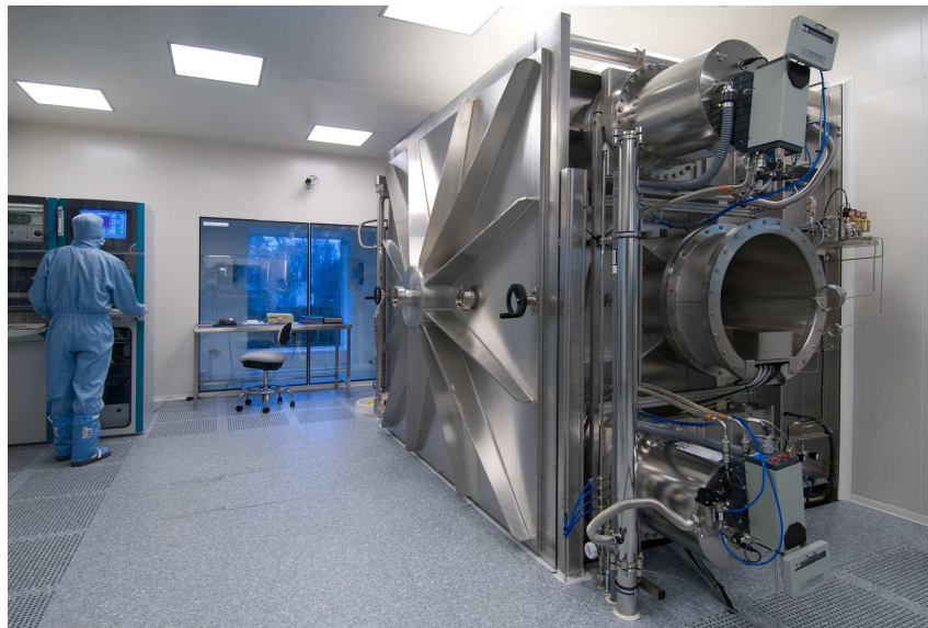
Figure 6.4: The large Ion Beam Sputtering coating machine.
