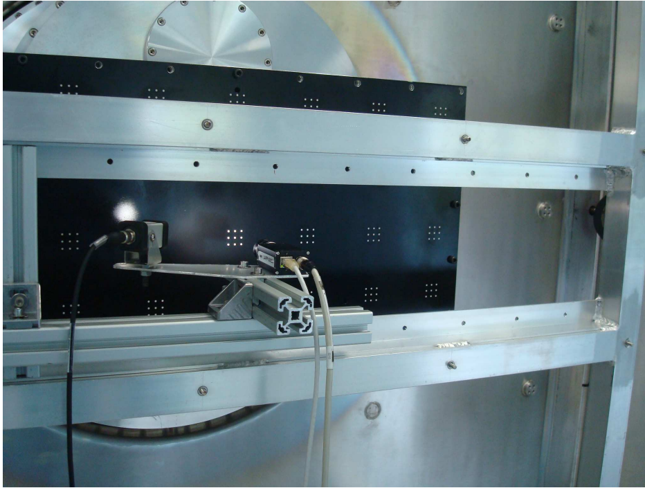
Figure 5.13: Camera set up to test the accuracy of the robot in terms of positioning.
