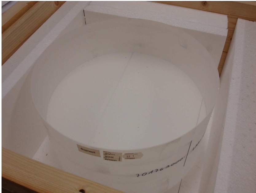
Figure 1.12: Input mirror blank (35 cm diameter, 20 cm thickness).
