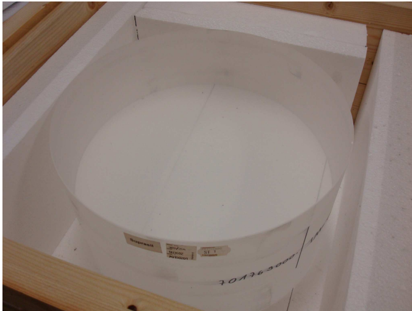
Figure 1.12: Input mirror blank (35 cm diameter, 20 cm thickness).
