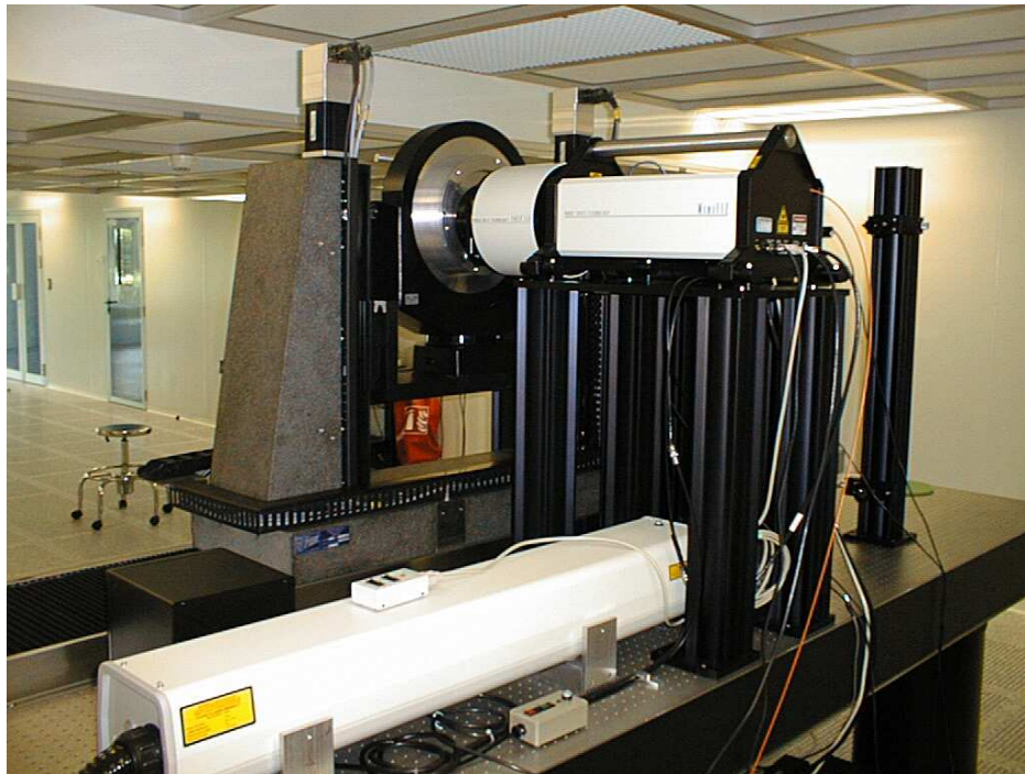
Figure 4.2: The Minifiz phase-shifting interferometer on the metrology bench.
