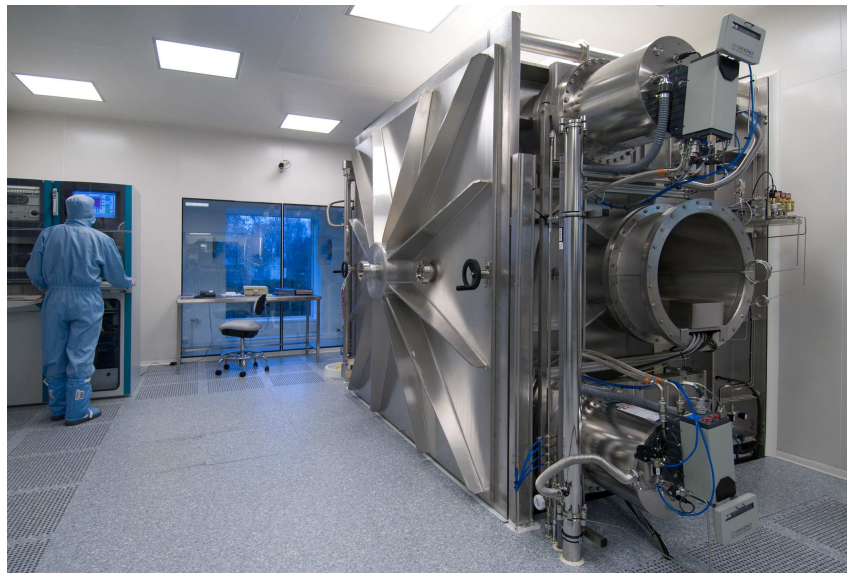
Figure 6.4: The large Ion Beam Sputtering coating machine.
